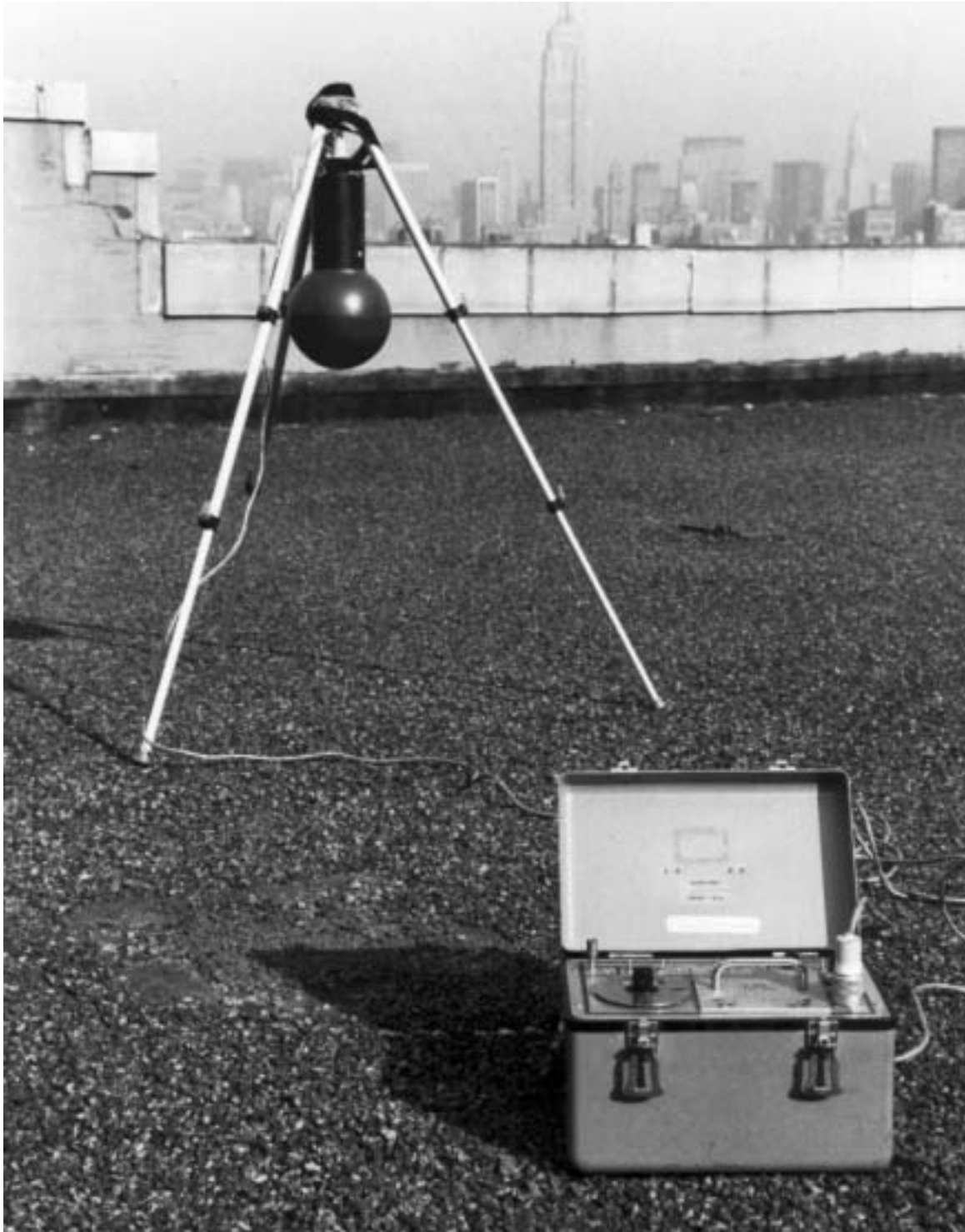
Figure 3.1. SPICER system set up for field measurements showing a tripod mounted ion chamber with an electrometer unit connected via cable to the digital readout box.
