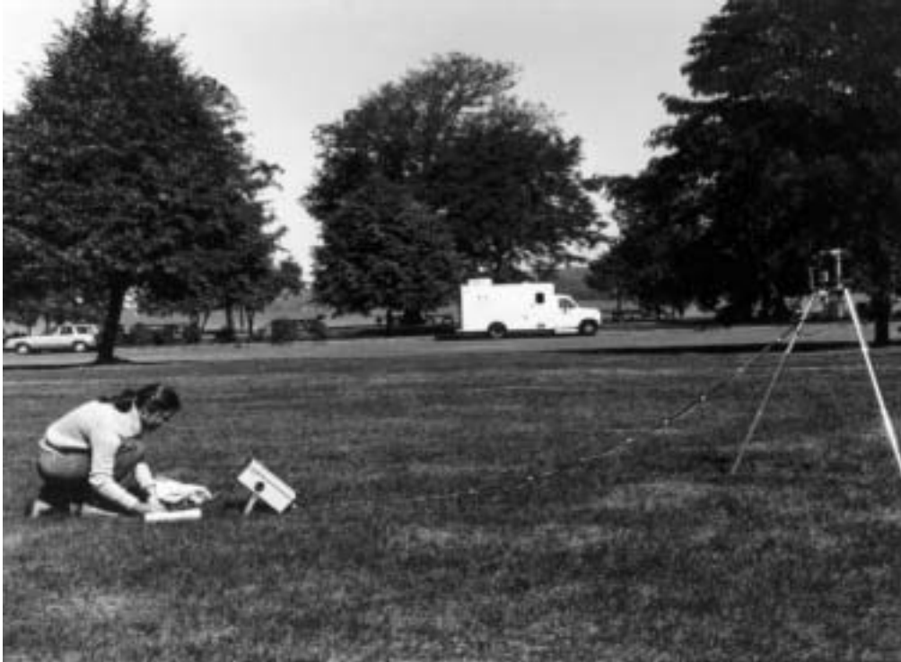
Figure 3.4. Typical field site for conducting in situ \gamma -ray spectrometry showing placement of tripod mounted portable Ge detector and battery-powered multichannel analyzer.
