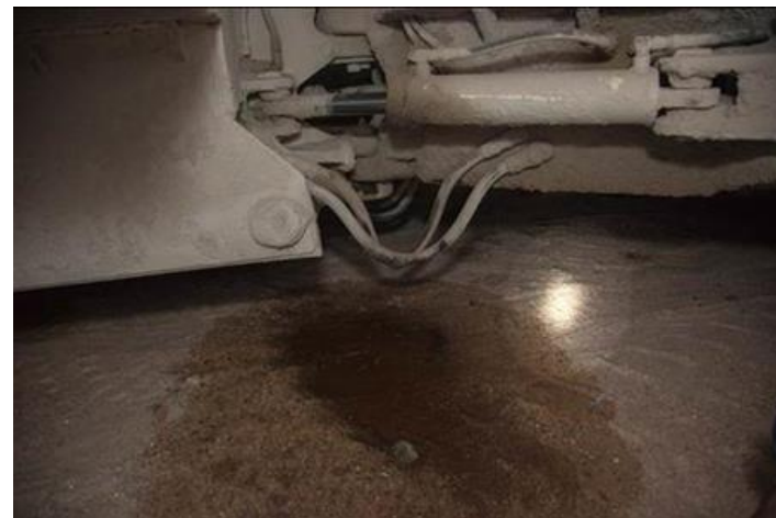
Hydraulic Leak under Sister Vehicle
