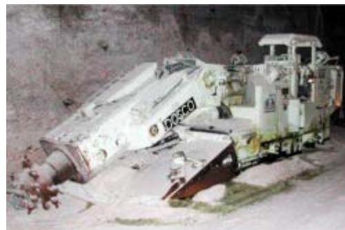
The DOSCO rotary head (road header) mining machine and its pineapple-shaped cutting head underground at WIPP.
