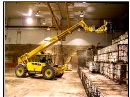
An operator removes a drum from an unburied berm stack.
