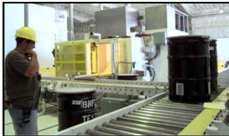
An operator observes test drums as they are transported on a conveyor in the characterization facility at the AMWTP.
