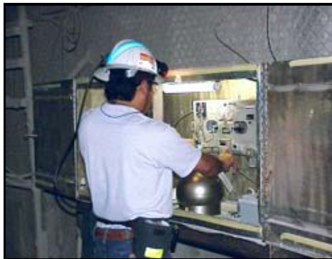
Oscar Garcia, WTS environmental technician, checks canisters used to monitor VOC concentrations.
