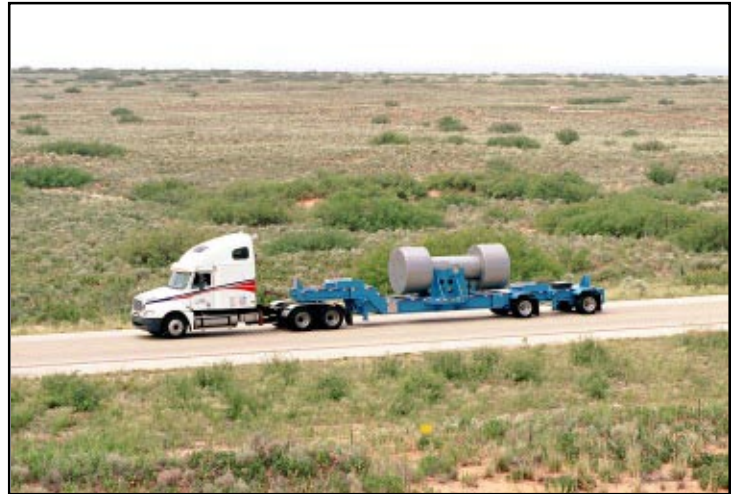
RH72-B shipping casks will be used to transport RH-TRU waste to WIPP.
