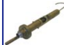
Hanford continuous air monitor (Mid 40s to early 50s)*
