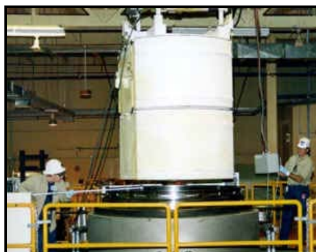
In this file photo: WIPP waste handlers remove CH-TRU waste from this NRC approved TRUPACT-II transportation container. NRC officials will watch a similar operation today.
