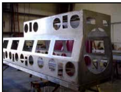
Glovebox under construction at EPD
