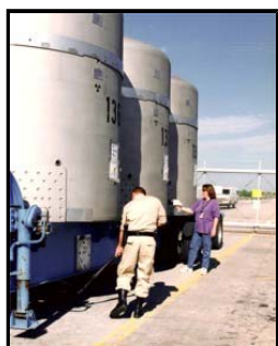
An SFPS employee (left) performs a security check, while a WIPP radcon tech (right) measures for external radiation at the WIPP site gate.
