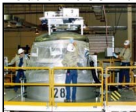
RCT swipes the inside of the ICV lid and the top of the payload.
