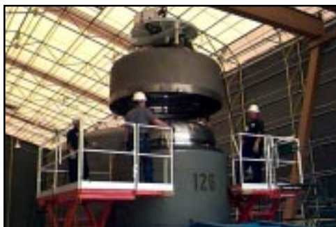
A mobile loading unit is used to close the outer vessel lid on a TRUPACT-II in preparation for shipment.
