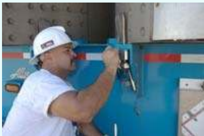
Munoz inspects a tie down that secures the TRUPACT-II to the trailer.
