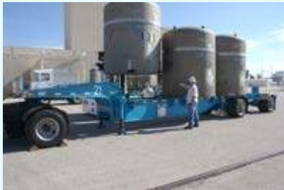
WTS employees Adrian Munoz and Doug Pierce look on as an empty TRUPACT-II is loaded onto a trailer.
