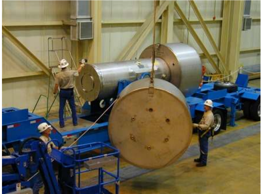
Waste handling technicians remove the impact limiter from an RH 72-B shipping cask during a 2002 performance dry run.
