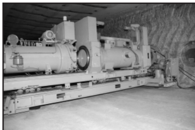
RH-TRU waste is disposed in the walls of the disposal rooms using shielded horizontal emplacement equipment.
