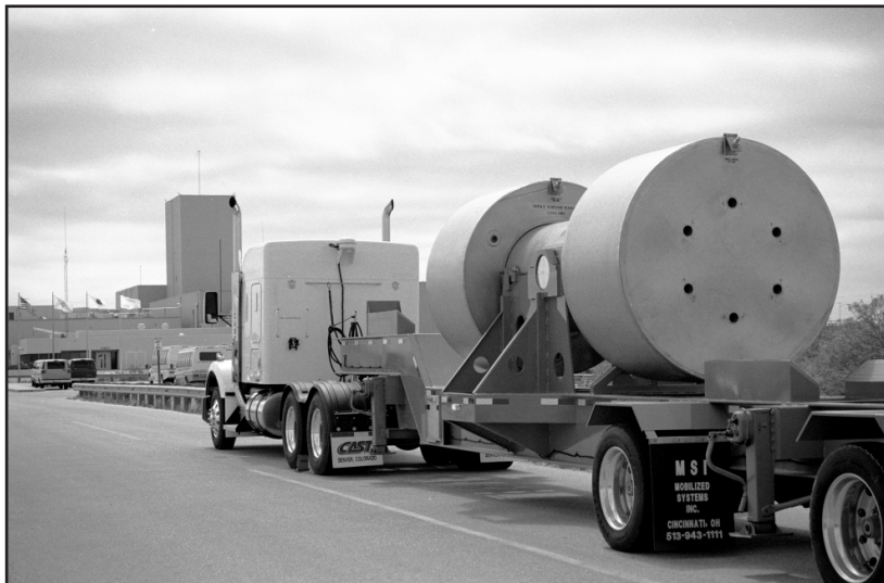
A truck hauling an empty RH-72B cask approaches WIPP. The specially-designed shipping container is shielded by lead and protected by sturdy impact limiters at both ends.
