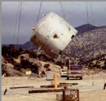
HalfPACT Puncture Test
