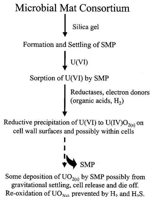
FIGURE 4. Diagram of likely processes that facilitate the removal of dissolved U in the SMP system in the dark.
