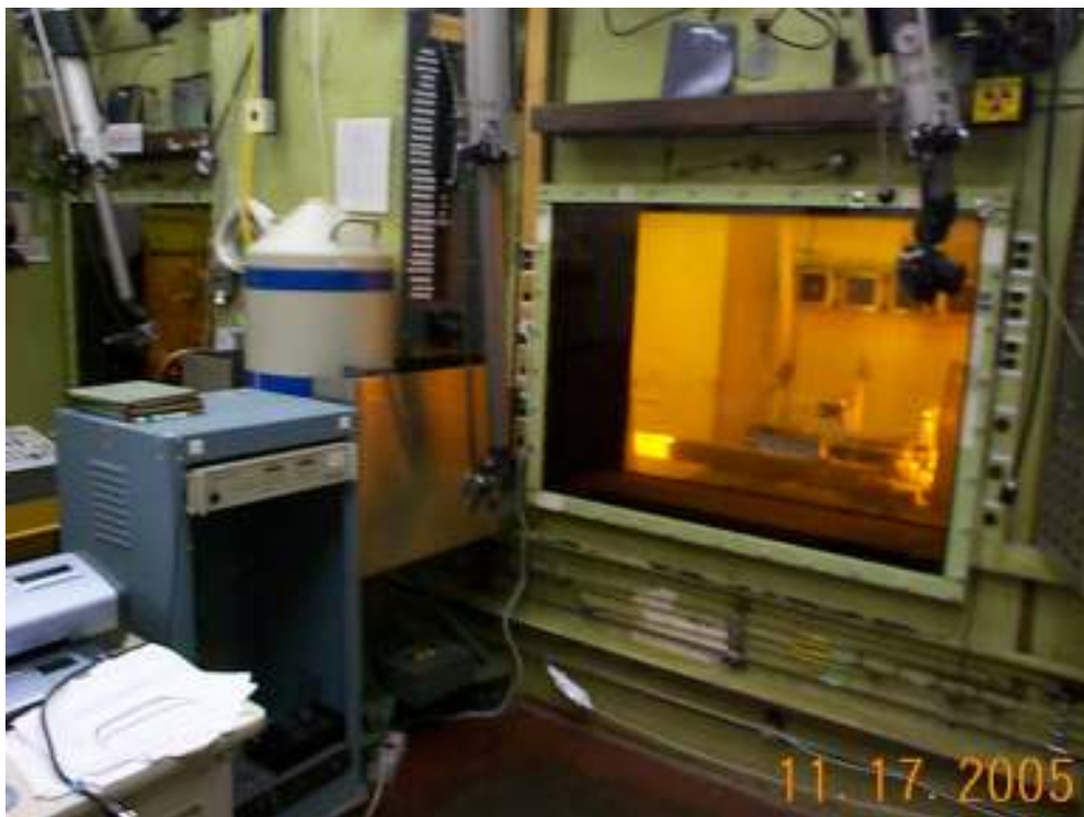
Figure 2. Exterior View of AGHCF Hot Cell
