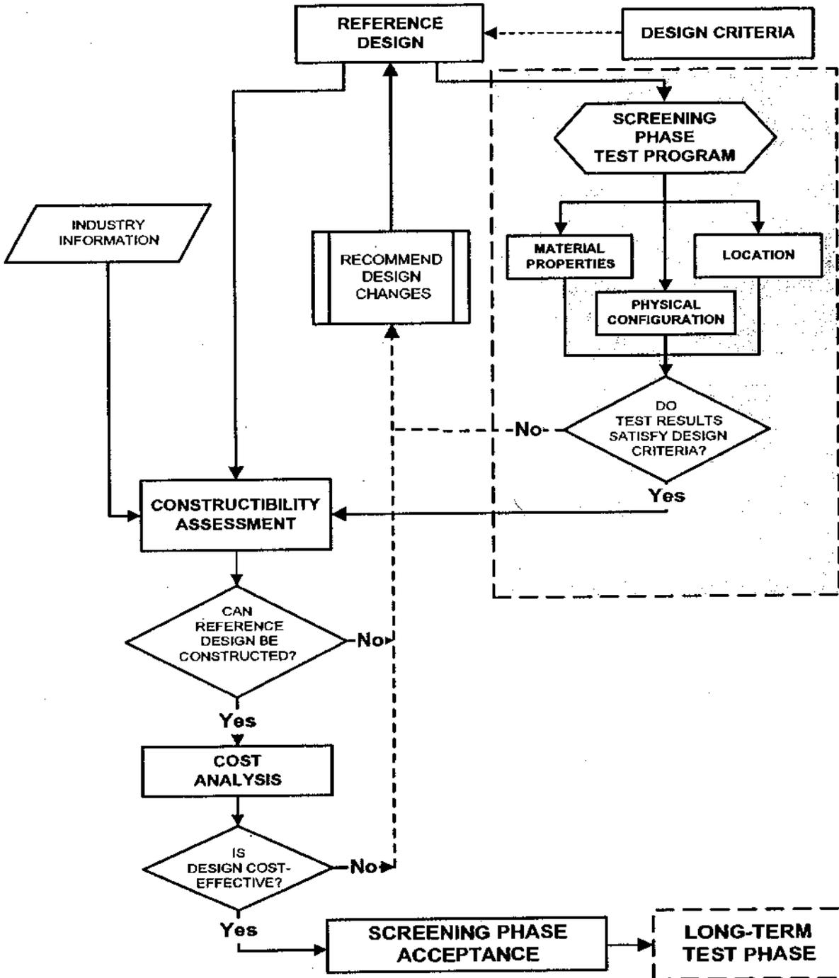
Figure 2. Screening Phase Testing Process
