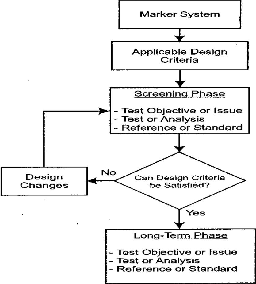
Figure 4. Tests Selection Rationale
