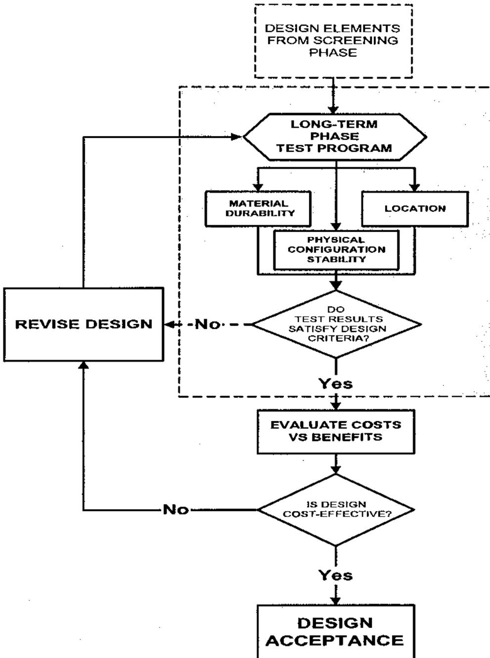
Figure 3. Long-Term Phase Testing Process
