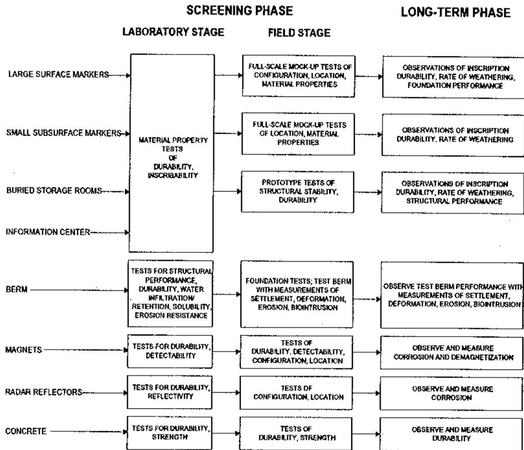
**Figure 5. Permanent Markers Test Program Sequence**
