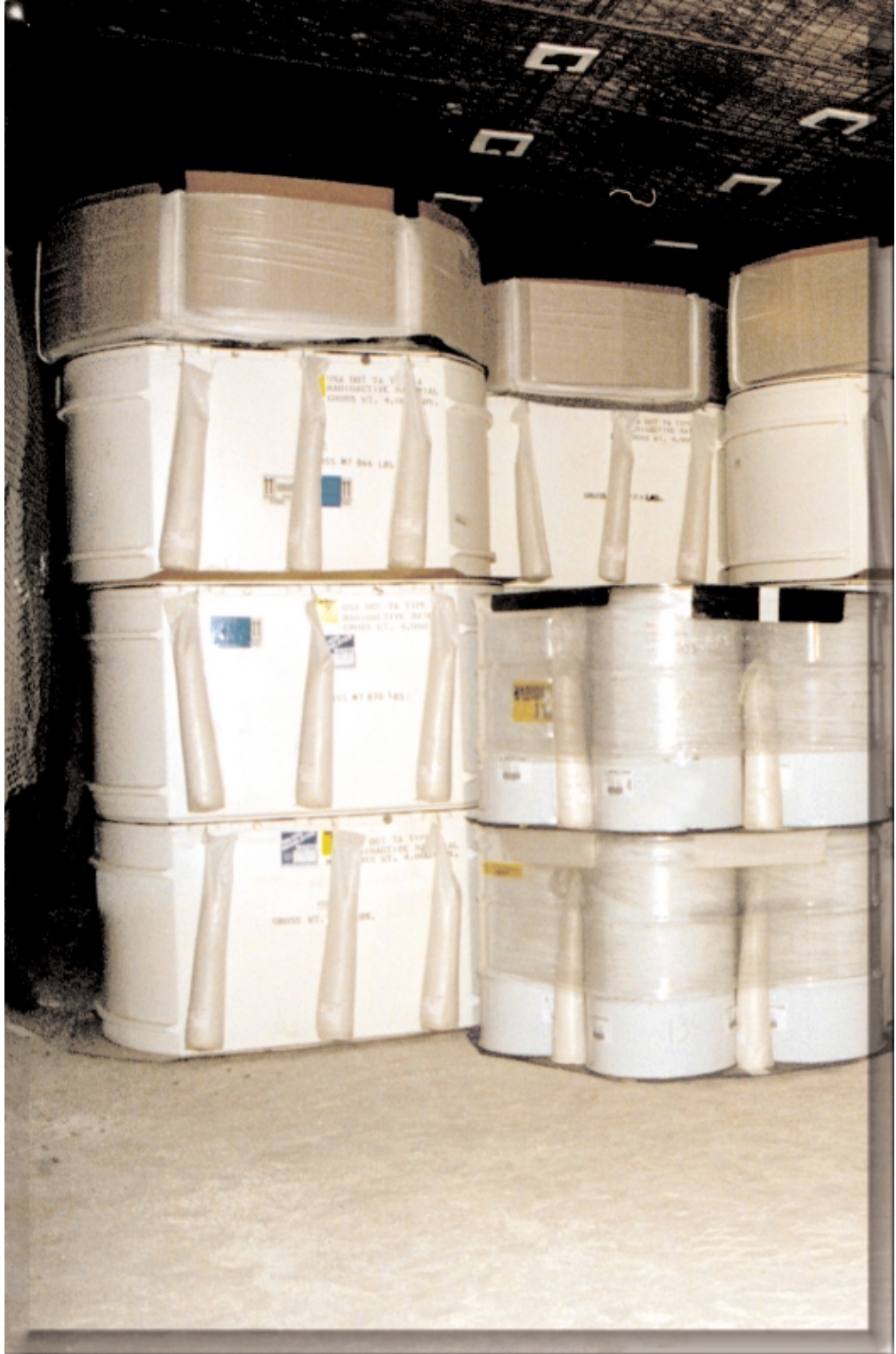
Standard waste boxes and seven packs stacked in Panel 1, Room 7 of the WIPP repository.
