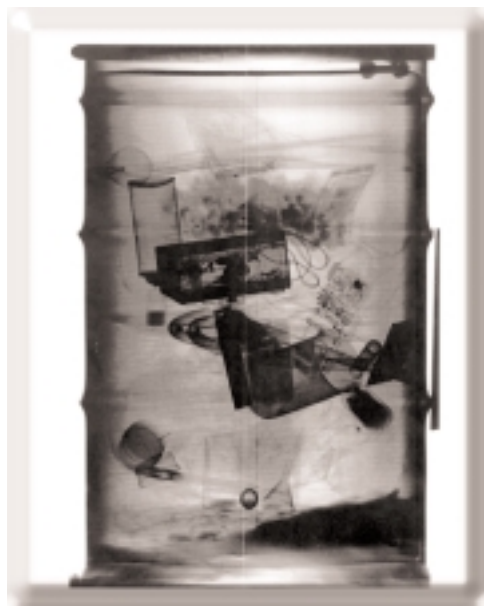
Each transuranic waste site that ships to the WIPP must first characterize (identify and describe) the waste’s physical, chemical, and radiological properties. Real-time radiography is a characterization method that uses x-rays.
