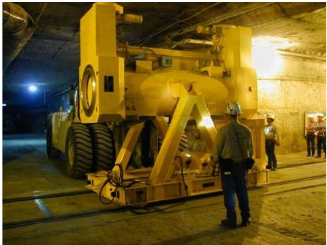
A demonstration of the Horizontal Emplacement and Retrieval Equipment (HERE) that will be used for RH waste disposal.
