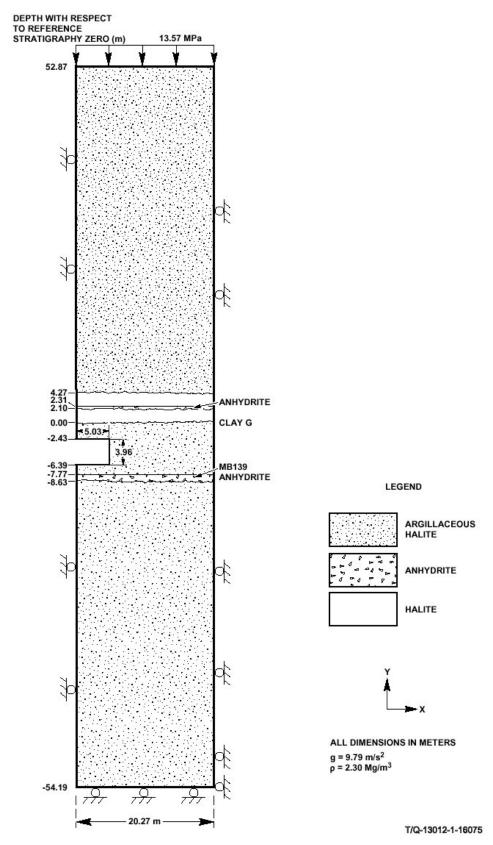
Figure PORSURF-1. Stratigraphy for the Porosity Surface Calculations.
