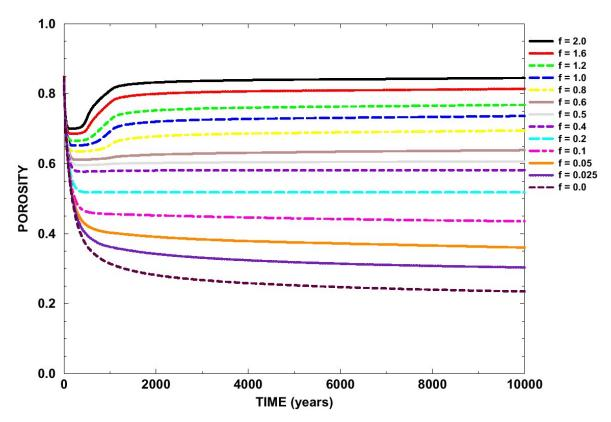
2 Figure PORSURF-3. Disposal Room Porosity for Various Values of the Scale Factor (f).
