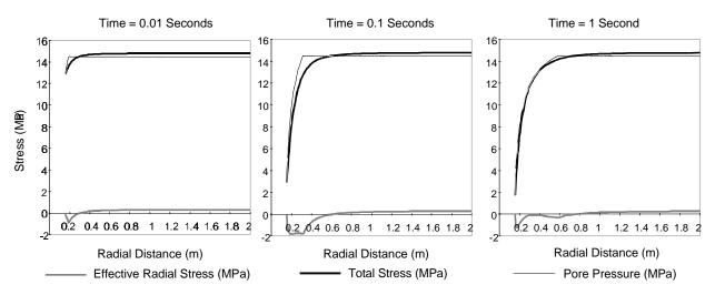
Figure 12. Effective Stress, Total Stress, and Pore Pressure Profiles in the waste at three independent times from the EPA's Analysis of Air Drilling.
