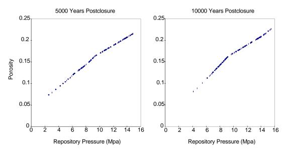
Figure 5. BRAGFLO Porosity Values Versus Pressure Profiles for Undisturbed Scenarios of the CCA.
