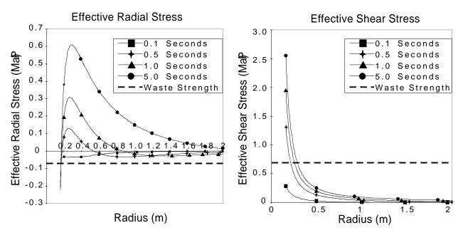
Figure 8. Computed Radial (Normal) And Shear Stresses In A Hemispherical Cavity During Spall From GASOUT, Assuming 14.5 MPa Initial Repository Pressure,  $1.7 \times 10^{-13}$  m<sup>2</sup> Waste Permeability, And No Material Removal From Failure.
