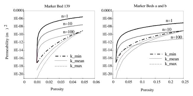
Fig. 21. Permeability vs. Porosity Model With BRAGFLO for Left) Marker Bed 139 and Right) Marker Beds a and b.
