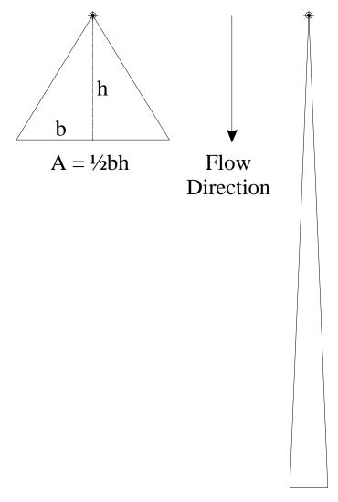
Fig. 22. Conceptual Diagram Of Contaminant Plumes Represented As Simple Triangles, Showing Different Travel Distances For A Relatively Wide Plume Compared To That Of A Relatively Narrow Plume, Where Both Plumes Encompass Equal Volumes Of Fluid And Equal Masses Of Solute.
