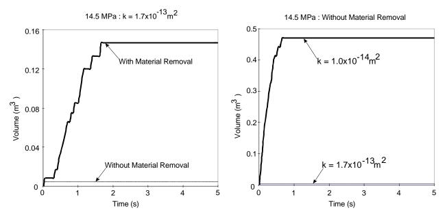
Figure 6. GASOUT Analogy Illustrating The Importance Of Considering Lower Permeabilities. Left) Constant Permeability With And Without Material Removal. Right) Without Material Removal At Two Different Permeabilities.
