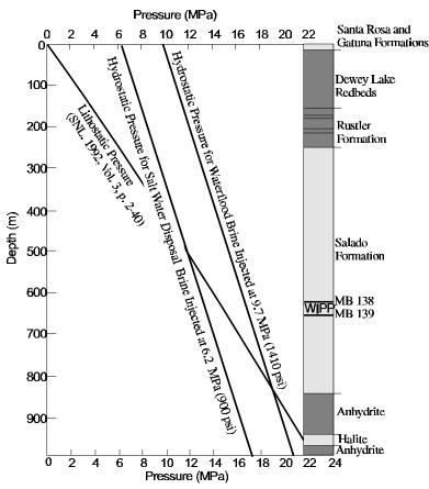
Fig. 19. Comparison of Approved Injection Pressures For Salt Water Disposal Well Versus Oil Field Water Flood Wells Near WIPP.
