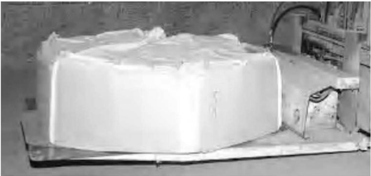
Figure 2.6-43. Push/Pull Attachment Installed on Forklift Tines
