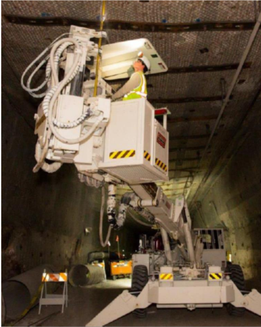
FIGURE 8.—A roof bolting machine at WIPP.
