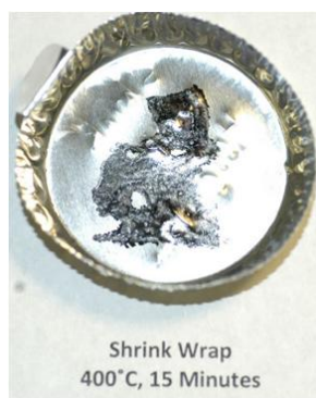
Figure D-33. Images of polymers exposed to elevated temperatures.
