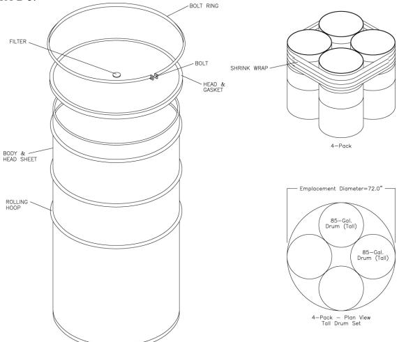
Figure DATA-B-3. 85-gal Drum (Tall) Components and Emplacement Configuration
