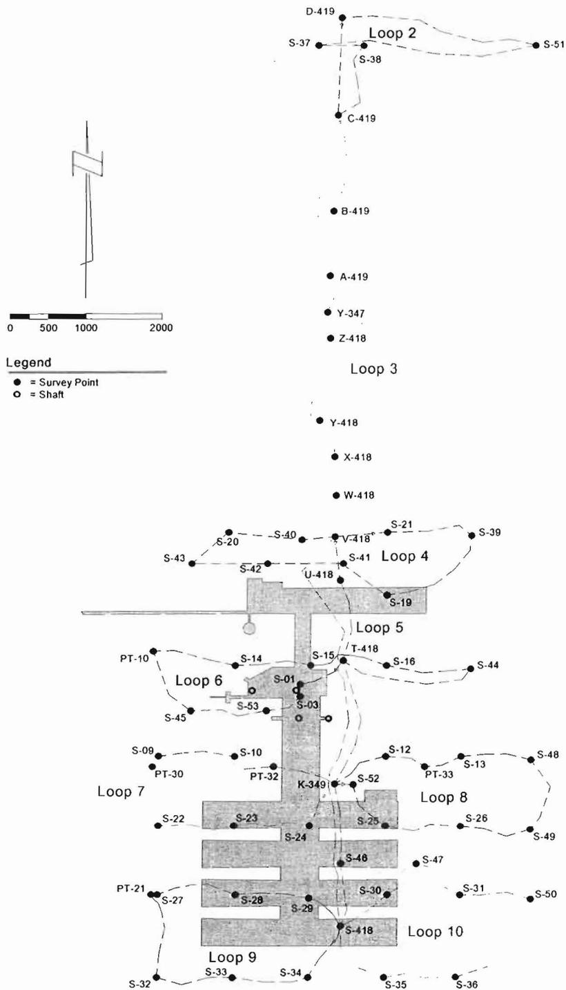
Figure 1. Individual Loops, Total Survey and Underground Excavations
