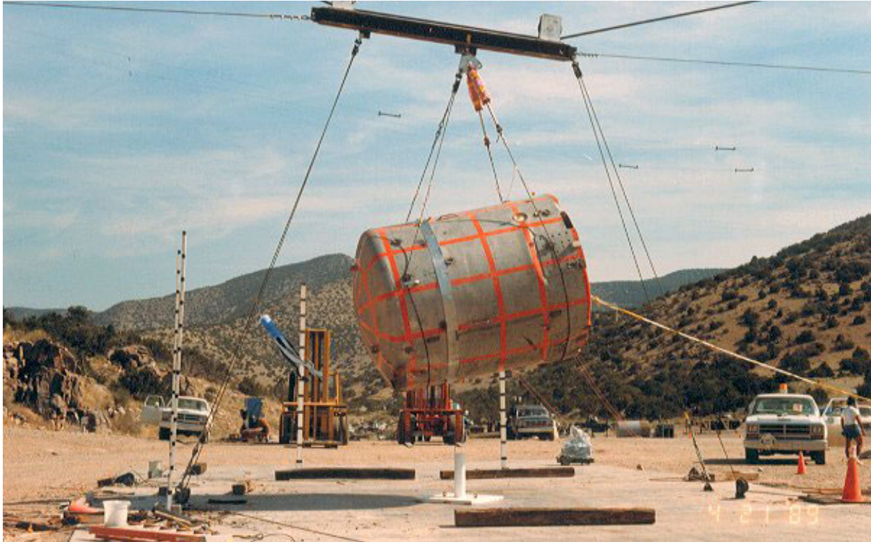
Figure 2.10.3-92 – CTU-3 Puncture Drop No. 7; Pre-Drop Positioning
