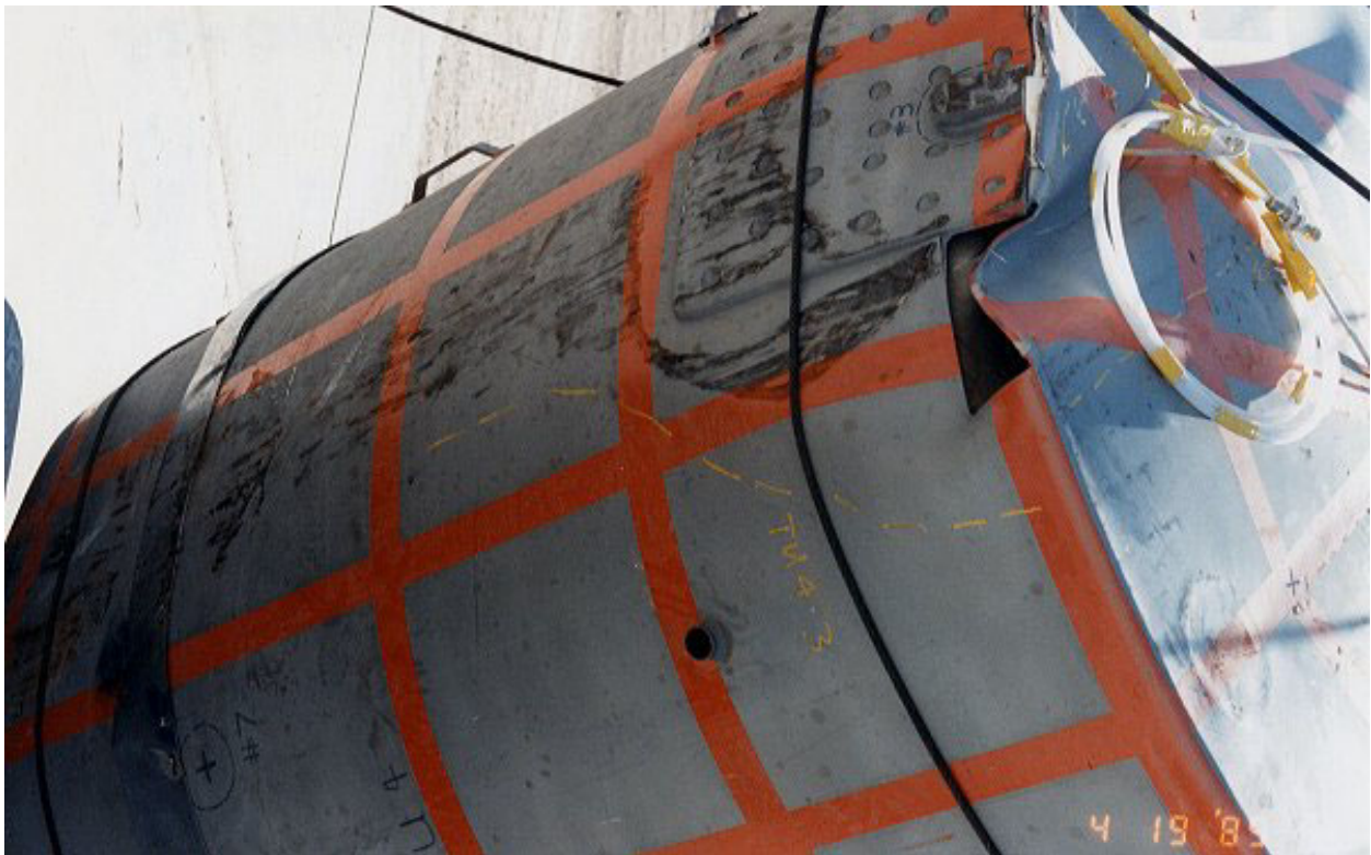
Figure 2.10.3-85 – CTU-3 Free Drop No. 3; Post-Drop Damage
