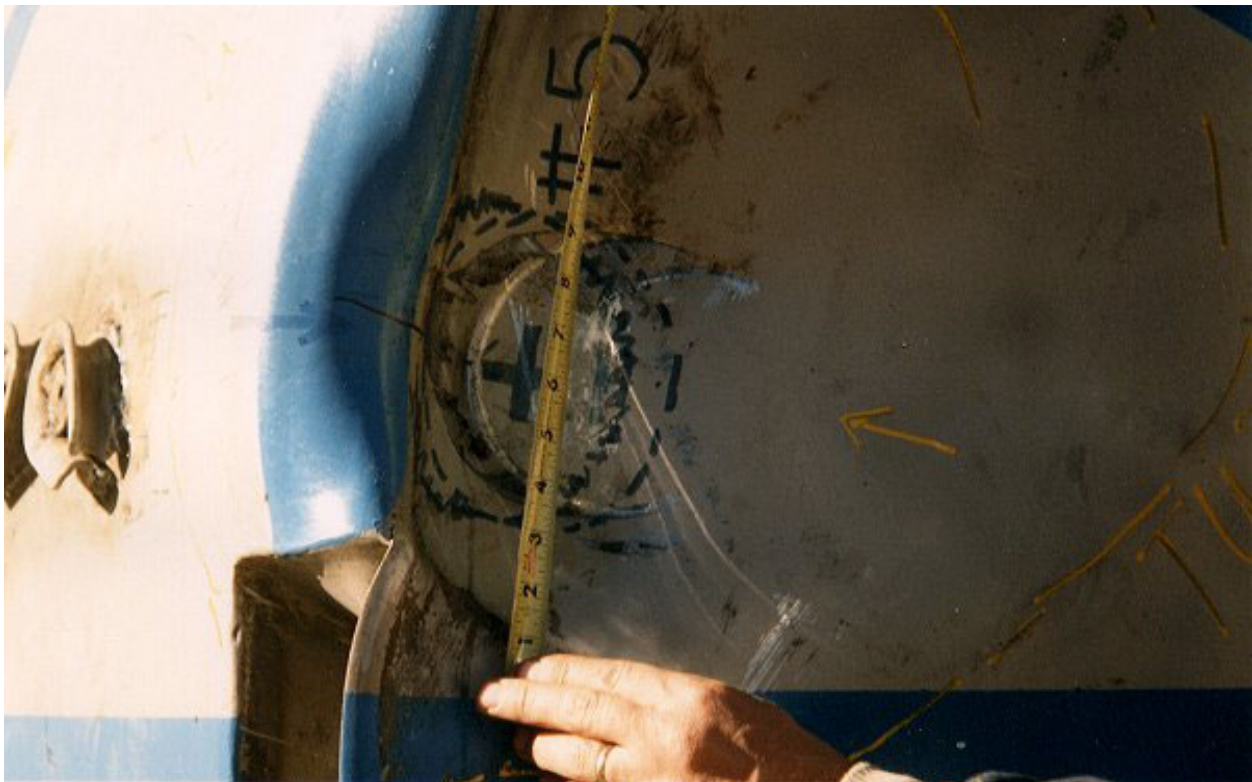
Figure 2.10.3-67 – CTU-2 Puncture Drop 5; Post-Drop Damage
