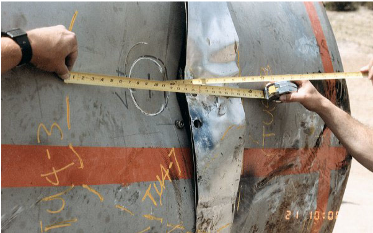
Figure 2.10.3-93 – CTU-3 Puncture Drop 7; Post-Drop Damage
