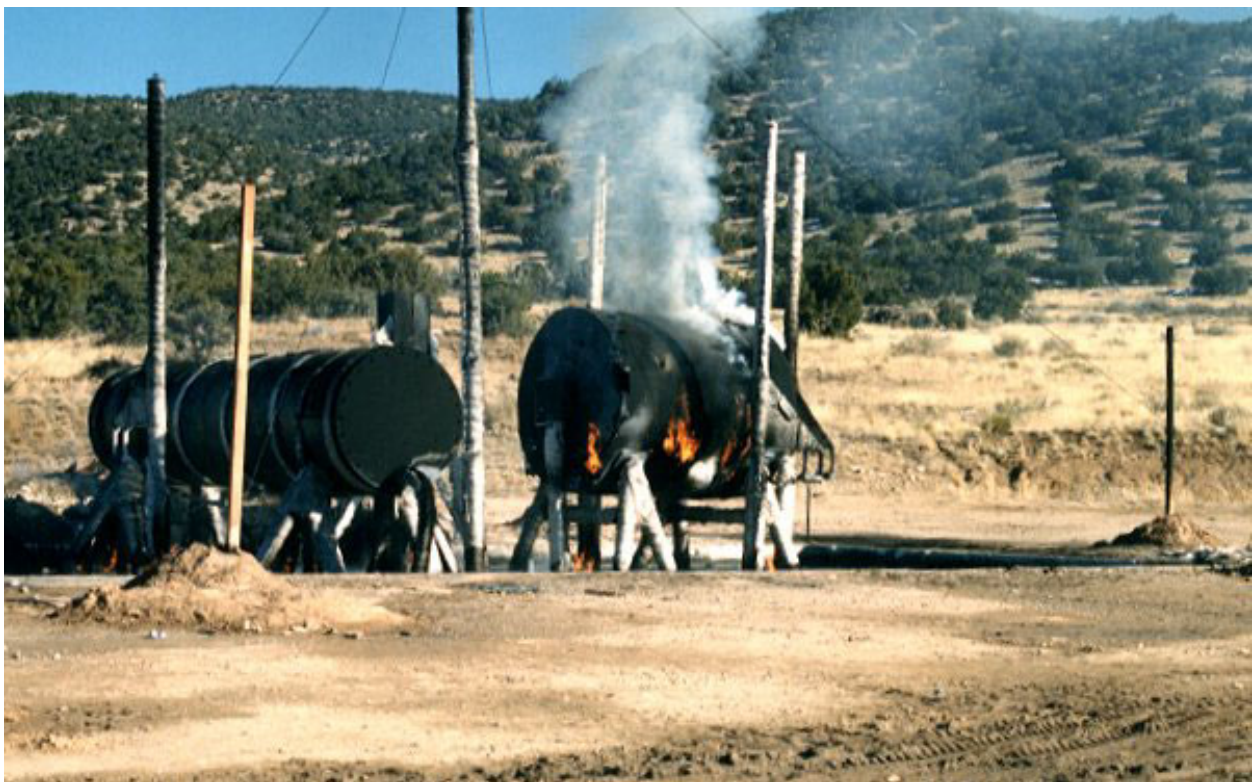
Figure 2.10.3-49 – CTU-1 Fire No. 10; Post-Fire Cool-Down
