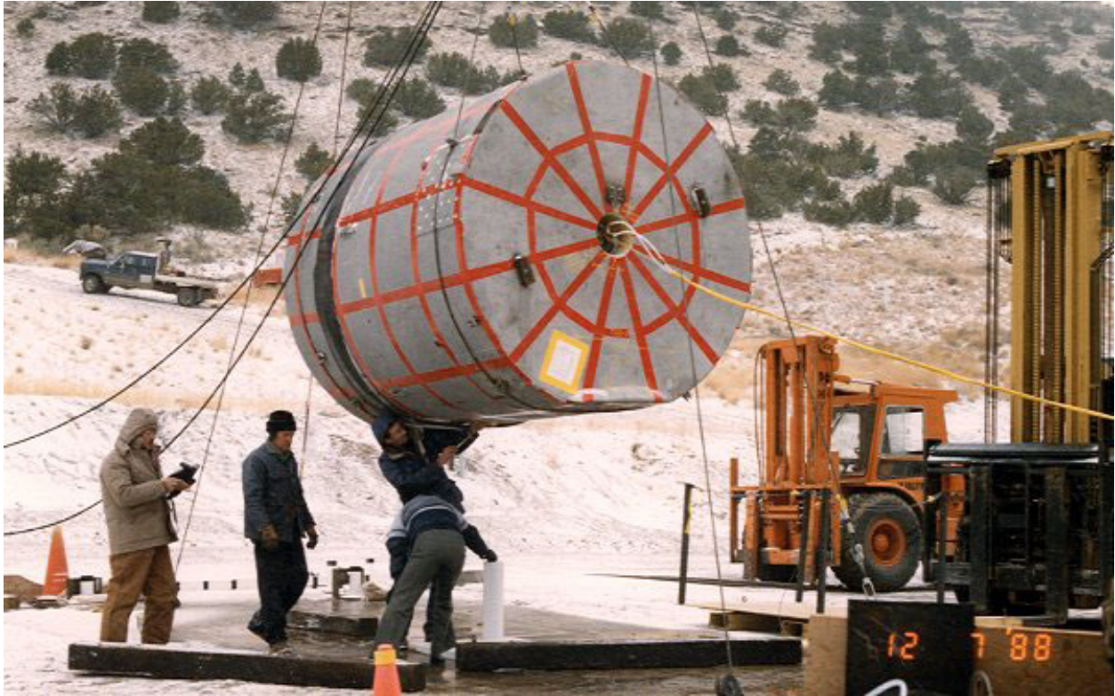
Figure 2.10.3-38 – CTU-1 Puncture Drop No. 6; Pre-Drop Positioning
