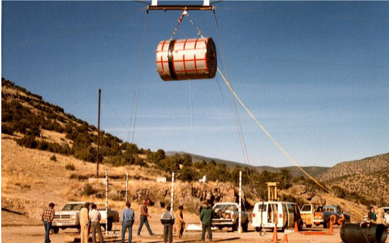
Figure 2.10.3-30 – CTU-1 Free Drop No. 2; Pre-Drop Positioning
