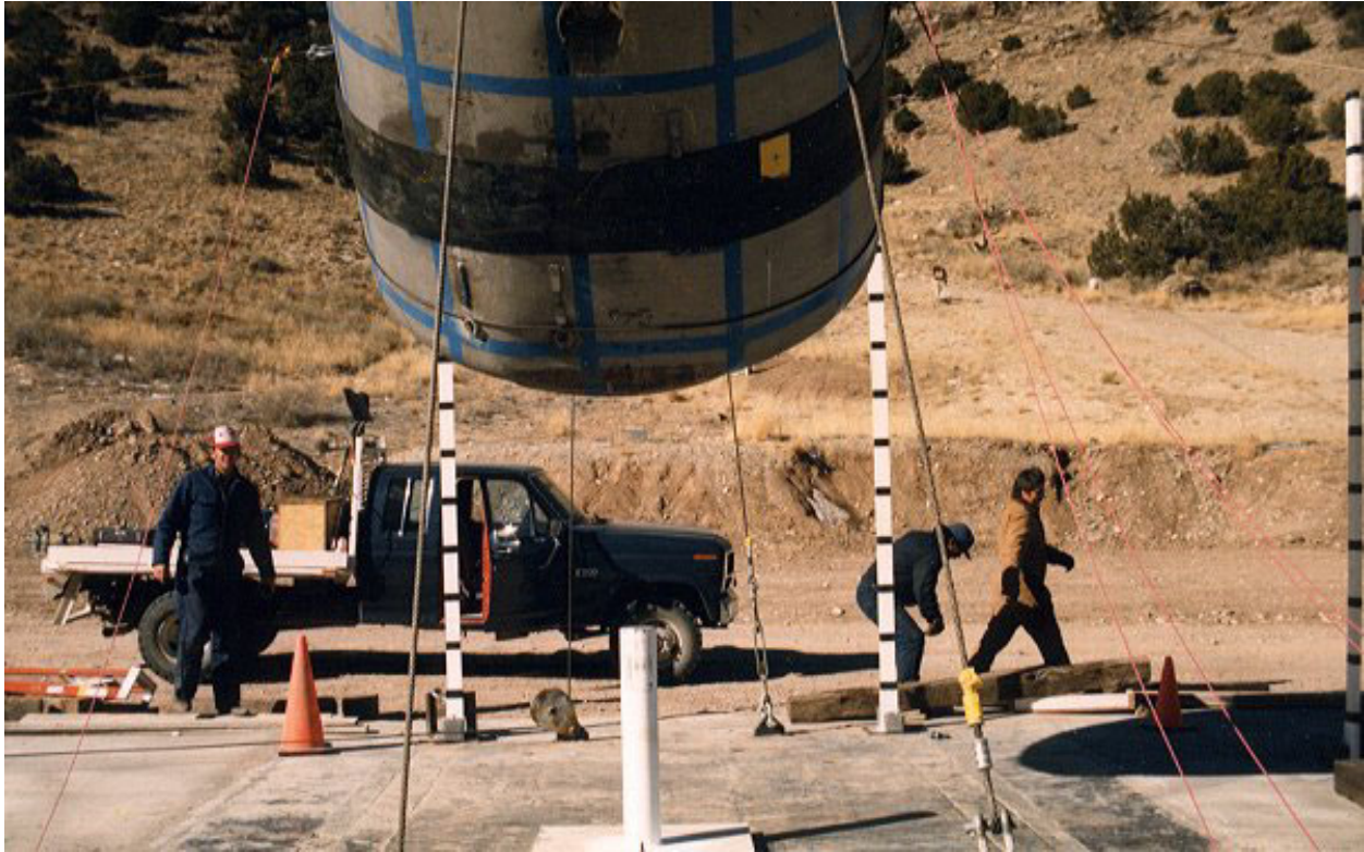
Figure 2.10.3-64 – CTU-2 Puncture Drop No. 4; Pre-Drop Positioning
