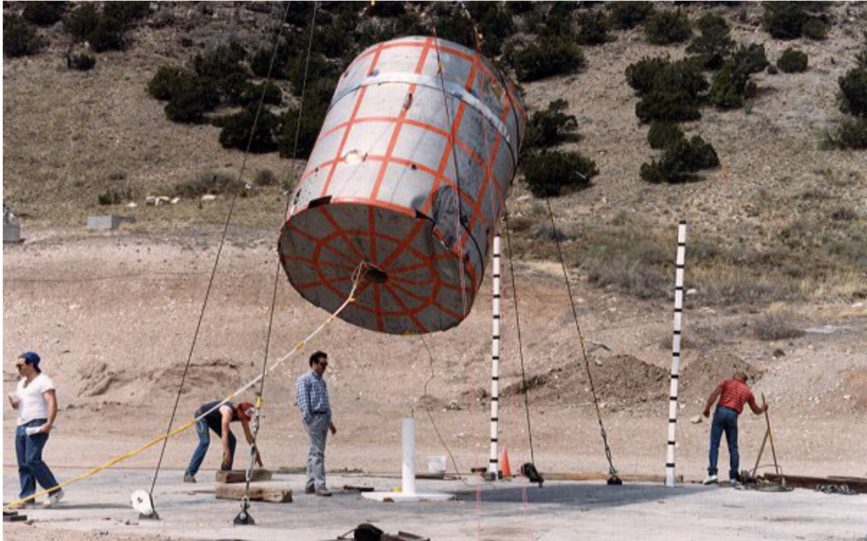
Figure 2.10.3-88 – CTU-3 Puncture Drop No. 5; Pre-Drop Positioning
