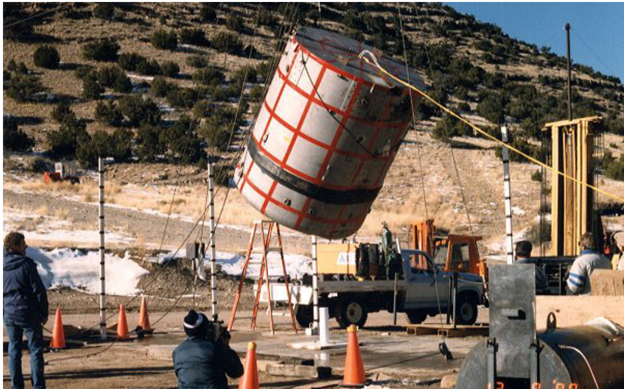
Figure 2.10.3-42 – CTU-1 Puncture Drop No. 8; Pre-Drop Positioning
