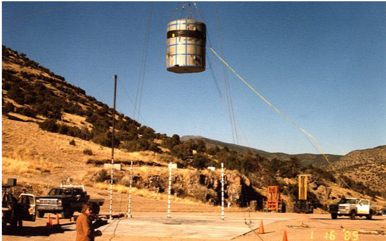
Figure 2.10.3-58 – CTU-2 Free Drop No. 2; Pre-Drop Positioning
