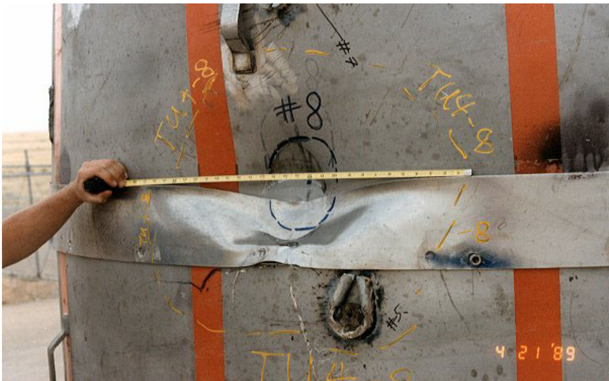
Figure 2.10.3-95 – CTU-3 Puncture Drop 8; Post-Drop Damage
