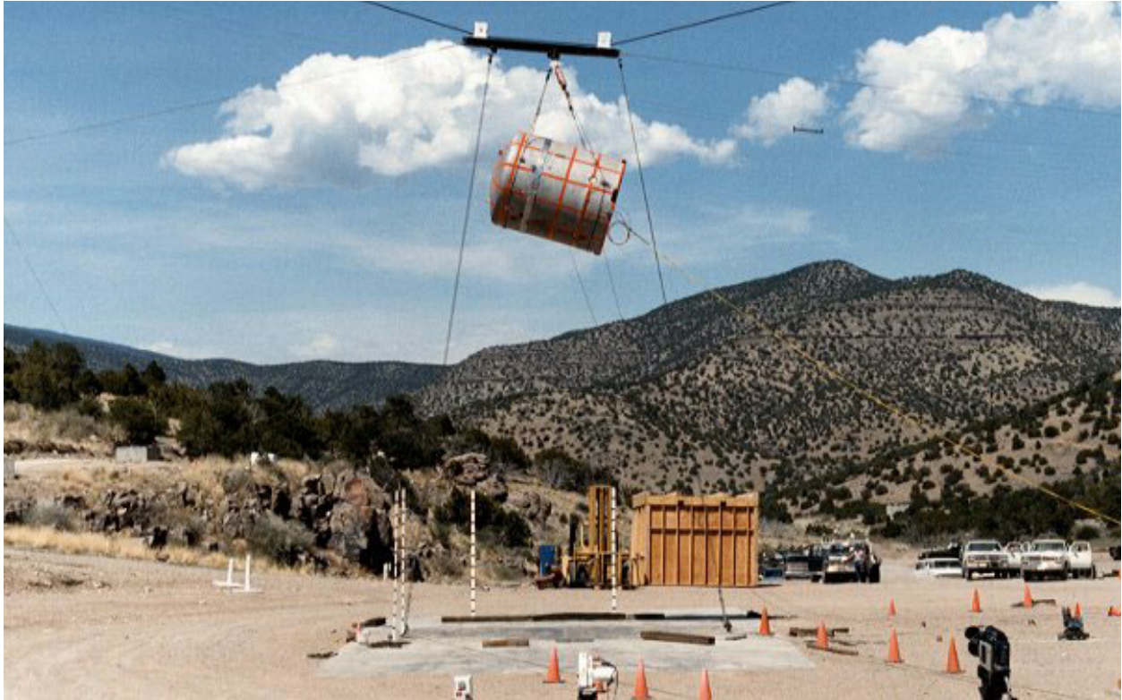
Figure 2.10.3-84 – CTU-3 Free Drop No. 3; Pre-Drop Positioning
