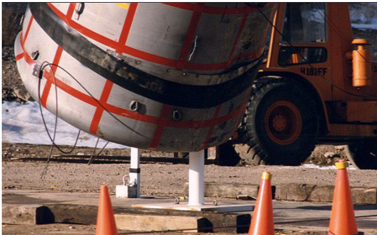
Figure 2.10.3-43 – CTU-1 Puncture Drop No. 8; Moment of Impact
