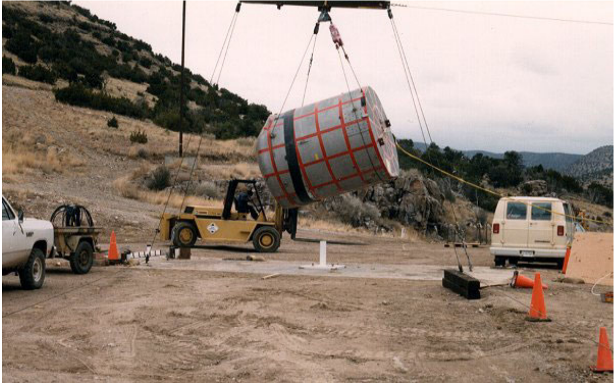
Figure 2.10.3-36 – CTU-1 Puncture Drop No. 5; Pre-Drop Positioning
