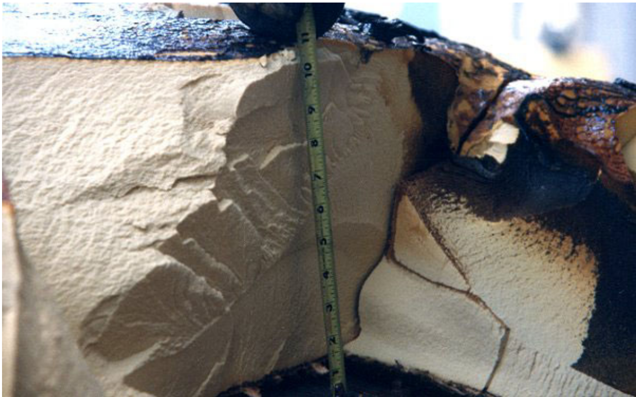
Figure 2.10.3-51 – CTU-1 Disassembly; OCA Lid Unburned Foam Thickness
