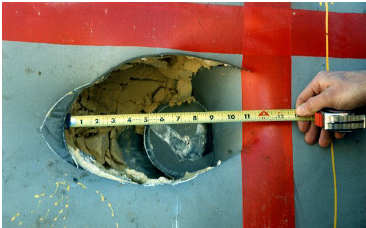
Figure 2.10.3-41 – CTU-1 Puncture Drop No. 7; Post-Drop Damage
