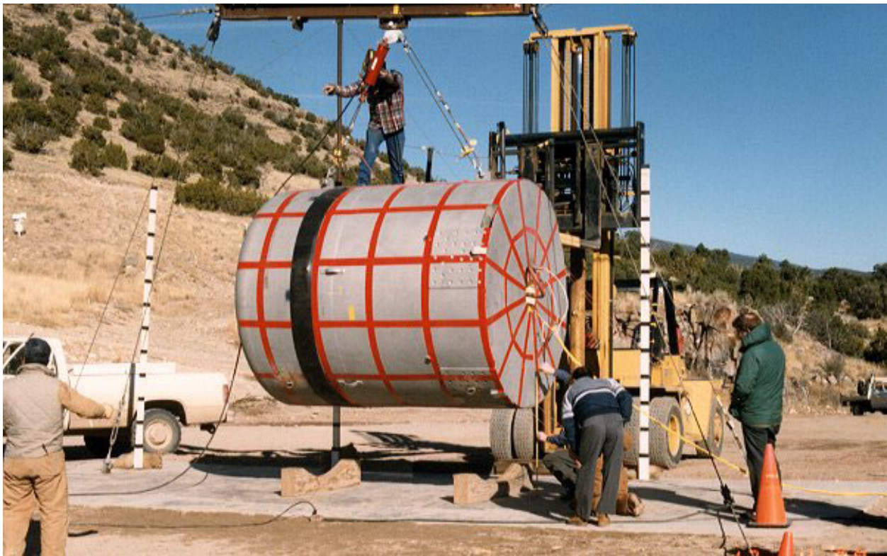
Figure 2.10.3-27 – CTU-1 Free Drop No. 1; Pre-Drop Positioning
