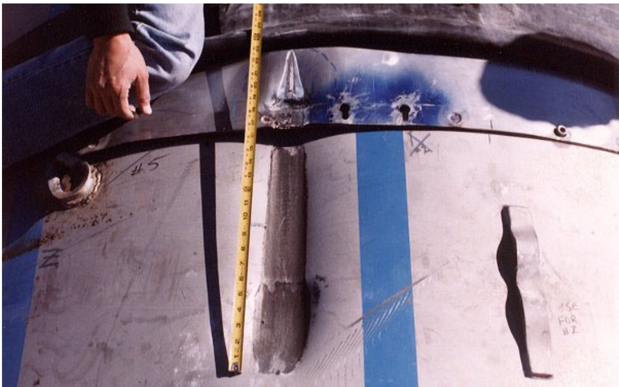
Figure 2.10.3-69 – CTU-2 Puncture Drop 6; Post-Drop Damage
