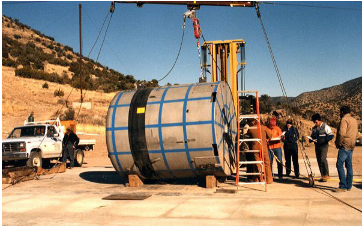
Figure 2.10.3-54 – CTU-2 Free Drop No. 1; Initial Preparation for Testing
