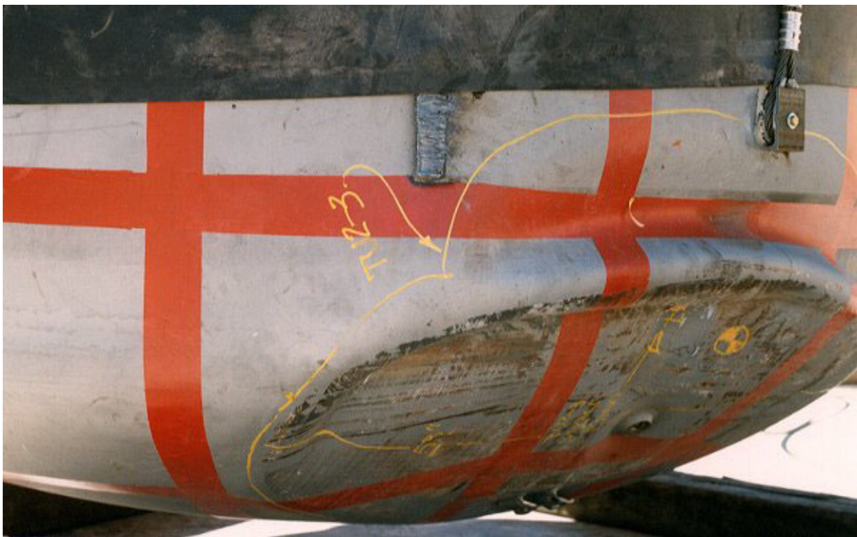
Figure 2.10.3-33 – CTU-1 Free Drop No. 3; Post-Drop Damage
