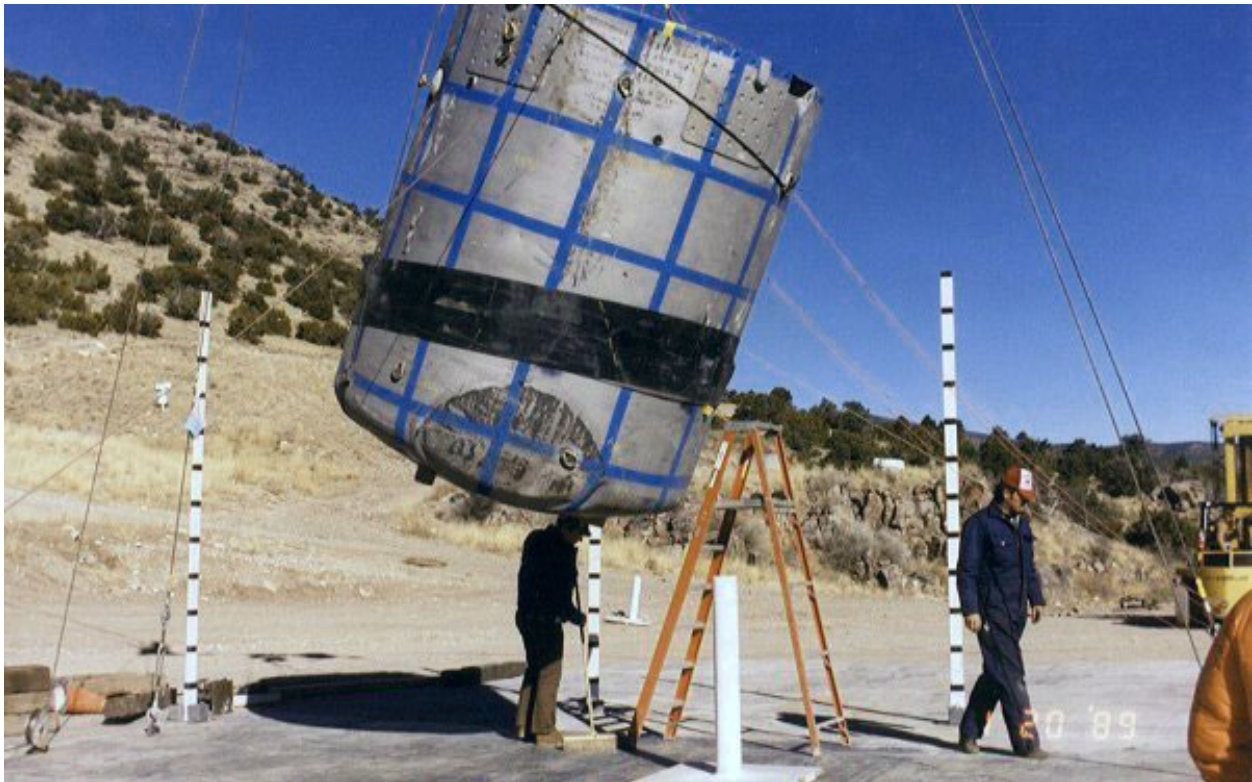
Figure 2.10.3-68 – CTU-2 Puncture Drop No. 6; Pre-Drop Positioning
