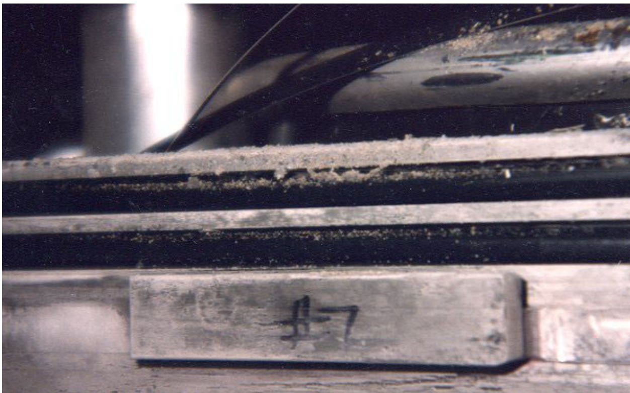
Figure 2.10.3-79 – CTU-2 Disassembly; Debris Contaminating the ICV Main O-ring Seals
