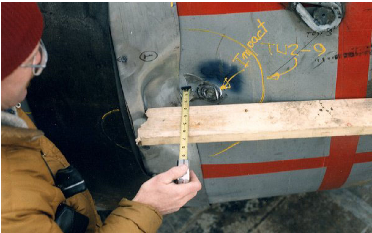
Figure 2.10.3-45 – CTU-1 Puncture Drop No. 9; Post-Drop Damage
