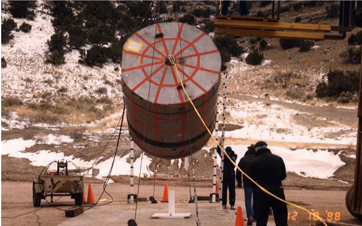
Figure 2.10.3-44 – CTU-1 Puncture Drop No. 9; Pre-Drop Positioning
