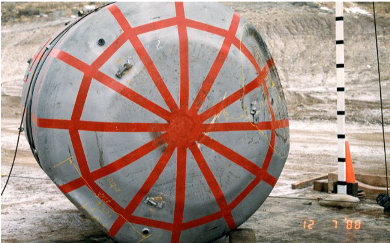
Figure 2.10.3-35 – CTU-1 Free Drop No. 4; Post-Drop Damage
