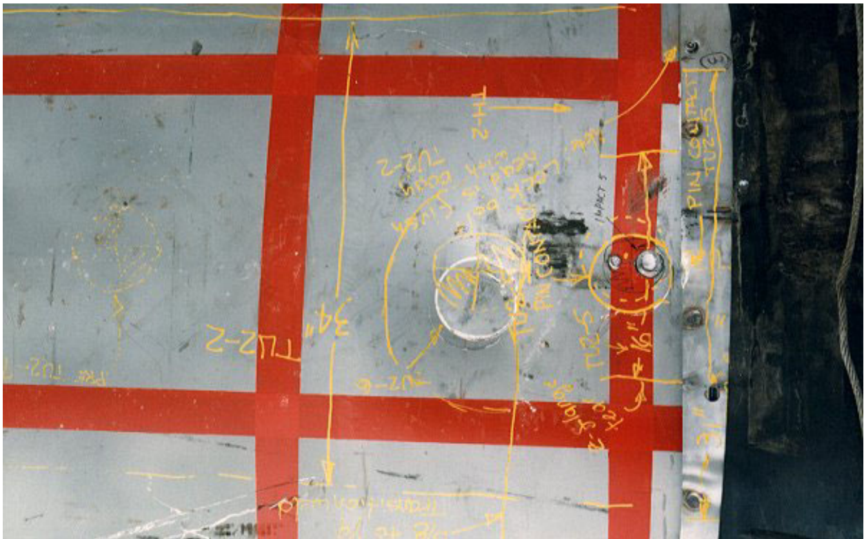
Figure 2.10.3-39 – CTU-1 Puncture Drop No. 6; Post-Drop Damage
