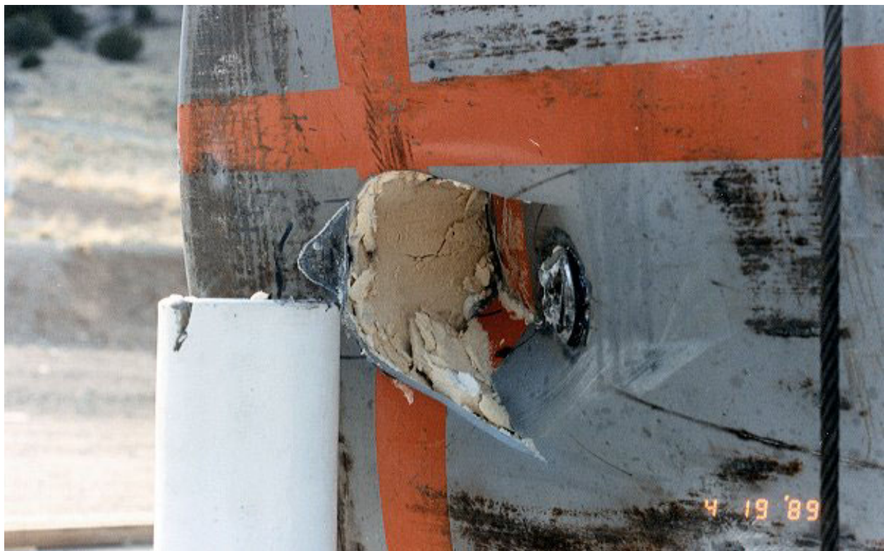
Figure 2.10.3-87 – CTU-3 Puncture Drop 4; Post-Drop Damage
