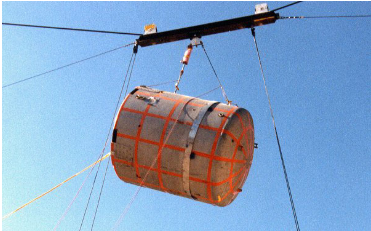
Figure 2.10.3-80 – CTU-3 Free Drop No. 1; Pre-Drop Positioning
