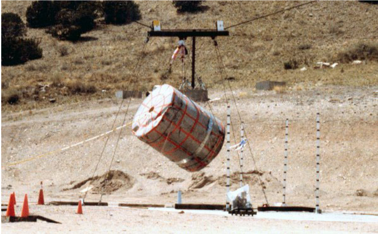
Figure 2.10.3-94 – CTU-3 Puncture Drop No. 8; Pre-Drop Positioning
