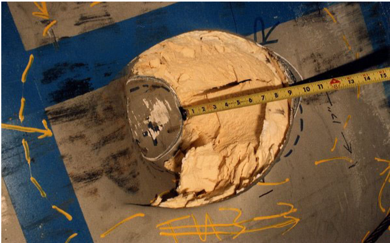
Figure 2.10.3-63 – CTU-2 Puncture Drop R; Post-Drop Damage
