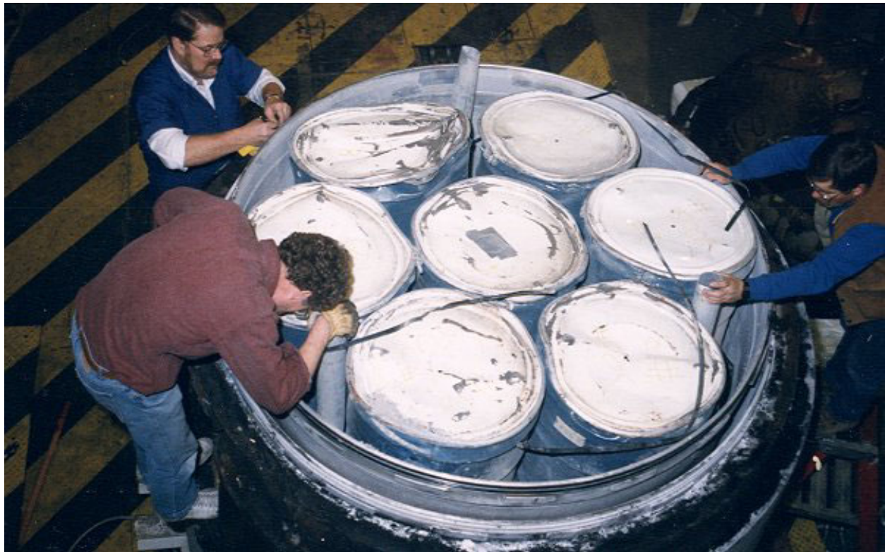
Figure 2.10.3-52 – CTU-1 Disassembly; Payload Drum Removal
