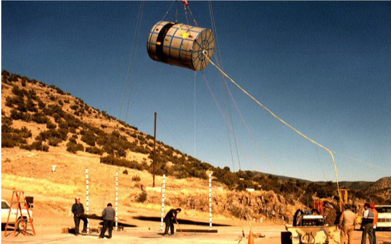
Figure 2.10.3-60 – CTU-2 Free Drop No. 3; Pre-Drop Positioning
