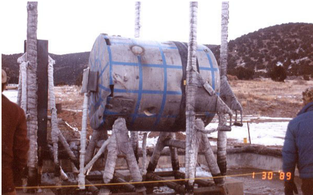
Figure 2.10.3-74 – CTU-2 Fire No. 9; Pre-Fire Positioning
