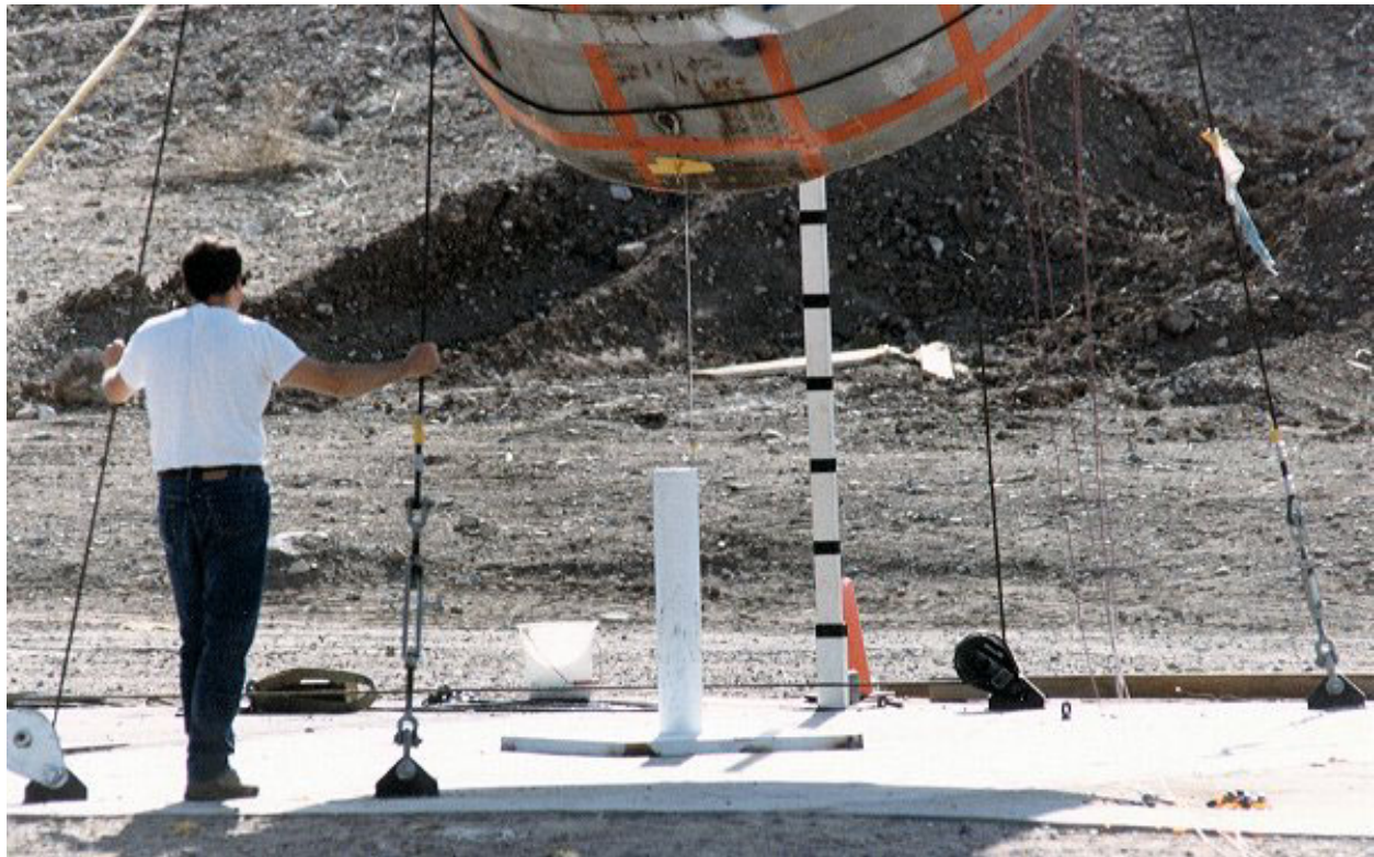
Figure 2.10.3-86 – CTU-3 Puncture Drop No. 4; Pre-Drop Positioning
