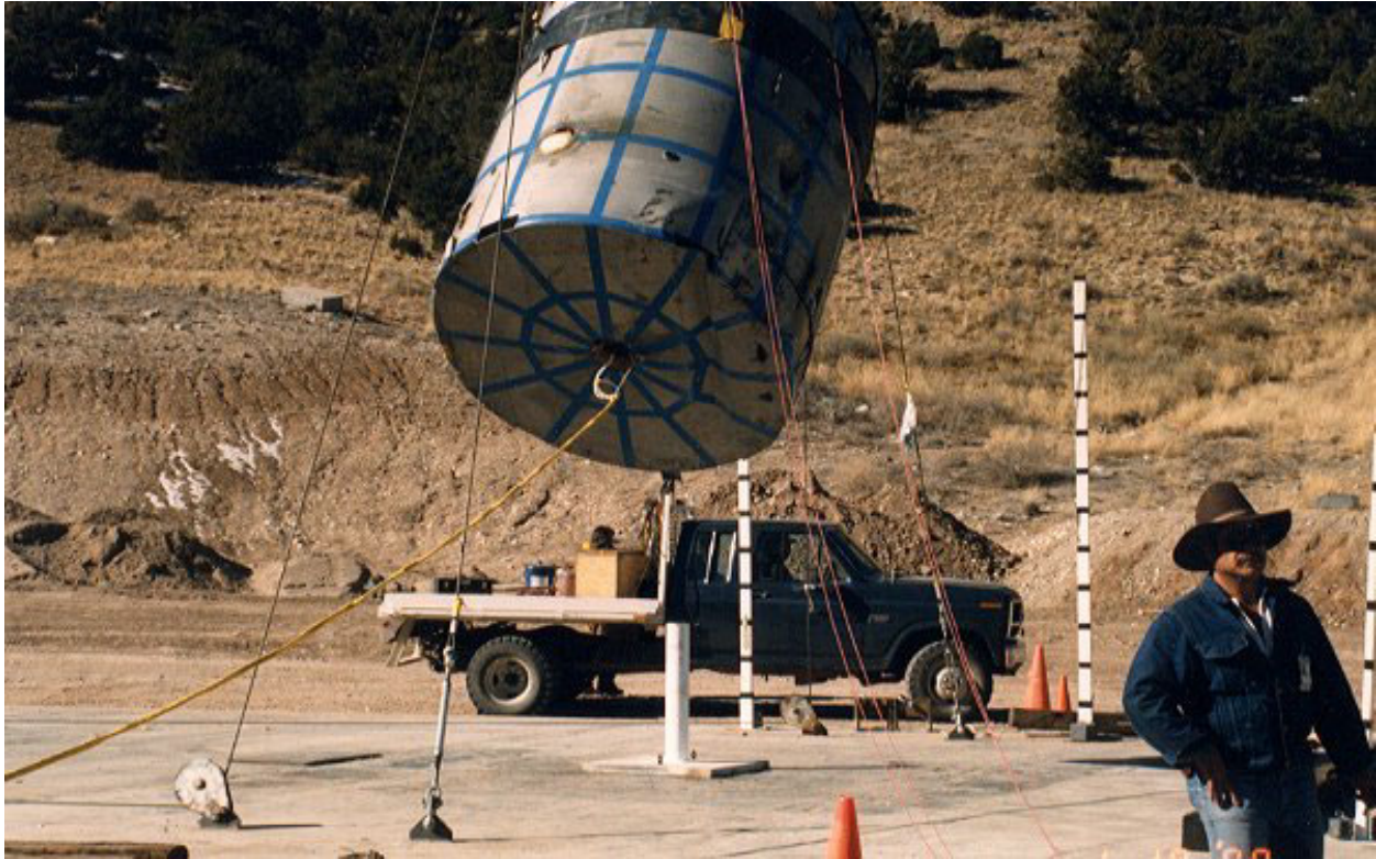
Figure 2.10.3-66 – CTU-2 Puncture Drop No. 5; Pre-Drop Positioning
