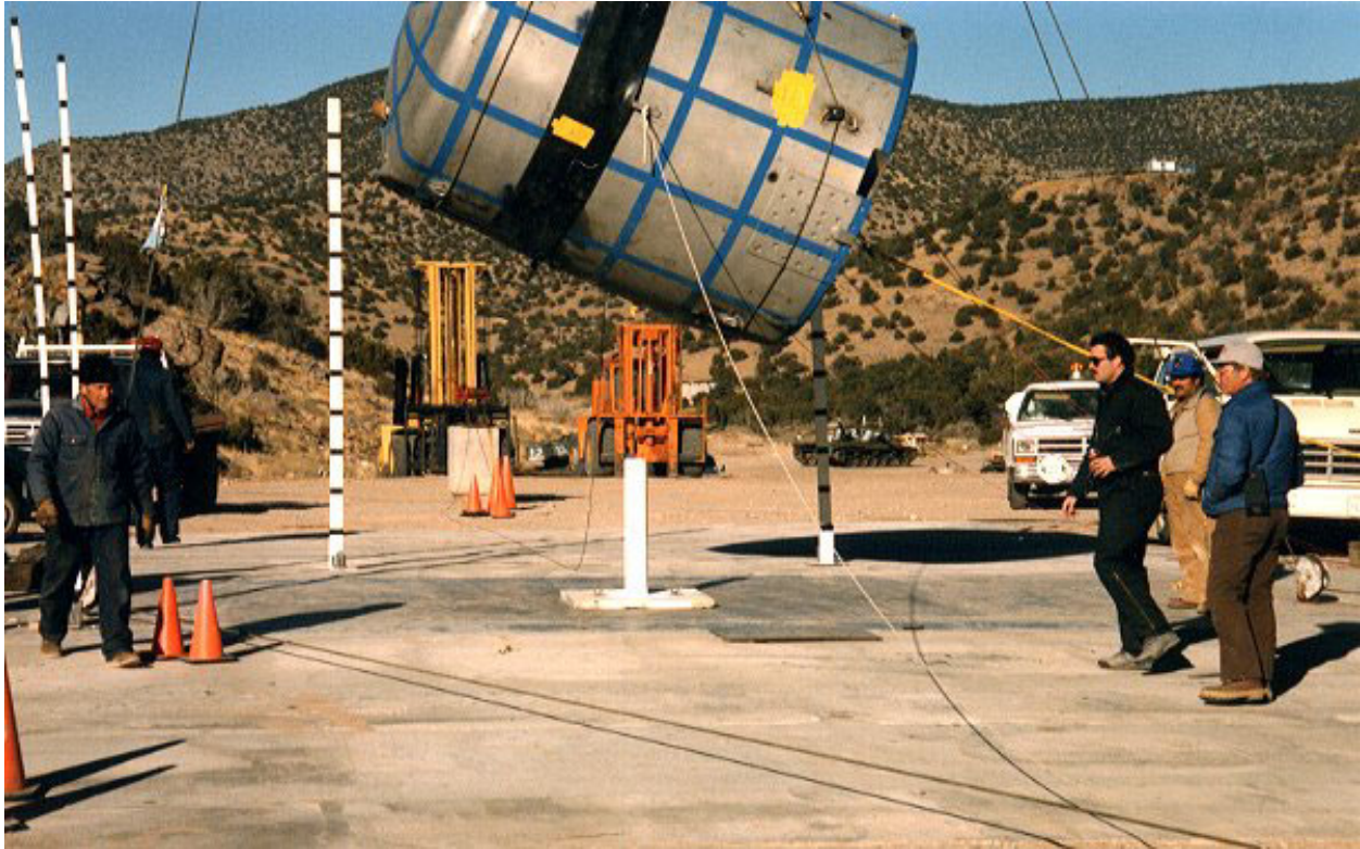
Figure 2.10.3-62 – CTU-2 Puncture Drop No. R; Pre-Drop Positioning
