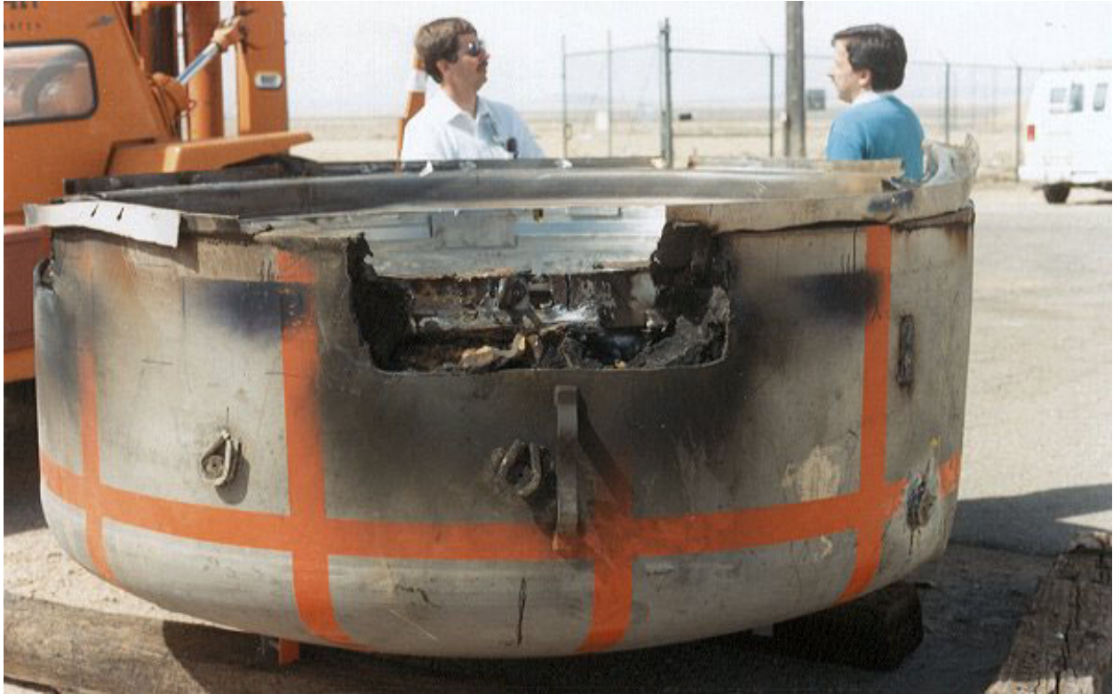
Figure 2.10.3-96 – CTU-3 Disassembly; OCA Lid
