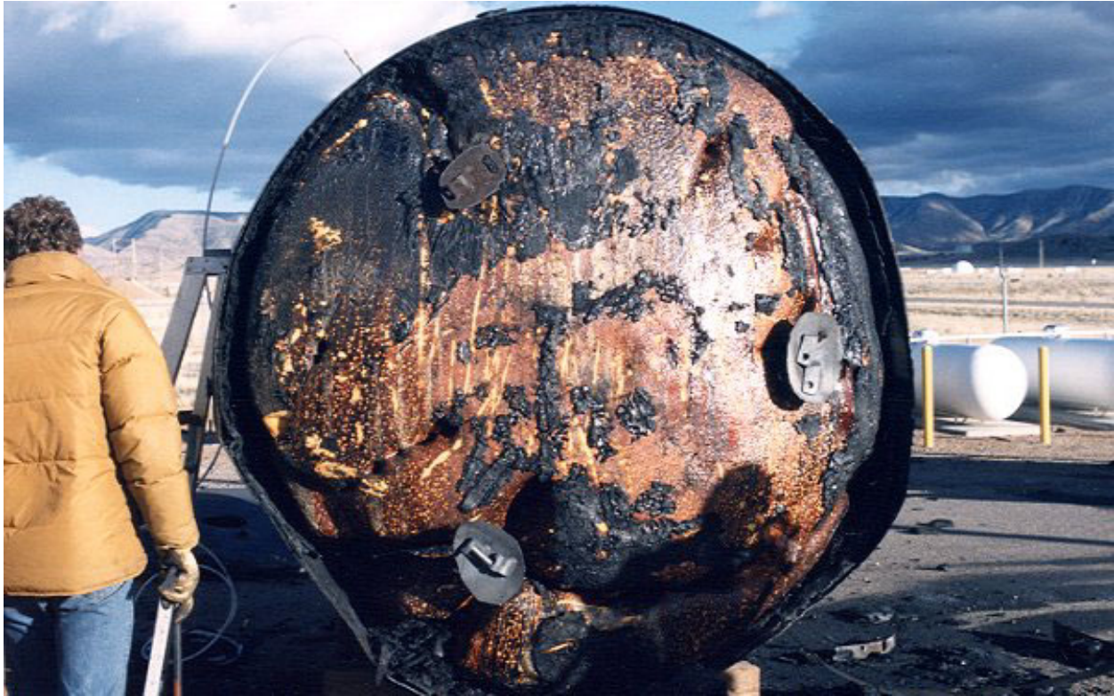
Figure 2.10.3-50 – CTU-1 Disassembly; OCA Lid Unburned Foam
