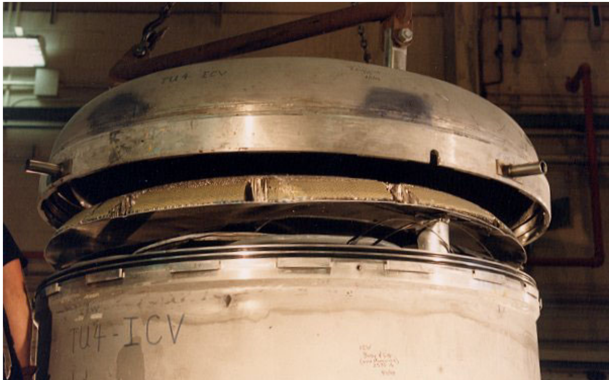
Figure 2.10.3-98 – CTU-3 Disassembly; ICV Lid Removal
