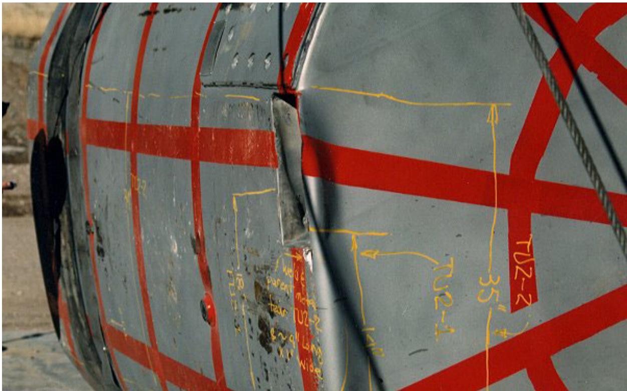
Figure 2.10.3-31 – CTU-1 Free Drop No. 2; Post-Drop Damage
