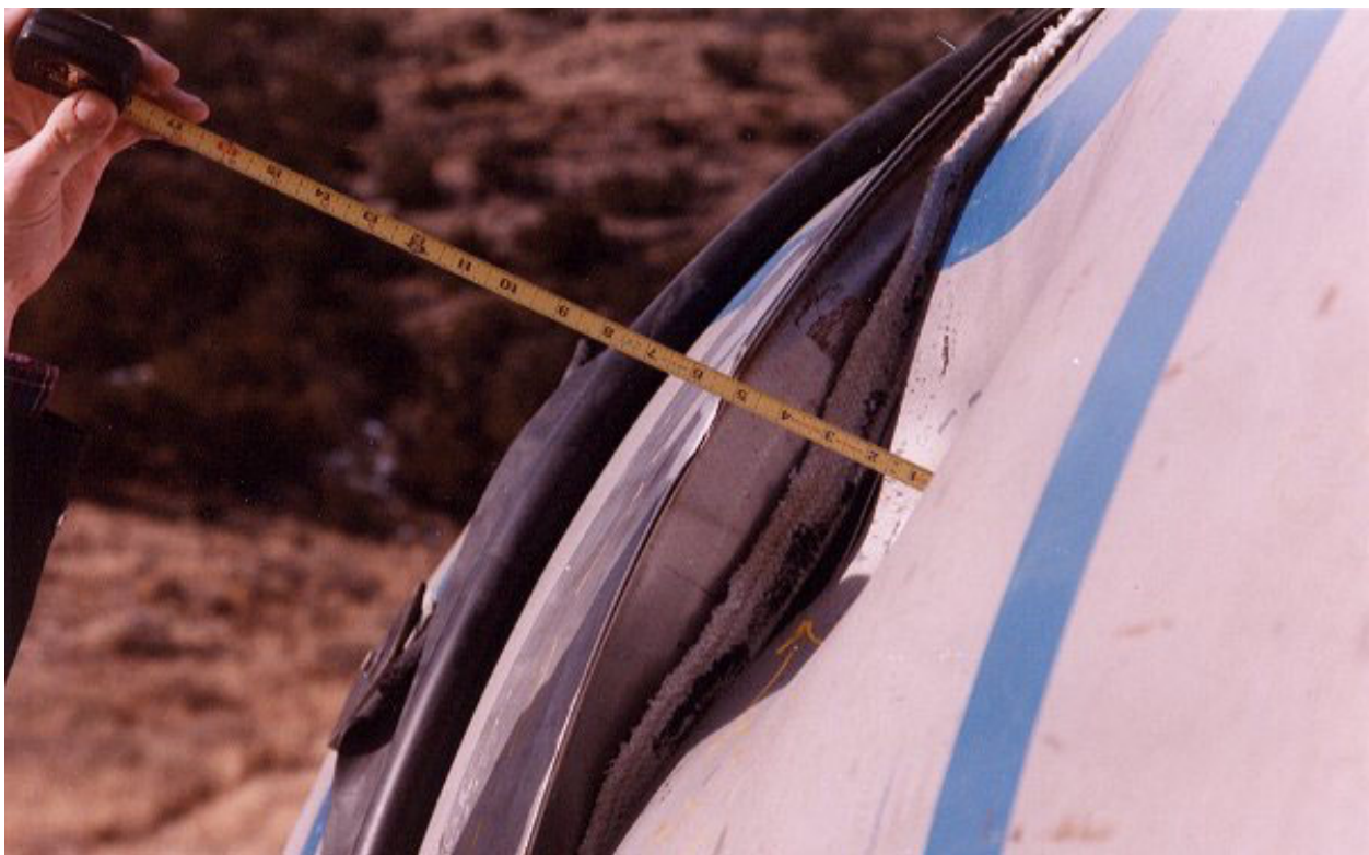
Figure 2.10.3-71 – CTU-2 Puncture Drop 7; Post-Drop Damage
