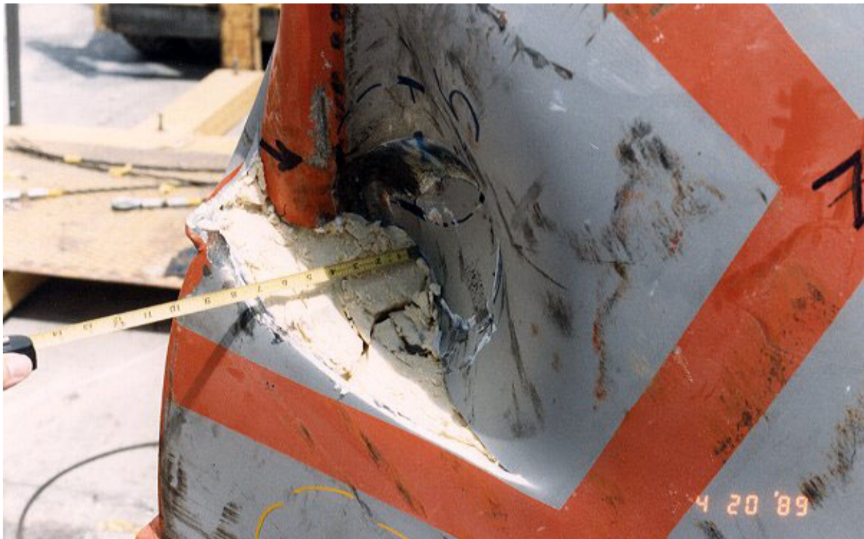
Figure 2.10.3-89 – CTU-3 Puncture Drop 5; Post-Drop Damage
