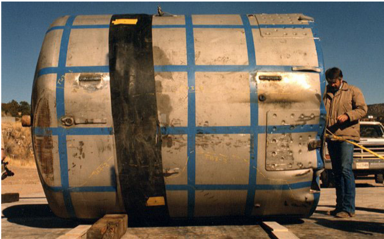
Figure 2.10.3-61 – CTU-2 Free Drop No. 3; Post-Drop Damage
