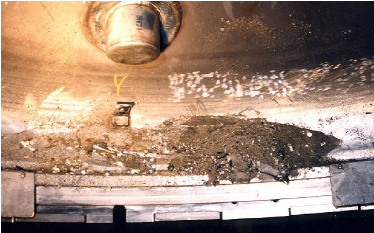
Figure 2.10.3-78 – CTU-2 Disassembly; Loose Debris in ICV Lid
