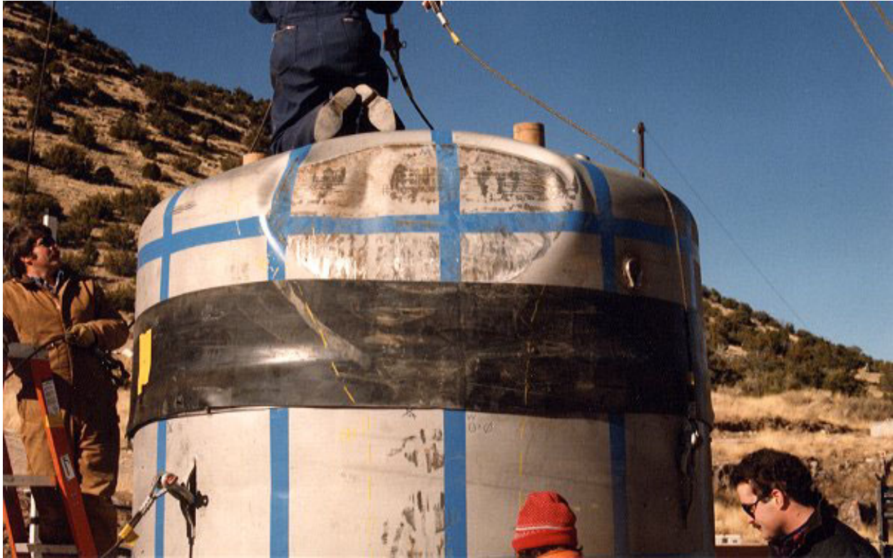
Figure 2.10.3-56 – CTU-2 Free Drop No. 1; Post-Drop Damage
