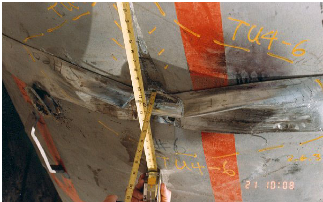
Figure 2.10.3-91 – CTU-3 Puncture Drop 6; Post-Drop Damage
