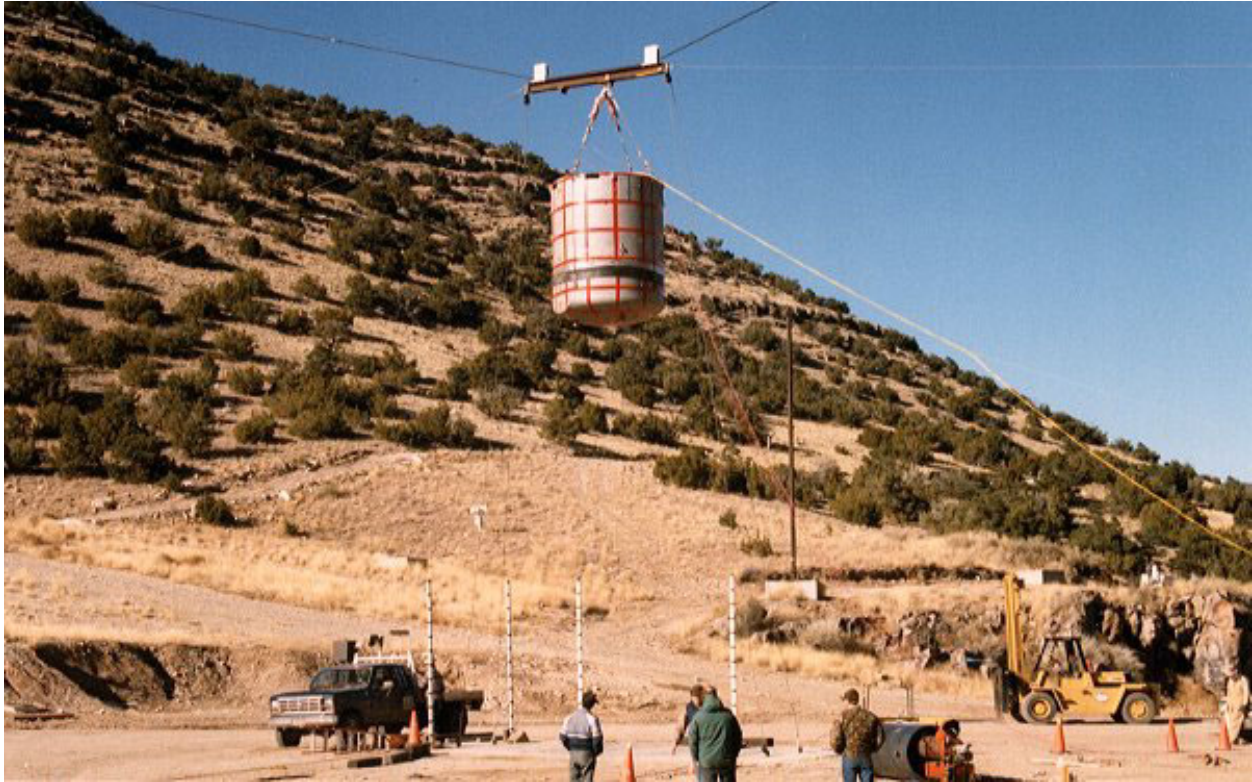
Figure 2.10.3-34 – CTU-1 Free Drop No. 4; Pre-Drop Positioning
