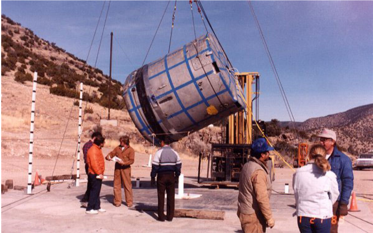
Figure 2.10.3-72 – CTU-2 Puncture Drop No. 8; Pre-Drop Positioning
