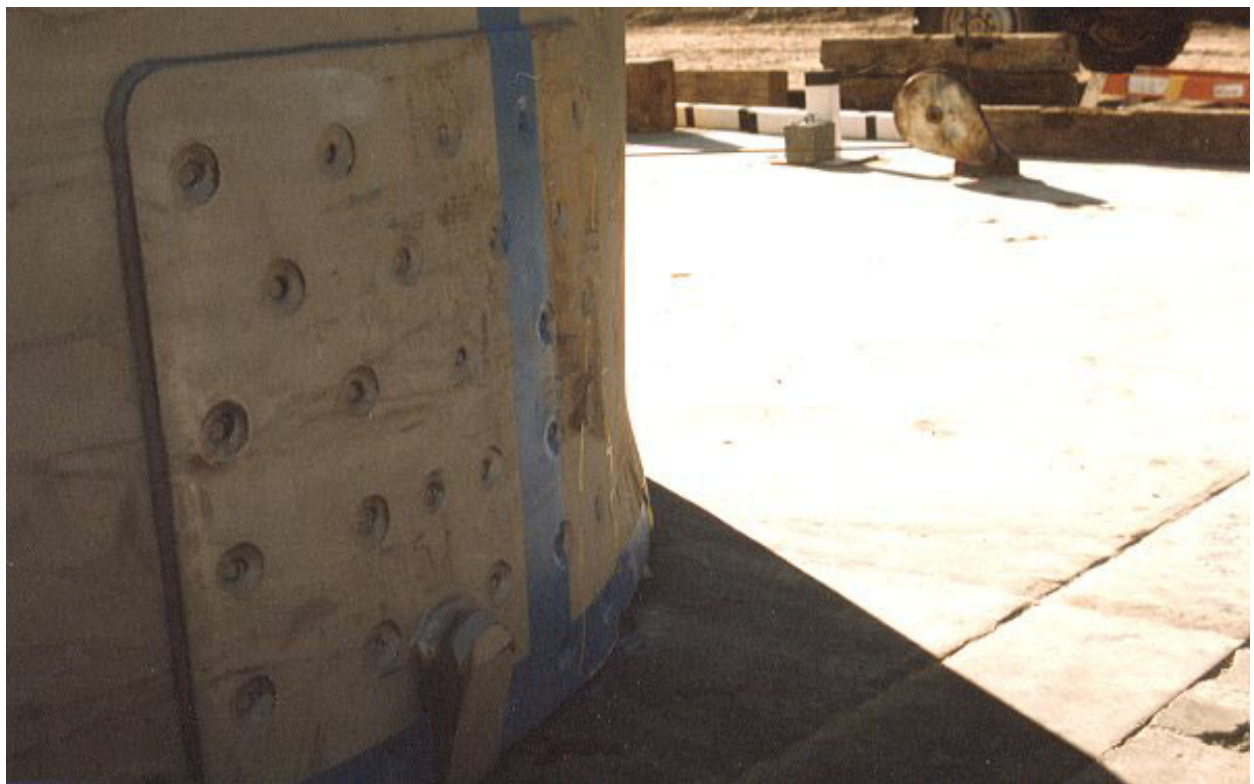
Figure 2.10.3-59 – CTU-2 Free Drop No. 2; Post-Drop Damage
