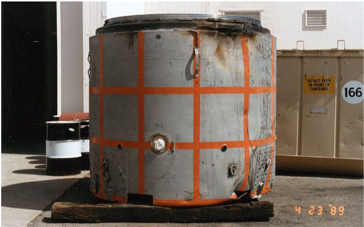
Figure 2.10.3-97 – CTU-3 Disassembly; OCA Body
