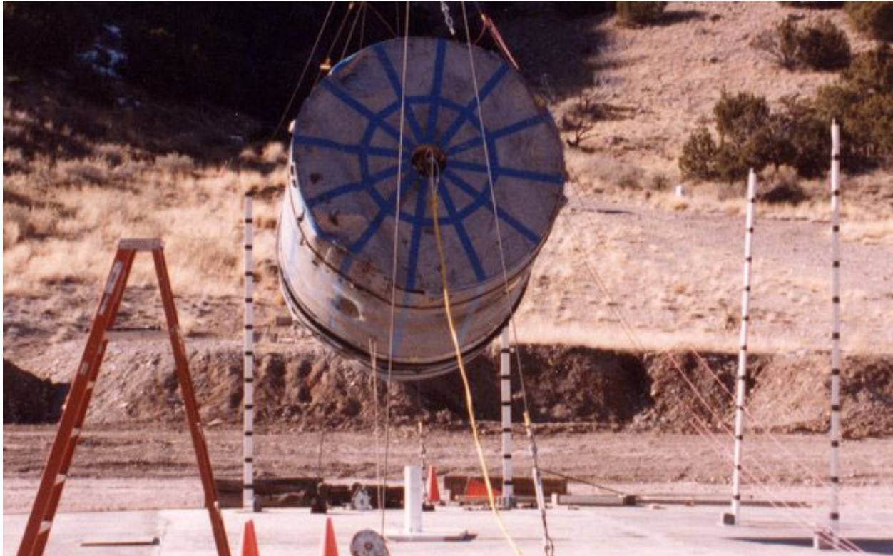
Figure 2.10.3-70 – CTU-2 Puncture Drop No. 7; Pre-Drop Positioning
