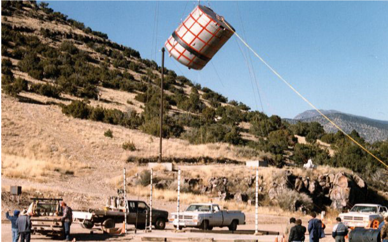
Figure 2.10.3-32 – CTU-1 Free Drop No. 3; Pre-Drop Positioning
