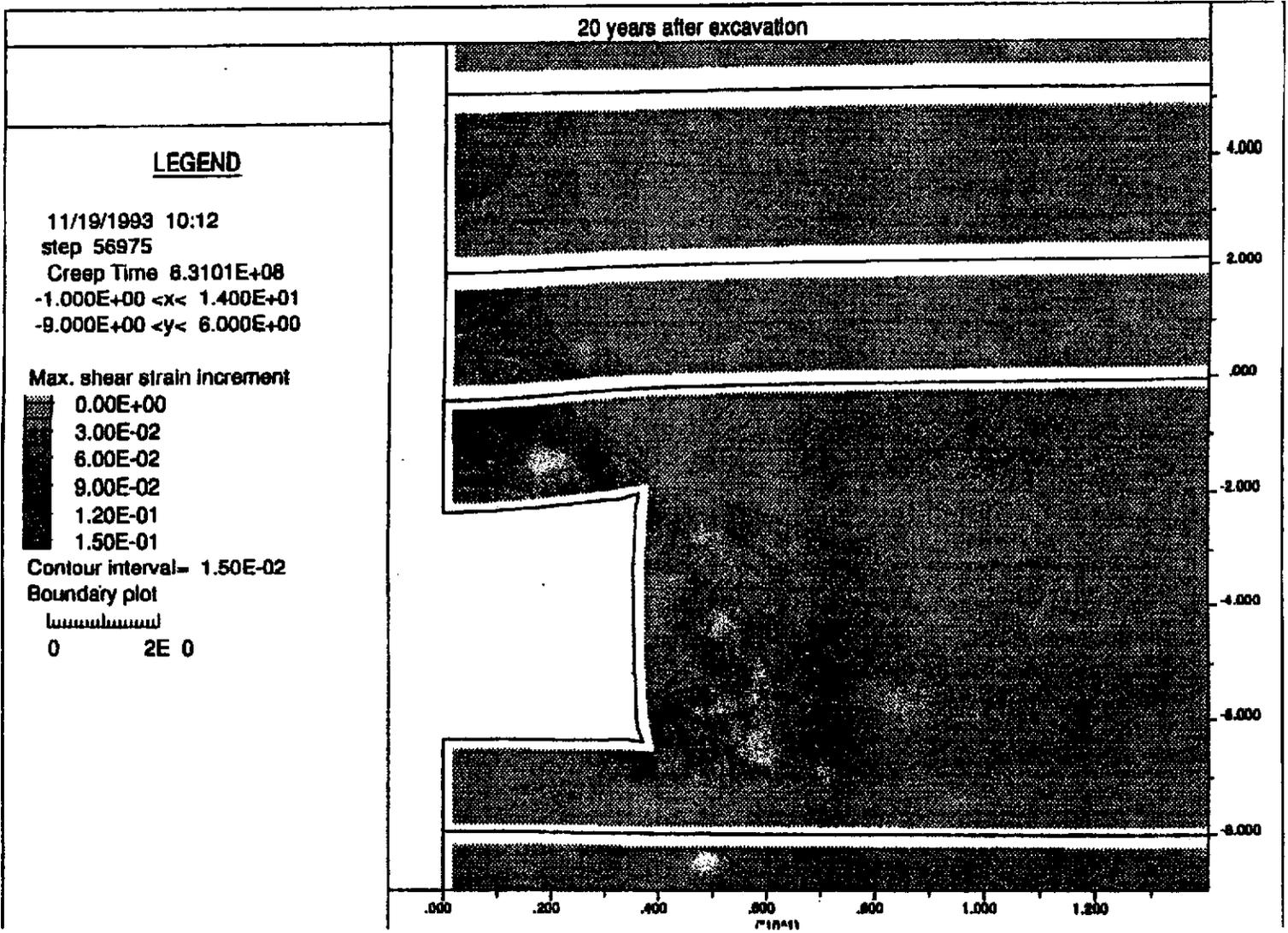
Model Results for E140 Drift With Roof Beam Removed
