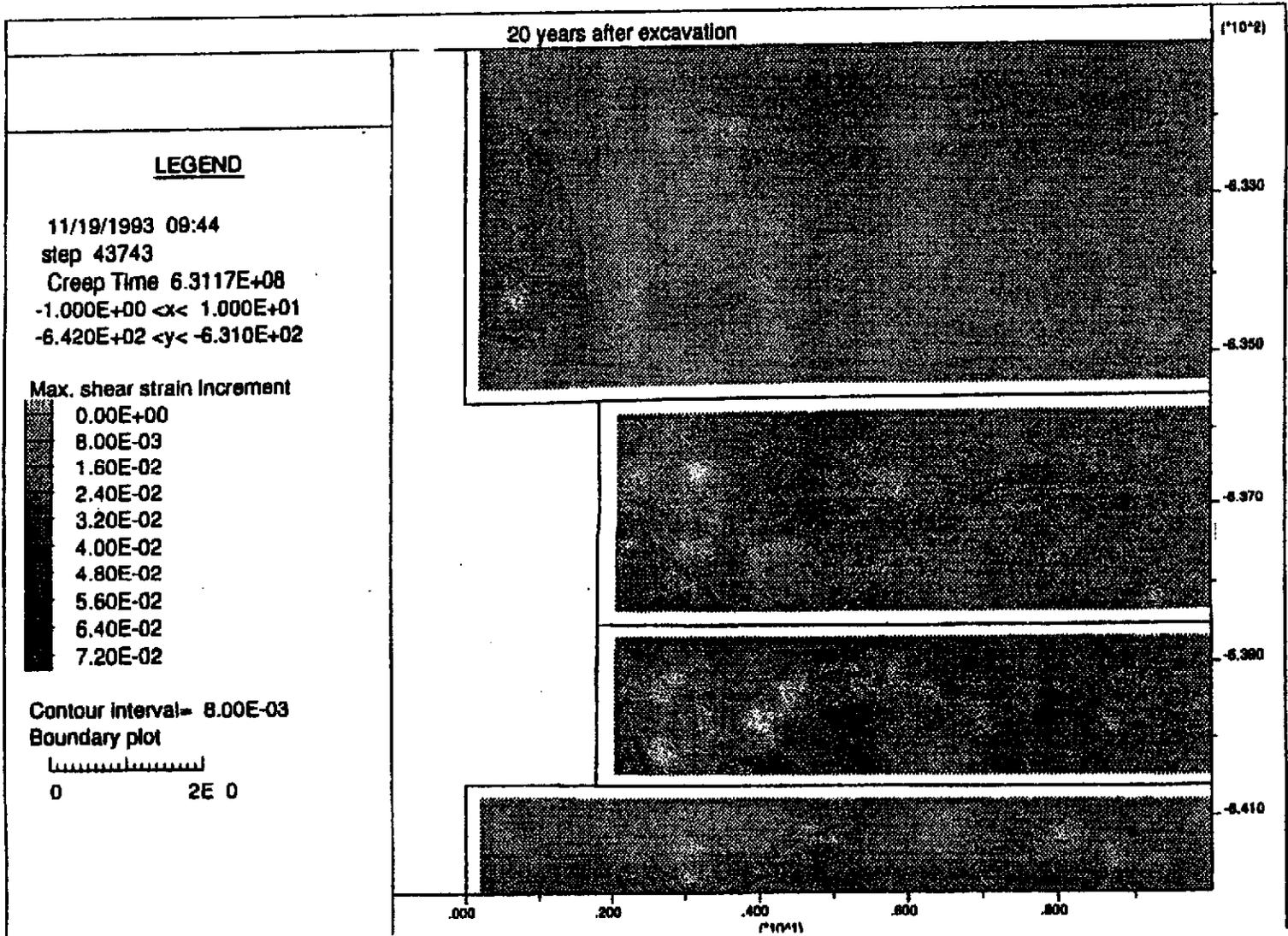
Model Results for E140 Drift Before Roof Beam Removal
