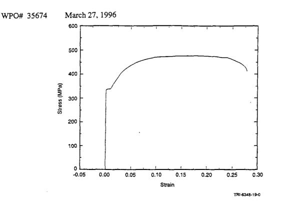
Figure 4.8.1. Stress versus strain curve for a typical ferritic steel exhibiting Lüders strain.
