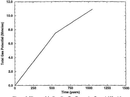
Figure 3. History of the Baseline Gas Generation Potential Used for the Disposal Room Analyses
