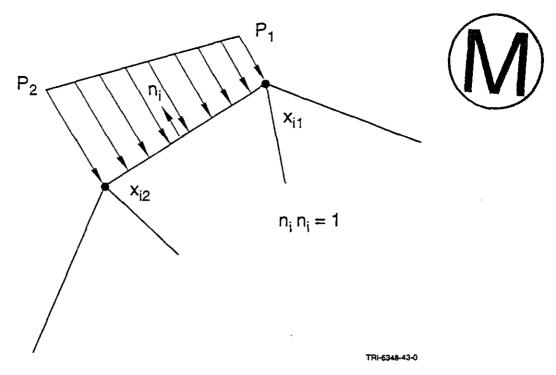
Figure 6.2.1. Definition of a pressure boundary condition along an element side.
