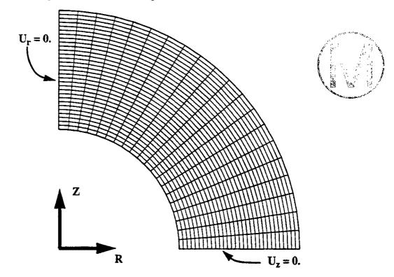
Figure E-8. Finite Element Mesh Discretization Used for the Thick-Walled Hollow Sphere Analyses.
