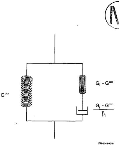
Figure 4.14.1 Mechanical analogy of the standard linear solid.
