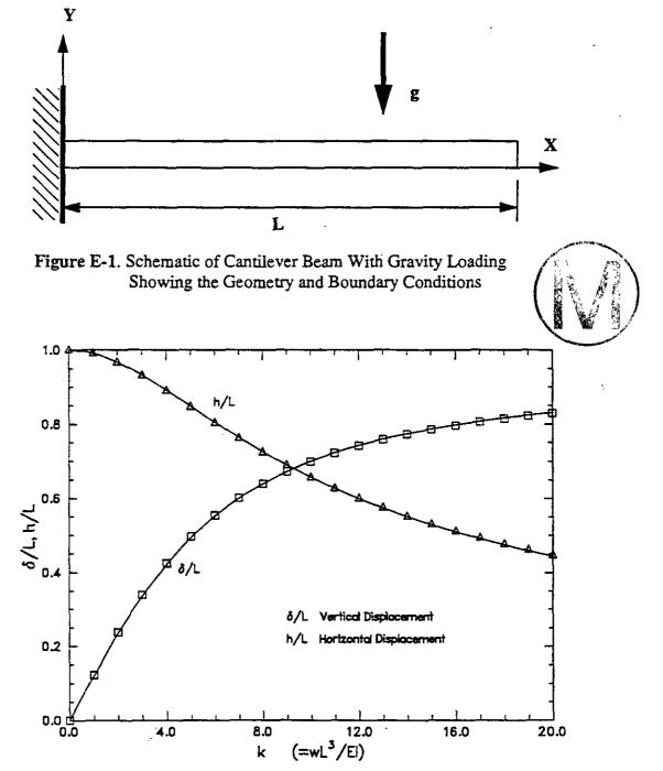
Figure E-2. Comparison of Analytic (solid line) and SANTOS (triangles and squares) Tip Displacements for the Beam With Gravity Loading.
