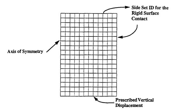
Figure E-12. Mesh Discretization and Boundary Conditions Used for the Analysis of the Upsetting of a Cylindrical Billet.
