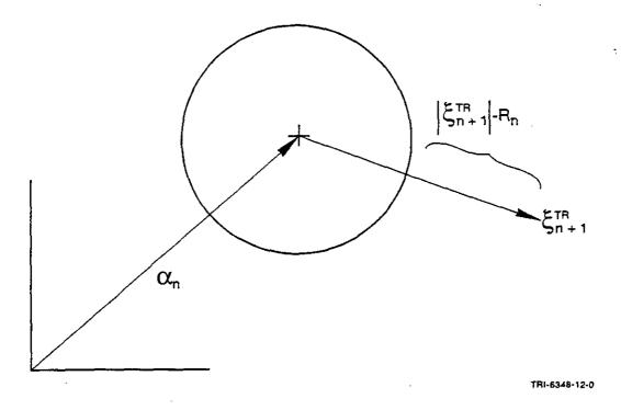
Figure 4.5.6. Geometric interpretation of the radial return correction.
