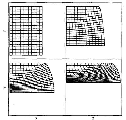
Figure E-13. Plots of the Deforming Billet at Various Times During the Upset. Plots Shown Correspond to Non-Dimensional Times of 0., 0.33, 0.667, and 1.0.
