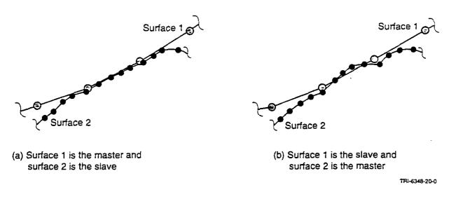
Figure 5.1. Schematic showing the effect of changing the master-slave designation between two surfaces.
