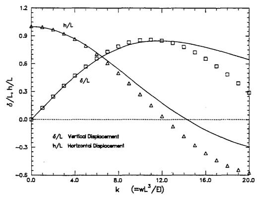
Figure E-6. Comparison of Analytic (solid line) and SANTOS (squares and triangles) Tip Displacements for the Beam With Applied Pressure Loading.
