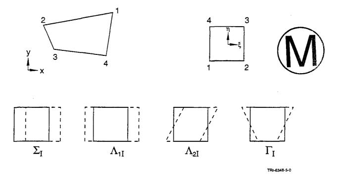
Figure 3.1.1. Mode shapes for the four-node constant strain quadrilateral element.
