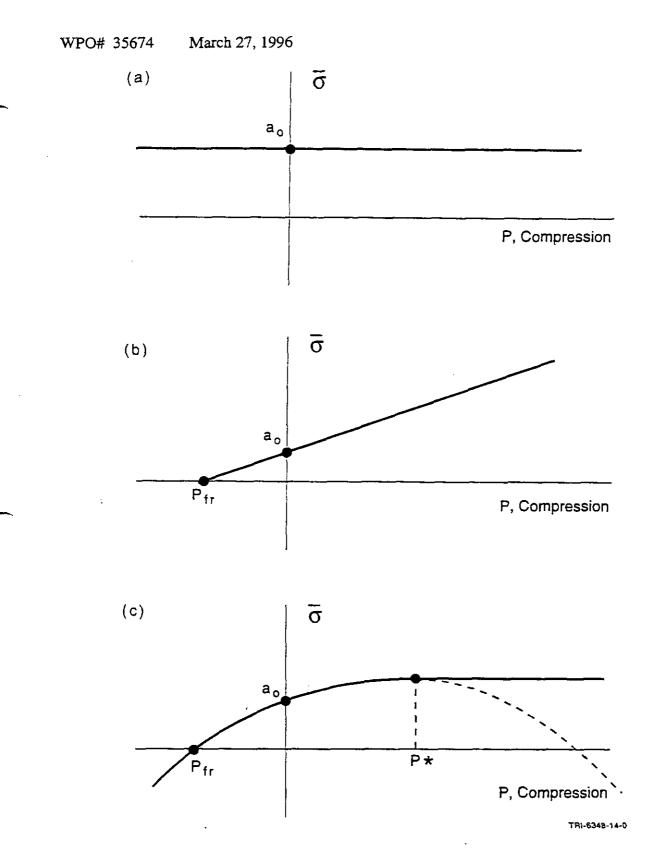
Figure 4.6.2. Forms of valid yield surface which can be defined for the soils and crushable foams material model.
