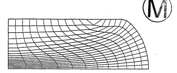
Figure E-14. Final Deformed Shape of the Billet After 60% Upset.
