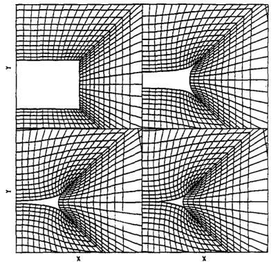
Figure E-18. Plots of the Deforming Disposal Room at Selected Times From Initial Excavation to Final Closure. Times 0., 25. 50., and 80 Years.
