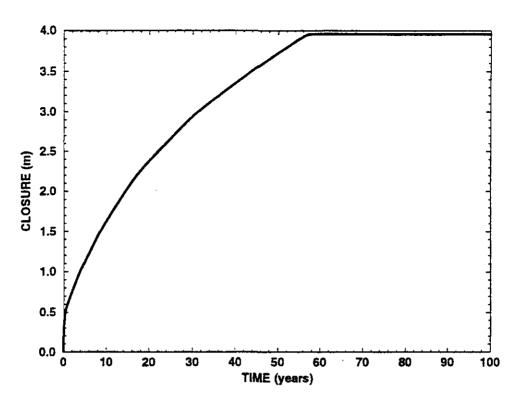
Figure E-20. Closure History of the Disposal Room Centerline. Contact of the Floor and Roof is Reached at Approximately 57 Years.
