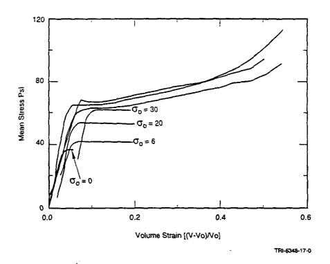
Figure 4.7.2. Foam volume strain versus mean stress for 9505 foam at various confining pressures.
