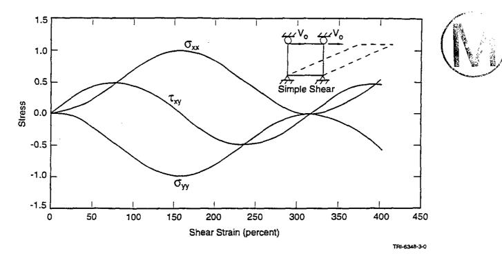
Figure 2.2.1. Computed stress-strain curves for a body undergoing simple shear using the Jaumann rate.
