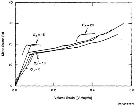
Figure 4.7.1. Foam volume strain versus mean stress for 6602 foam at various confining pressures.
