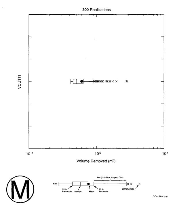
Figure SA-2. Distribution of Original (that is, uncompacted) Volume of Cuttings and Cavings Removed by a Single Drilling Intrusion through CH-TRU Waste
