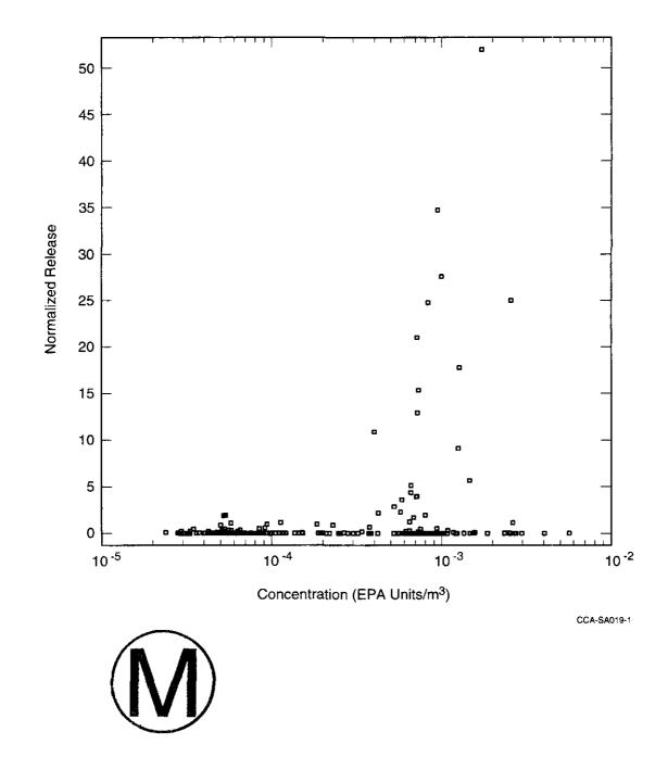
Figure SA-19. Scatterplot for Normalized Release (EPA units) from Repository from Direct Brine Release Resulting from a Single Drilling Intrusion at 10,000 Years into a Previously Unintruded Repository that Passes through CH-TRU Waste in a Lower Waste Panel versus Radionuclide Concentration in EPA units per cubic meter at 10,000 Years
