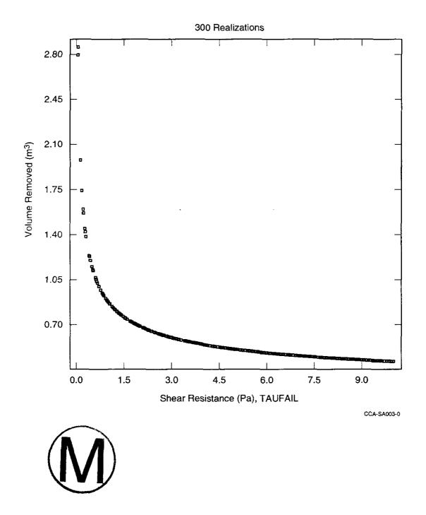
Figure SA-3. Scatterplot for Volume of Material (cubic meters) Removed From Repository Due to a Single Drilling Intrusion through CH-TRU Waste versus Shear Resistance (pascals) for Erosion (TAUFAIL) THIS PAGE INTENTIONALLY LEFT BLANK
