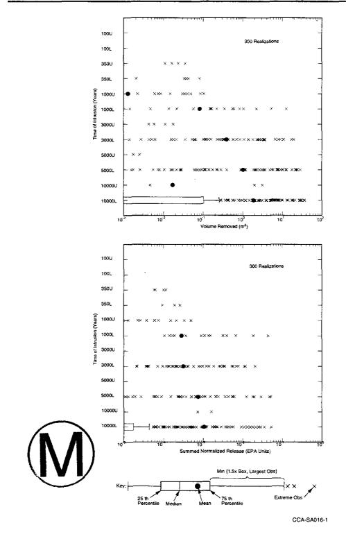
Figure SA-16. Distribution of Brine Release (cubic meters) and Summed Normalized Release (EPA units) from Direct Brine Release for a Single Drilling Intrusion into a Previously Unintruded Repository
