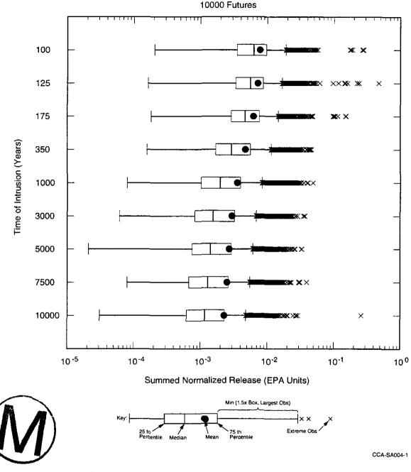
Note: Results calculated with median volume (0.508 cubic meters) from Figure SA-2, 38.6 percent of removed volume assumed to be CH-TRU waste, and a sample size of 1,000 at each time.
