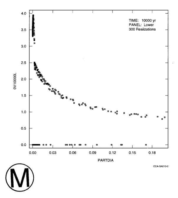
Figure SA-10. Scatterplot for Volume of Material (cubic meters) Removed from Repository due to Spallings Resulting from a Single Drilling Intrusion at 10,000 Years into a Previously Unintruded Repository that Passes through CH-TRU Waste in Lower Waste Panel versus Logarithm of Diameter of Particles Available for Removal by Spallings (PARTDIA) Title 40 CFR Part 191 Compliance Certification Application
