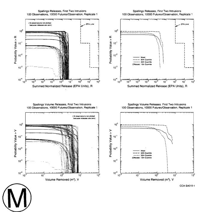
Figure SA-15. Distributions of CCDFs for Summed Normalized Release to Accessible Environment and Volume of Material (cubic meters) Removed to Accessible Environment over 10,000 Years due to Spallings with the Assumption that Spallings Releases Will Occur Only for the First Two Drilling Intrusions into the Repository
