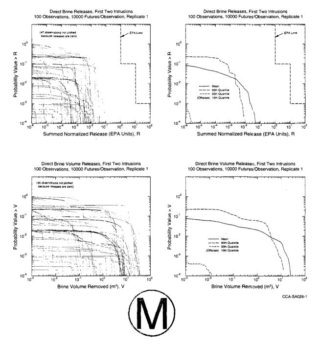
Figure SA-26. Distributions of CCDFs for Summed Normalized Release to Accessible Environment and Volume of Brine (cubic meters) Removed to Accessible Environment over 10,000 Years due to Direct Brine Releases with the Assumption that Direct Brine Releases Will Occur Only for the First Two Drilling Intrusions into the Repository
