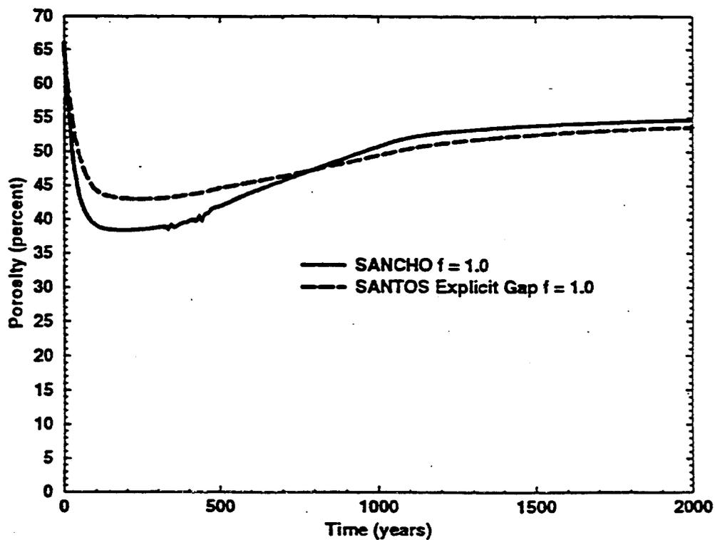
Figure 9. Comparison of Effective Disposal Room Porosity Calculations Between a Reference Model Analysis With SANCHO and SANTOS With the Headspace Explicitly Modeled.
