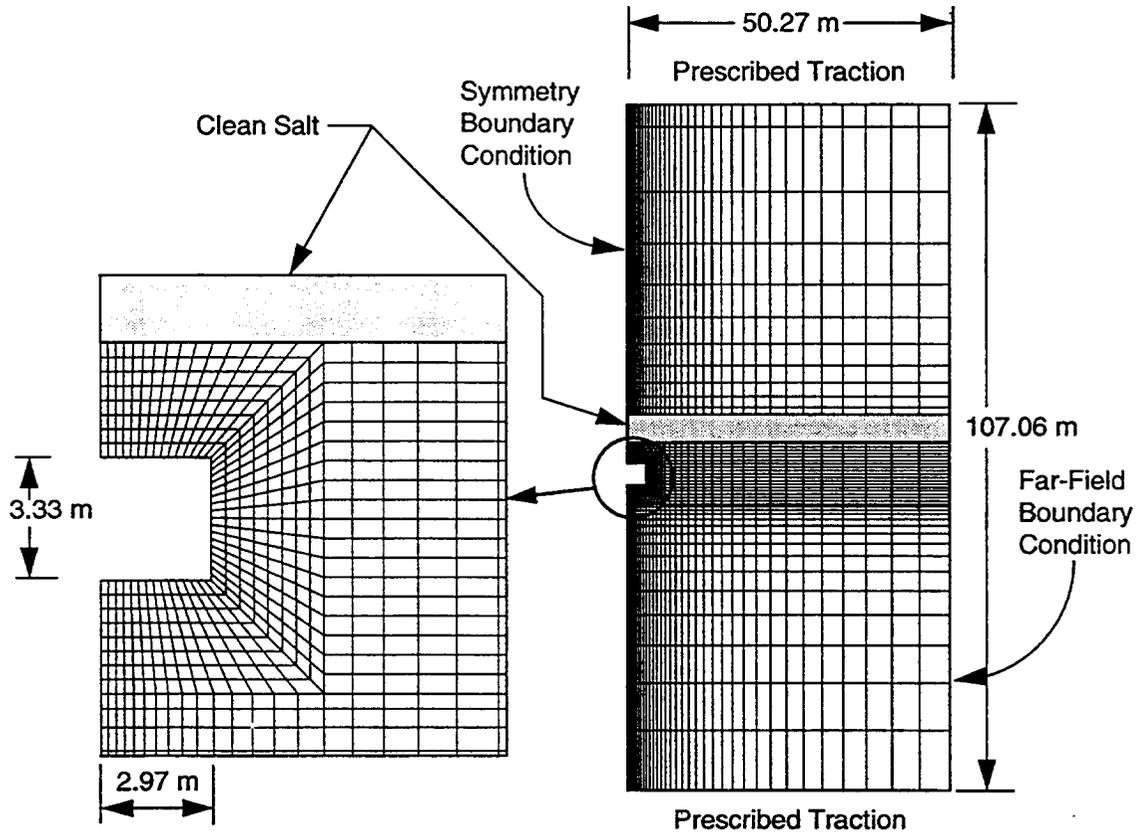
**Figure 3.** Finite Element Mesh and Boundary Conditions Used in SANTOS Analyses
