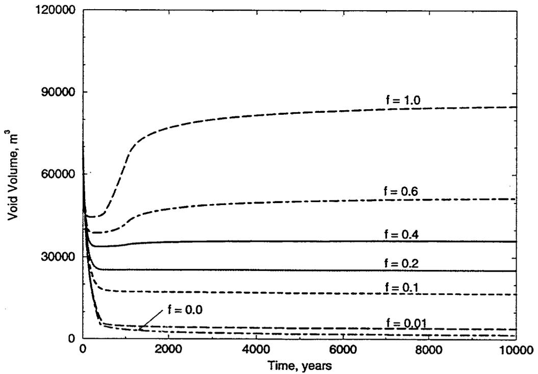
Figure 5 Room Volume Histories for “Equivalent” Room at WIPP North End
