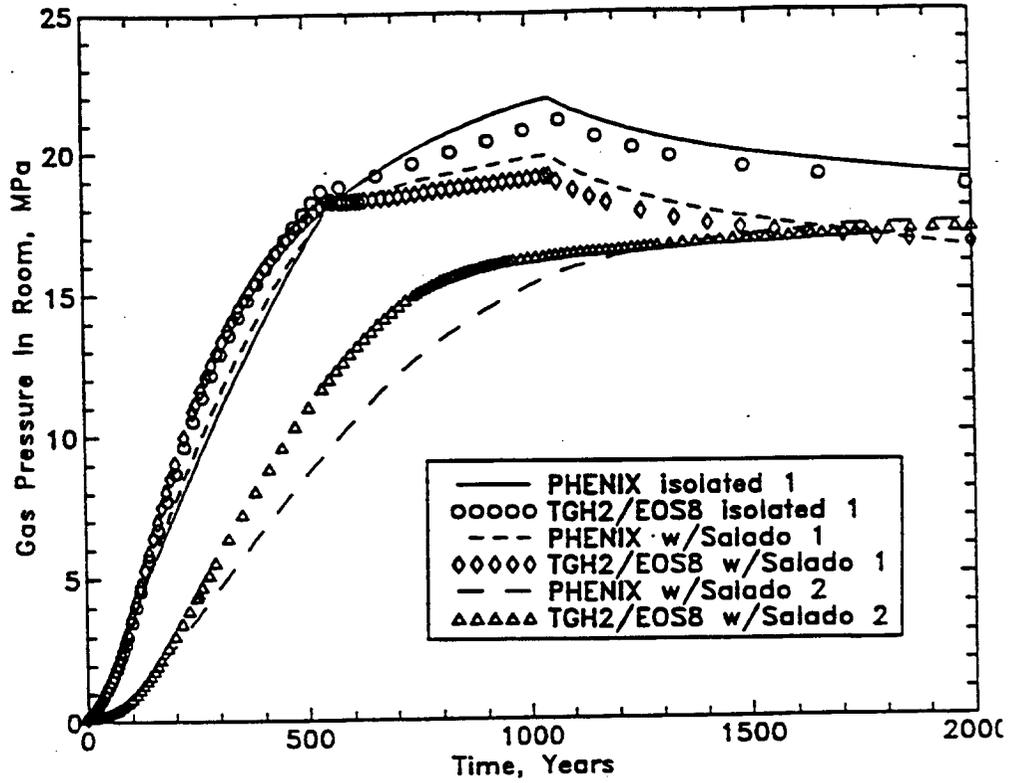
Figure 11. Comparison of gas pressure for several simulations calculated with PHENIX to comparable simulations calculated with the Fluid-Phase Salt method in TOUGH2/EOS8. Sealed room, halite and interbed, and brine dependent gas generation rate results are plotted.
