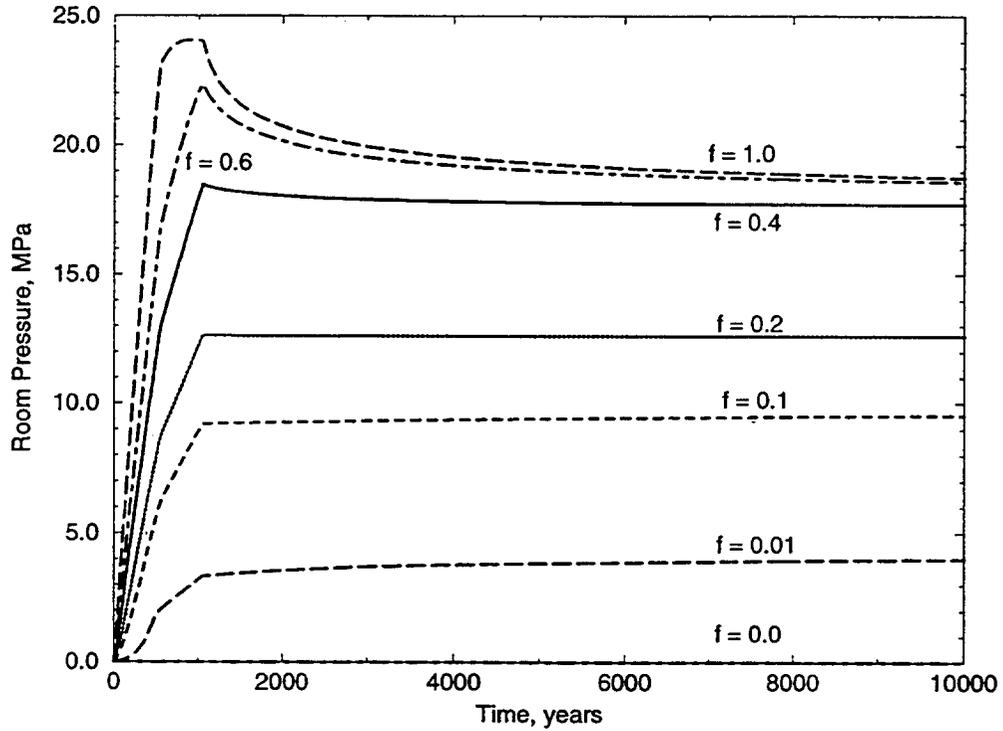
Figure 4 Room Pressure Histories for “Equivalent” Room at WIPP North End
