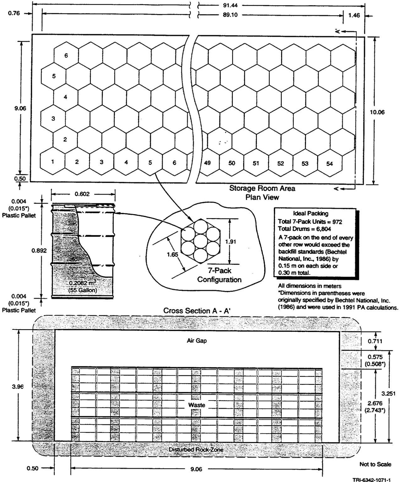
Figure 5. Ideal packing of drums in rooms and 10-m-wide drifts (not to scale). (From Sandia WIPP Project, 1992, Figure 2.1-4, p. 3.5.)
