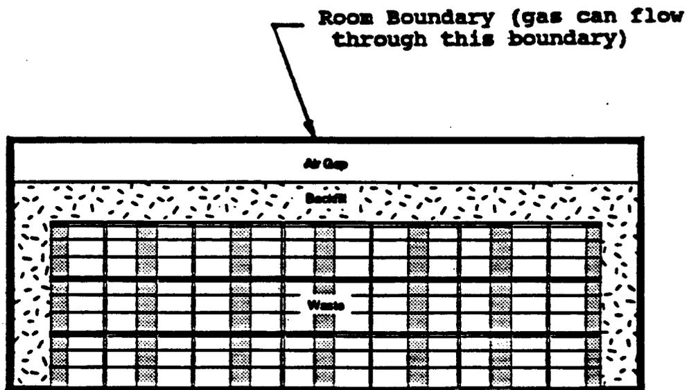
**Figure 6:** The boundary of the disposal room assumed for calculations. The room is not sealed and gas can flow through the boundary at any time during closure. However, when a specific quantity of gas is quoted it refers to the amount of gas contained inside the boundary.
