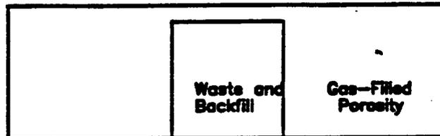
No contact between the backfill and the room ceiling: the ceiling is supported entirely by gas pressure.
