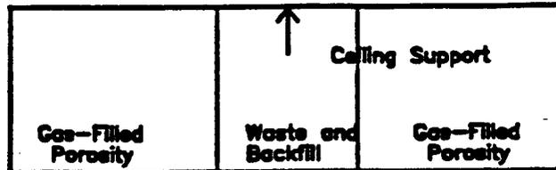
Waste and backfill in contact with room ceiling, partially supporting it.
