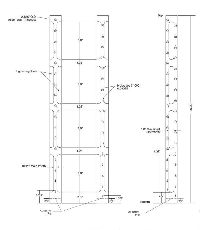
Figure C-4. SWB matrix surrogate PDP standard insert fixture.
