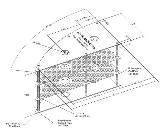
Figure C-3. End type SWB matrix module.
