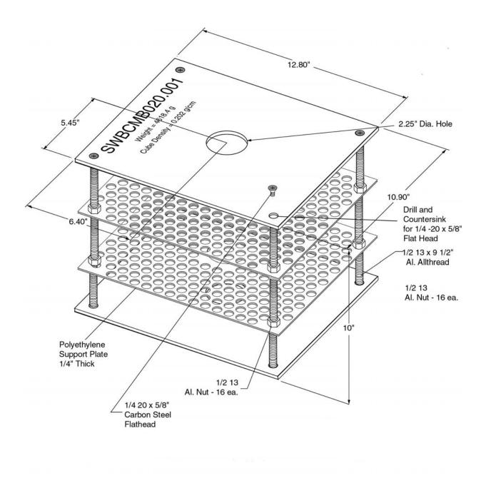
Figure C-2. Center type SWB matrix module.
