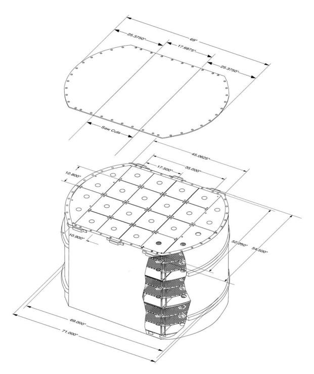
Figure C-1. Cutaway isometric of SWB matrix surrogate.
