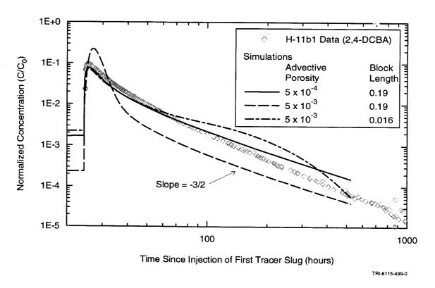
Figure 4-7. Simulated concentration vs. time curves for H-11 SWIW test for different advective porosities and matrix block lengths compared to observed data (Meigs et al., 1997).
