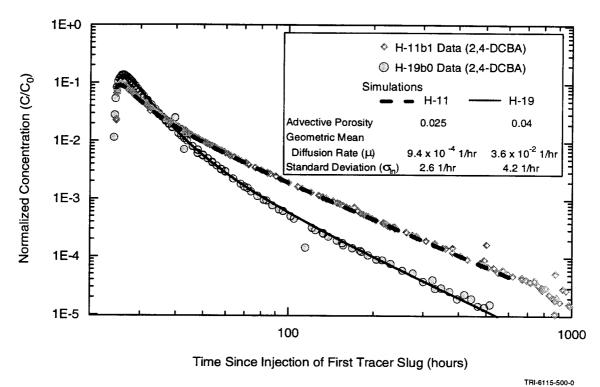
Figure 4-8. Simulated concentration vs. time curves for H-11 and H-19 SWIW tests with the multirate, double-porosity model plotted with observed data (Meigs et al., 1997).
