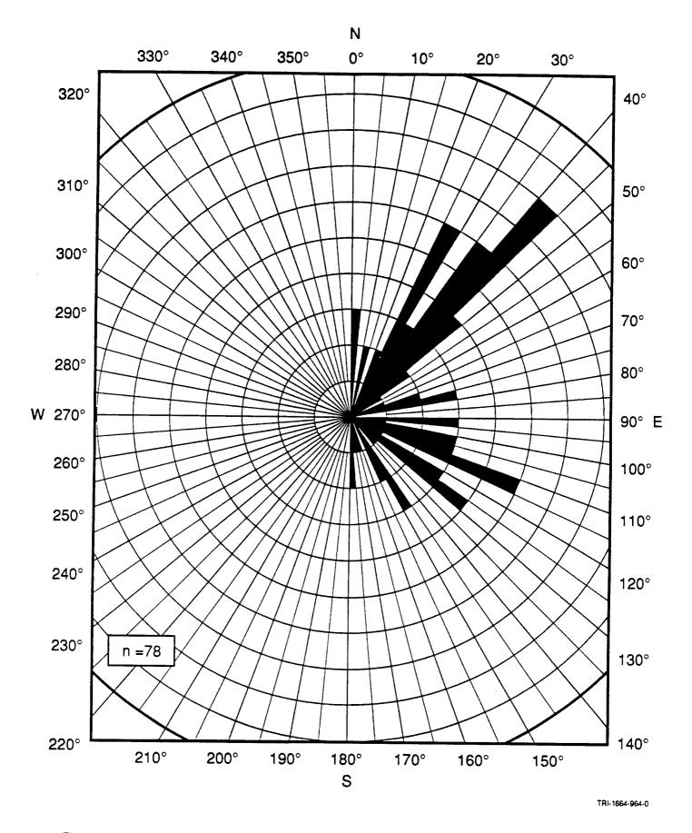
Figure 5. Strike of High-Angle Joints at Location 3 (Culebra Dolomite northeast of "L-R Hill," section 19, T23S,R30E and section 24, T23S,R29E).
