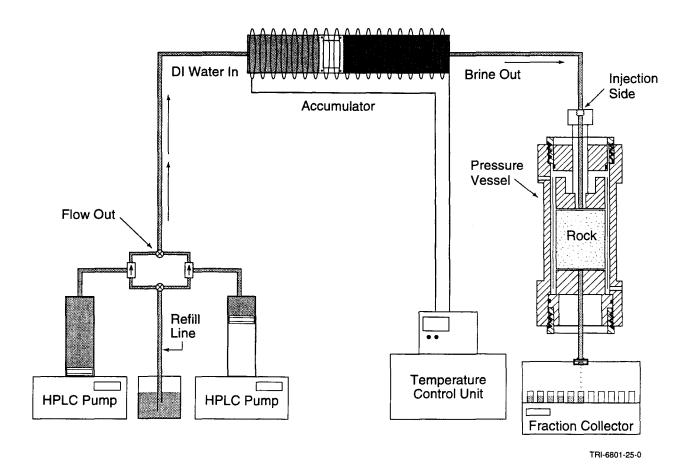
Figure 4-1. Schematic diagram of apparatus used for retardation experiments.
