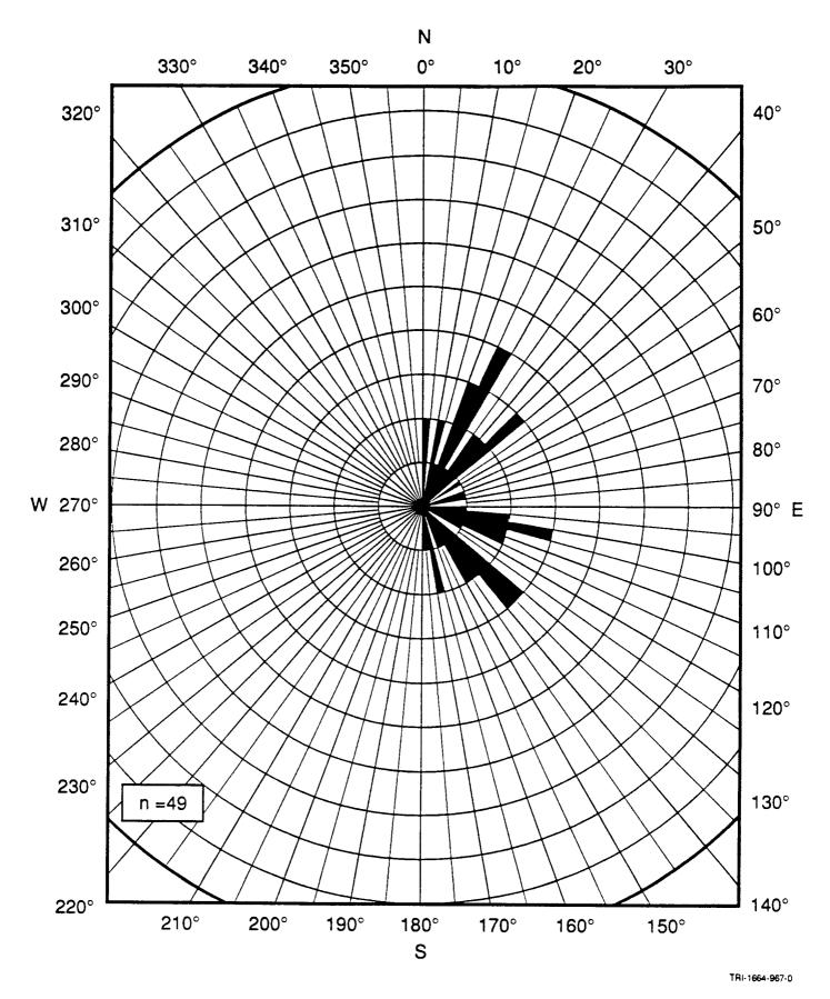
Figure 8. Strike of High-Angle Joints at Location 6 (Dewey Lake Red Beds in section 15, T22S,R30E, northeast of WIPP-25).
