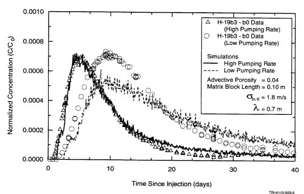
Figure 4-11. Simulated breakthrough curves for multiple-well convergent-flow test data, H-19b3-b0 path, using heterogeneous, single-rate double-porosity model for two different pumping rates.
