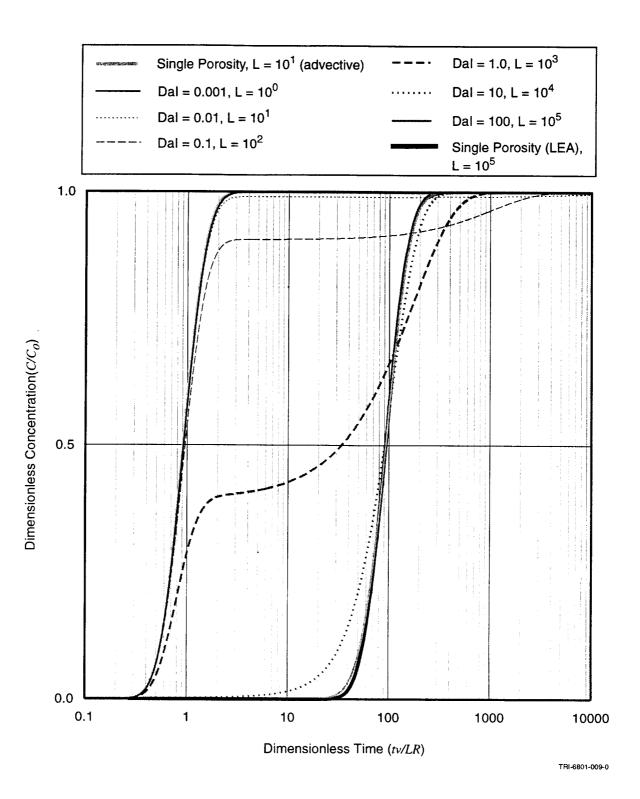
Figure 3-2. Simulated breakthrough curves for one-dimensional transport in a double-porosity, single-rate medium. To provide reference, single porosity breakthrough curves equivalent to Equations 3-12 and 3-14 are shown. The boundary condition at the inlet is an infinite duration, step increase in concentration.
