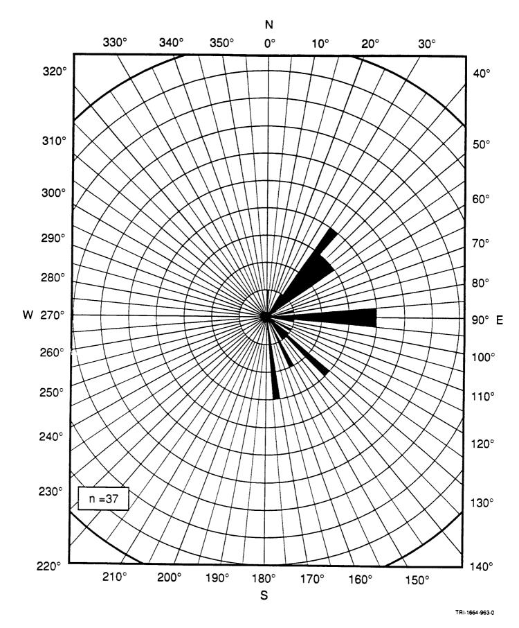
Figure 4. Strike of High-Angle Joints at Location 2 (Culebra Dolomite in and near roadside quarry, section 18, T23S,R30E).
