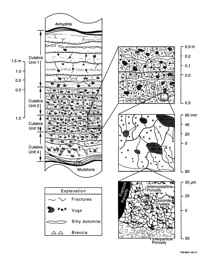
Figure 2-1. Scales of porosity in the Culebra.
