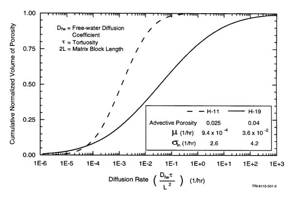
Figure 4-9. Diffusion rate coefficient cumulative distribution function for H-11 and H-19 SWIW test simulations shown in Figure 4-8 (Meigs et al., 1997).
