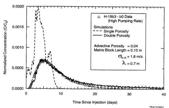
Figure 4-10. Simulated breakthrough curves for multiple-well convergent-flow test data, H-19b3-b0 path, using heterogeneous, single- and double-porosity models (Meigs et al., 1997).
