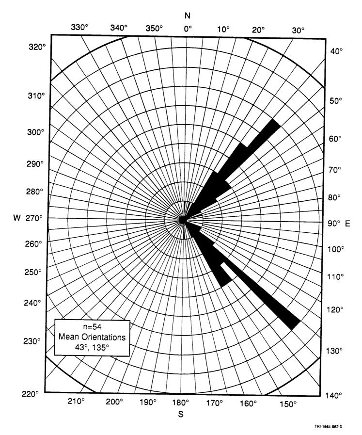
Figure 3. Strike of High-Angle Joints at Location 1 (Culebra Dolomite at Culebra Bluff, sections 2 and 11, T23S,R28E).
