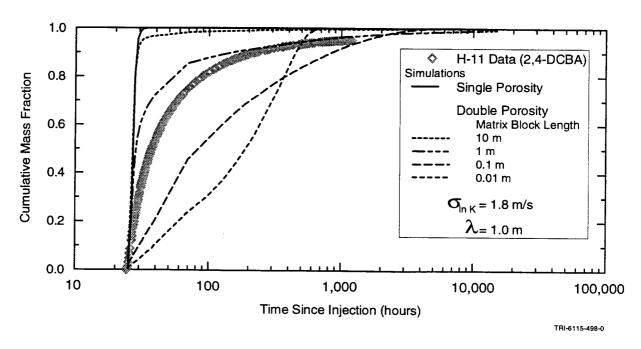
Figure 4-6. Simulated mass recovery curves for H-11 SWIW test for different advective porosities and matrix block lengths compared to observed data (Meigs et al., 1997).
