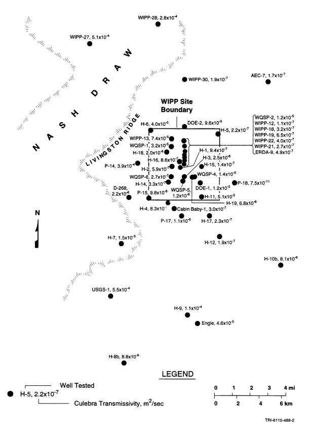
Figure 1-10. Culebra test locations and estimated transmissivity (data from Beauheim, 1996)
