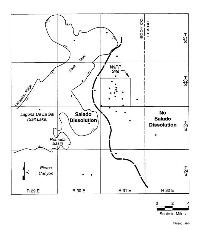
Figure 1-6. Margin of Salado dissolution in the vicinity of the WIPP site (Powers and Holt, 1995b).
