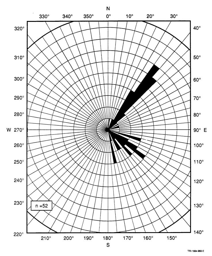
Figure 7. Strike of High-Angle Joints at Location 5 (Magenta Dolomite in railroad cut, section 18, T23S,R30E).
