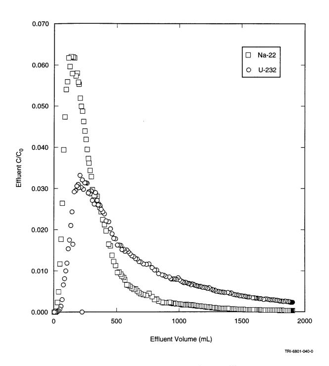
Figure 4-2. Results of a typical elution experiment using <sup>22</sup>Na and <sup>232</sup>U as conservative and sorbing tracers, respectively.
