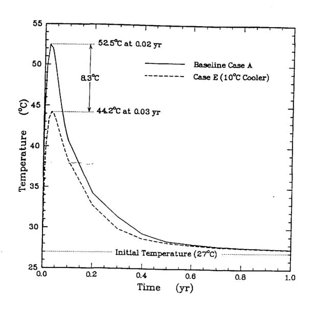
Figure 5-5. Effect of Initial Cooling — SMC3 Midpoint Temperatures for Case E.
