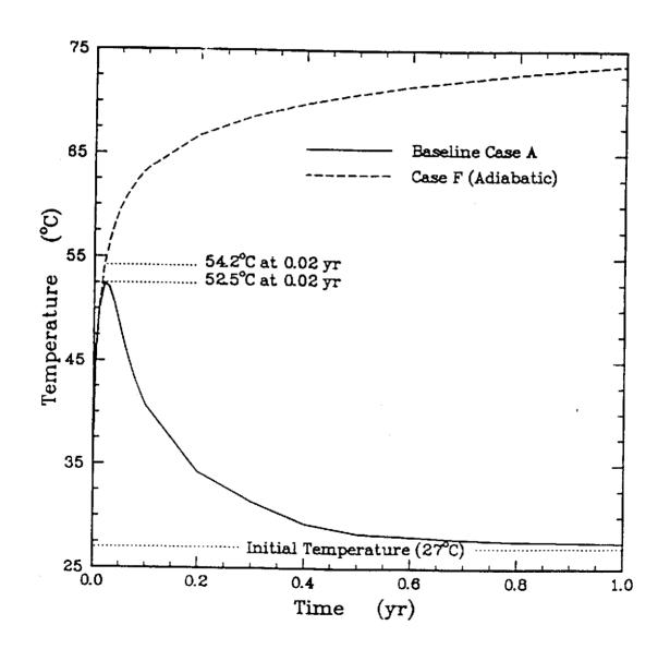
Figure 5-6. Effect of Heat Transfer to Salt — SMC3 Midpoint Temperatures for Case F.
