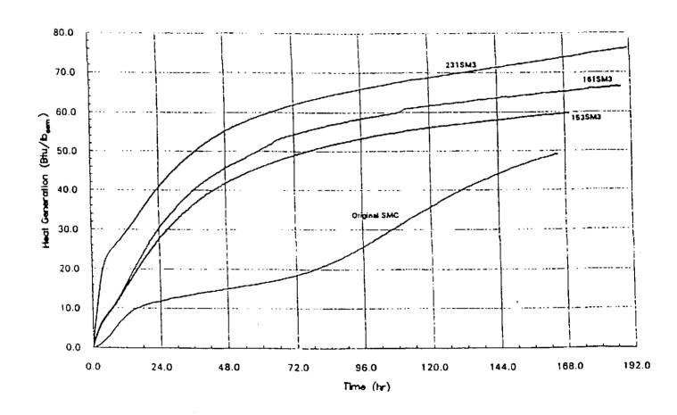
Figure 2-1. Heat Generation of Salado Mass Concrete Mixtures.
