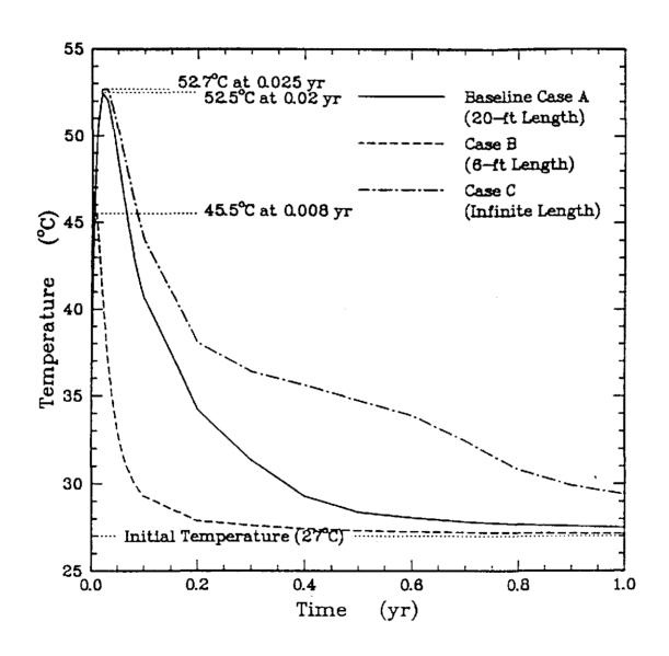
Figure 5-3. Effect of Seal Length — SMC3 Midpoint Temperatures for Cases B and C.
