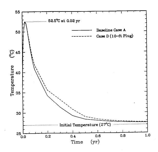
$\mbox{ Figure 5-4. } \mbox{ Effect of Room Properties} -- \mbox{SMC3 Midpoint Temperatures for Case } D.$
