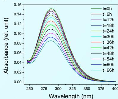
Absorption spectra showing the decomposition of hypochlorite ion in 5M NaCl simplified brine ( $[\text{OCl}^-]_{\text{initial}} = 2 \text{ mM}$  at  $\text{pH} = 10.7$ ).
