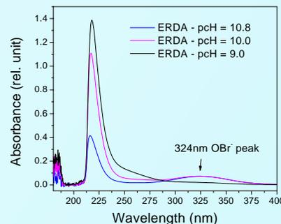
Absorption spectra showing the hypobromite peak at 324 nm in ERDA-6 at pH 9,10 and 10.8.
