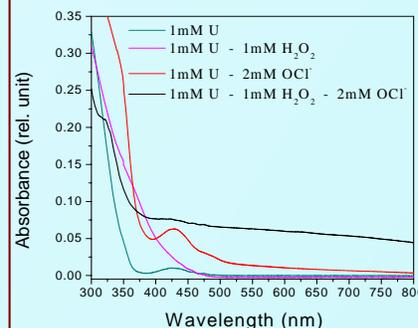
Absorption spectra of four U- $\text{H}_2\text{O}_2$ - $\text{OCl}^-$  mixtures in 5M NaCl brine show evidence for a uranyl complexes with  $\text{H}_2\text{O}_2$  and/or  $\text{OCl}^-$ .
