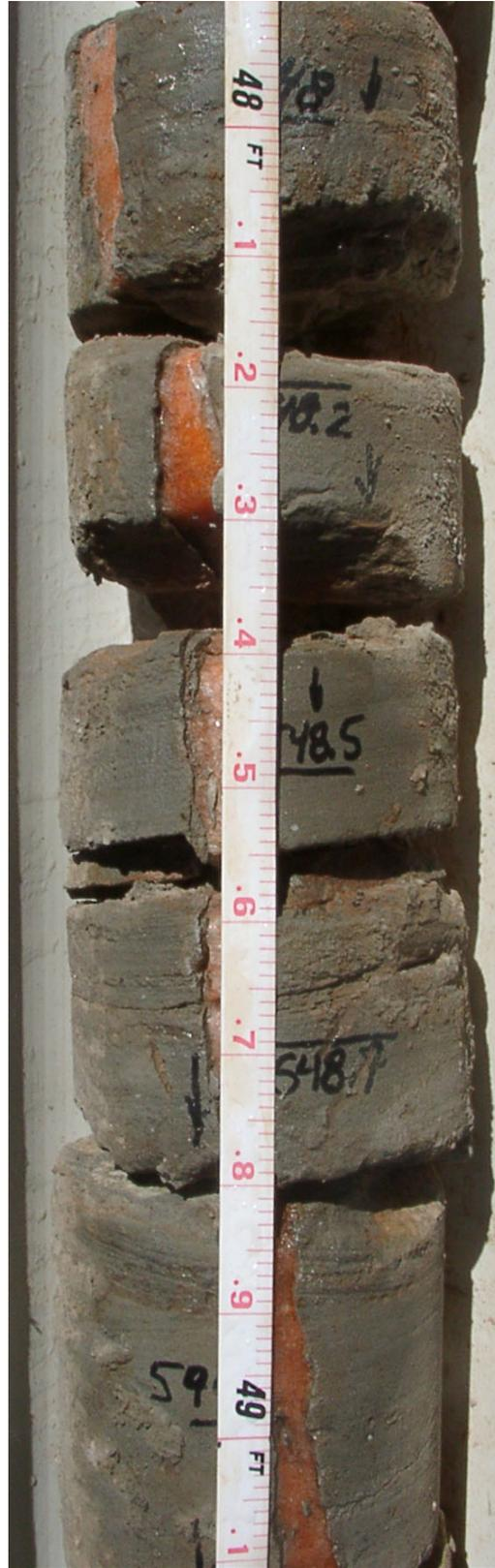
Note: fracture fits together with small aperture
