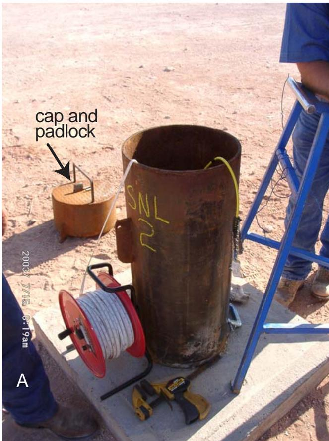
A - Surface casing for SNL-2 with cap and padlock (open for work to prepare well for water level monitoring).
