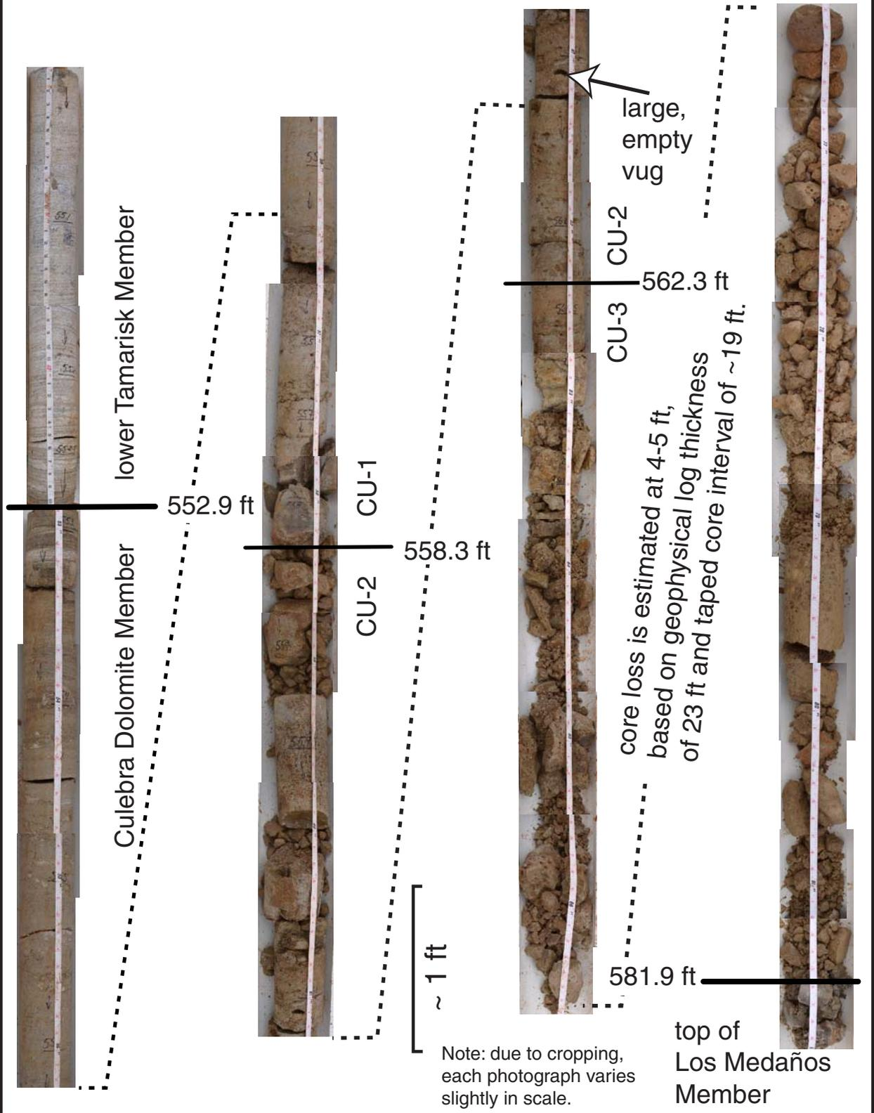
The basal 22.9 ft and upper 8.6 ft of the Tamarisk were cored; the remainder of the unit is described on the basis of cuttings and geophysical logs.
