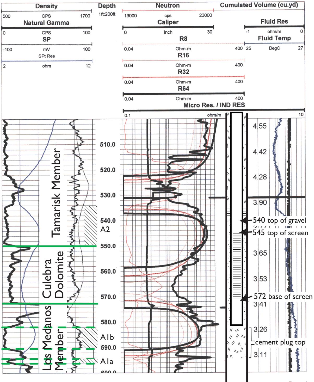
Preliminary Selection of Screened Interval, Cement Plug, and Gravel Pack Interval for SNL-9
