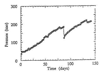
Figure 1. Pressure buildup as a function of time for Plutonium-spiked WIPP BRINE
