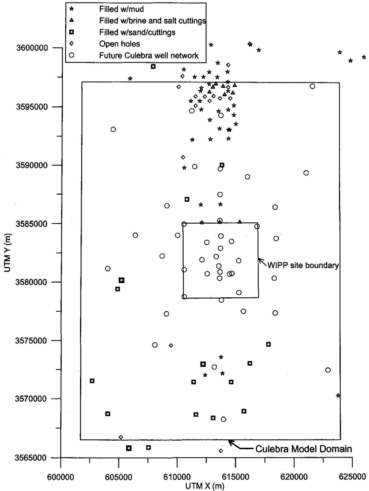
Figure 7. Potentially leaky potash holes.
