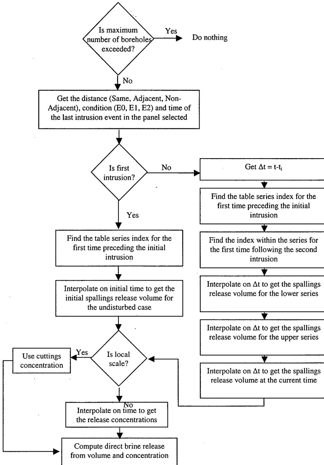
Figure 15. Computation of Spallings Releases.
