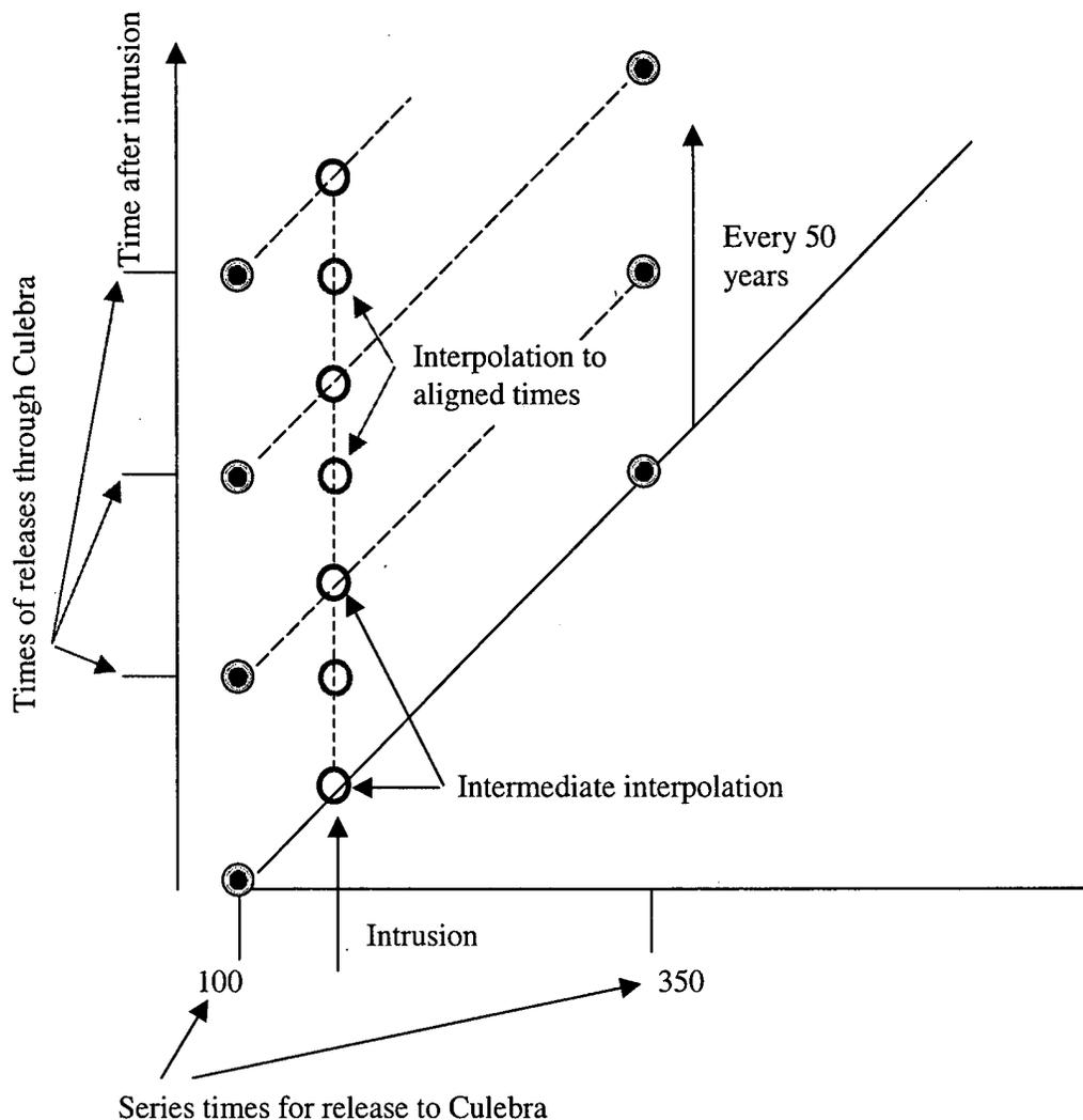
Figure 17. Interpolation for Release to Culebra for a Single Intrusion
