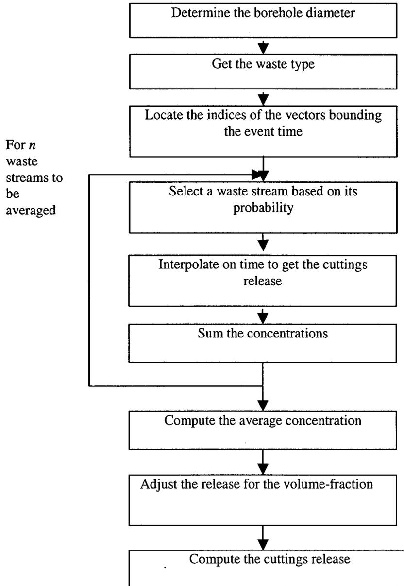
Figure 11. Calculation of Cuttings Releases.
