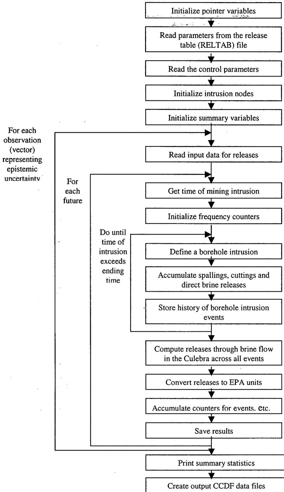
Figure 18. Flow of processing of input data to produce CCDFs.
