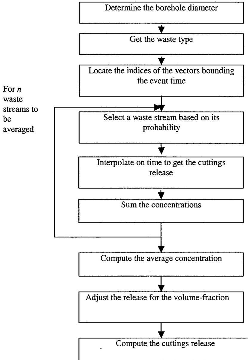
Figure 11. Calculation of Cuttings Releases.
