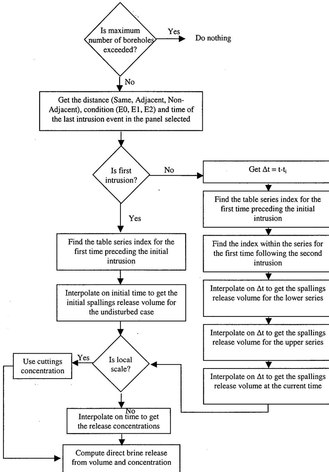
Figure 15. Computation of Spallings Releases.
