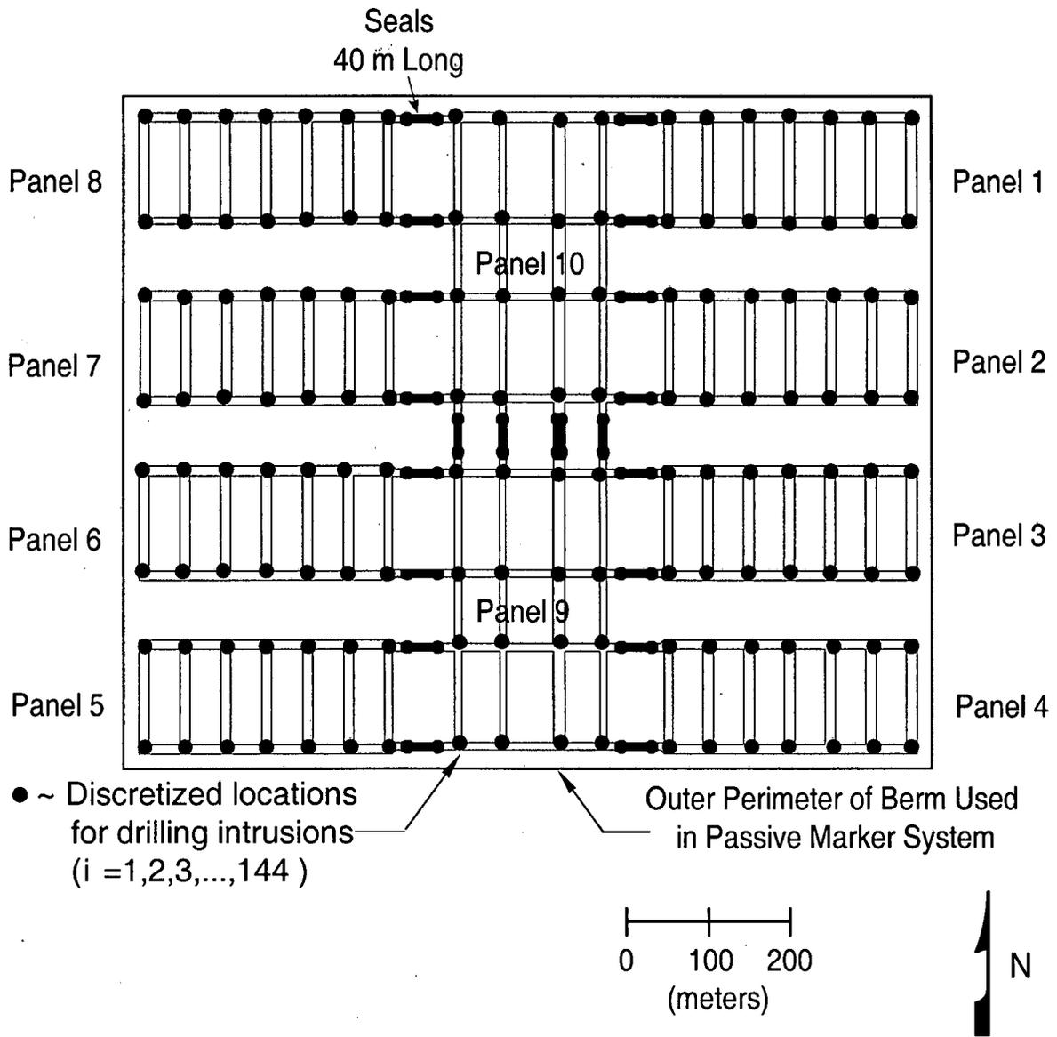
Figure 10. The location of drilling nodes.
