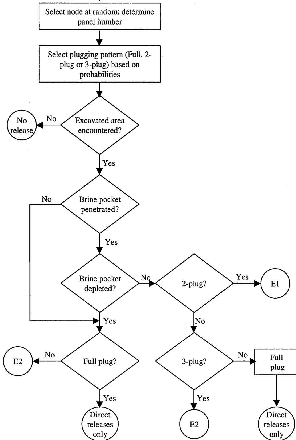
Figure 12. The determination of the type of intrusion.
