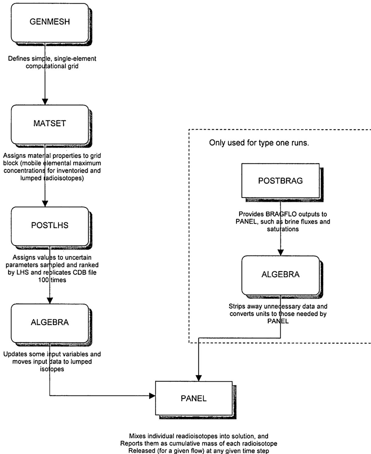
Figure 1: The run sequence for PANEL in a 2003 CRA PANEL run. Process codes are square and support codes are rounded..
