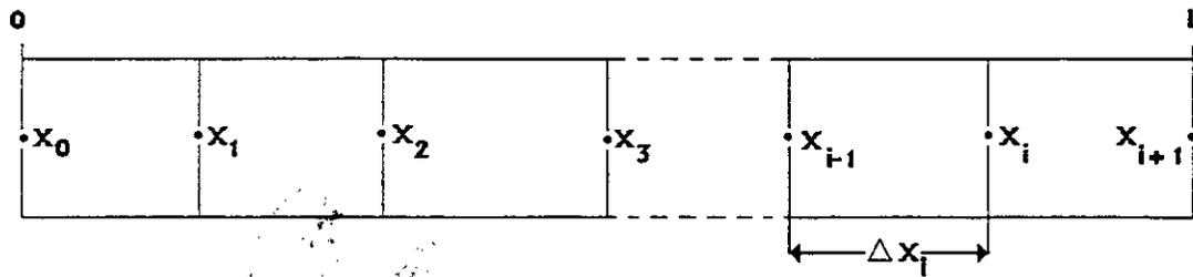
**Figure 4.4 Point-Center Grid in Finite-Difference Approximation.**
