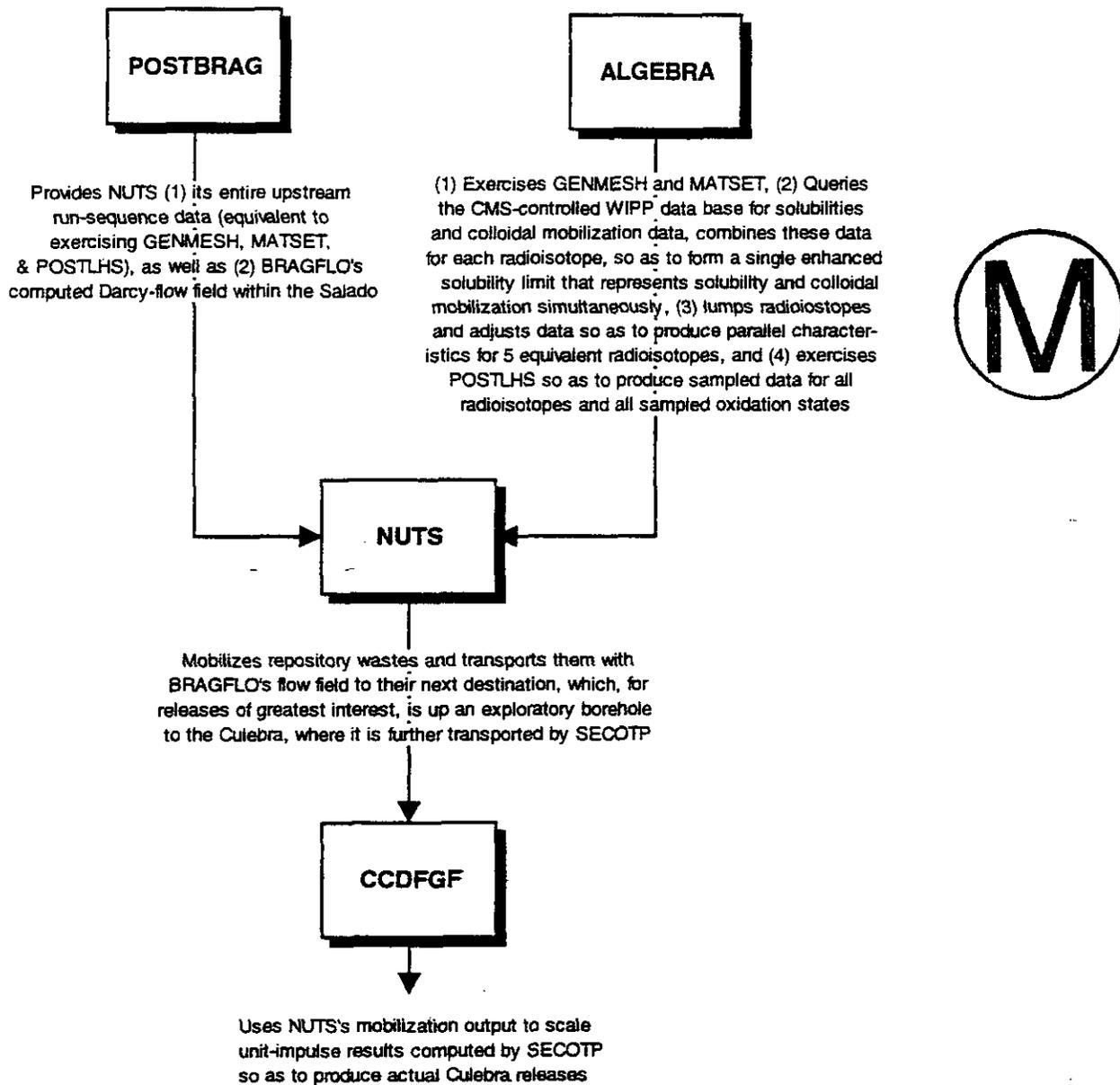
Figure 3.1: The code sequence for NUTS as it is exercised in the 1996 CCA.
