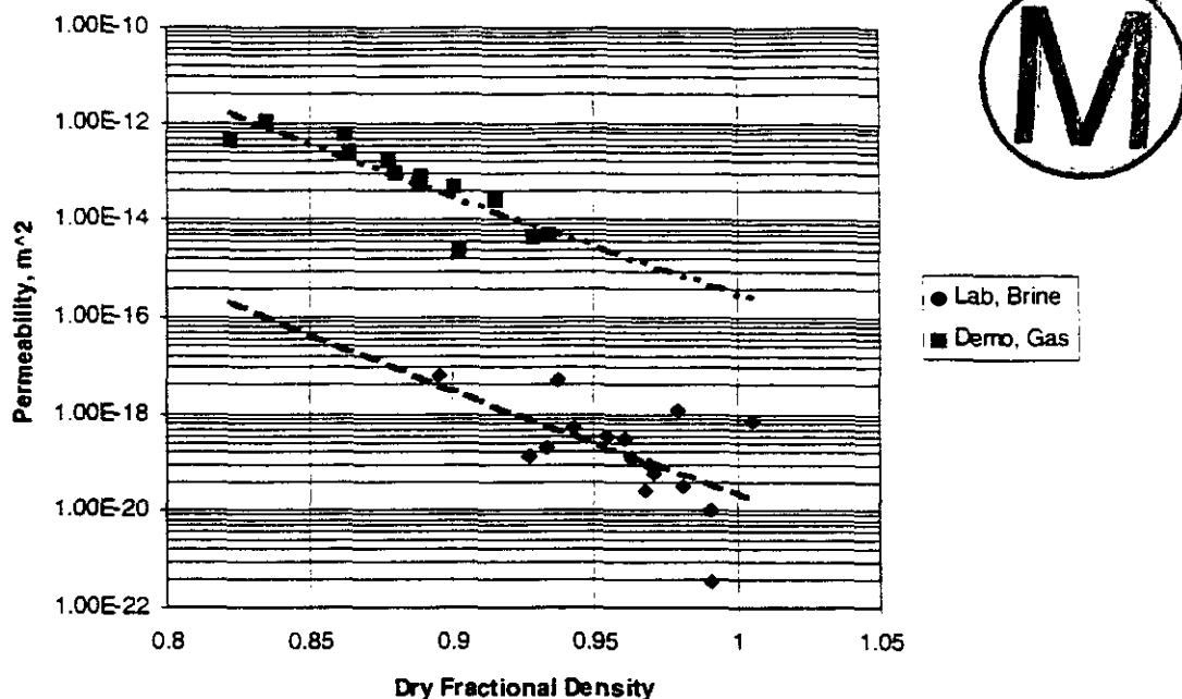
**Figure 4.4.2. Crushed Salt Permeability Data (Same Data as Figure 4.4.1), With Two Power-Law Trend Lines Representing Brine Permeabilities on Lab-Prepared Samples and Gas Permeabilities on Field Demonstration Samples**
