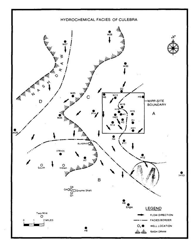
Figure 4.3.1: Summary of hydrochemical facies and local flow directions in the Culebra dolomite. Facies boundaries from Siegel et al. (1988a); modern flow directions from Figure 4.5B of LaVenue et al. (1988).
