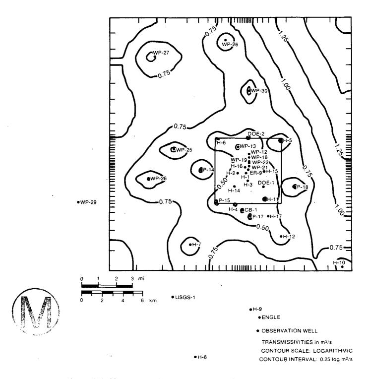
Figure 4.1.20: Estimation error in initial kriged Culebra transmissivities (one standard deviation), based on data available as of November 1987, assuming no uncertainty in individual measurements. Values kriged using code AKRIP. Figure 3.12B of LaVenue et al. (1988).
