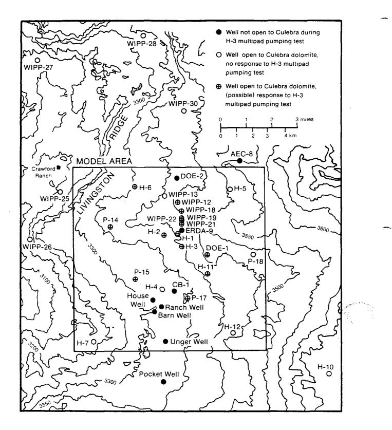
Figure 4.1.6: Pumping and observation wells for the H-3 multipad interference test. Figure 3.2 of Haug et al. (1987).
