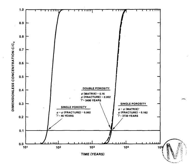
Figure 4.2.10: Comparison of base-case, regional-scale transport behavior of a conservative contaminant in the Culebra dolomite under discrete-fracture, dual-porosity, and porous-medium assumptions. Breakthrough is defined here as the time at which the concentration at the boundary of WIPP Zone 3 equals 10% of the injected concentration. Figure 5.1 of Reeves et al. (1987).
