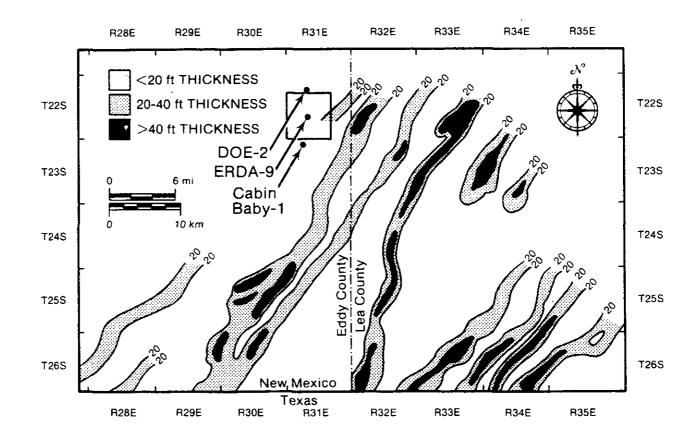
Figure 1.3: Lateral distribution and thicknesses of channel sands in the informal Ramsey member of the Bell Canyon Formation in the northern Delaware Basin, including holes DOE-2 and Cabin Baby-1. Simplified from Figure 2-2 of Davies (1983).
