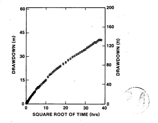
Figure 4.1.7: Observed drawdown versus the square root of time in hole H-3b2 during the H-3 multipad interference test. Slightly modified from Figure 15 of Tomasko and Jensen (1987).
