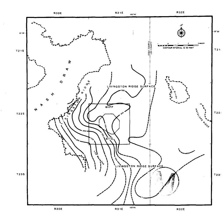
Figure 4.4.4: Distribution and thickness of the Dewey Lake Red Beds at and near the WIPP site. Figure 6 of Bachman (1985).
