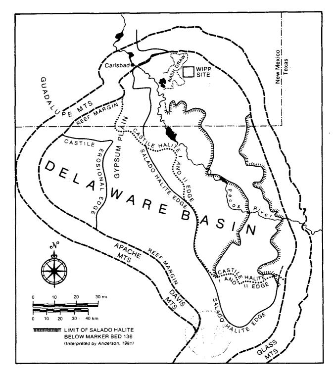
Figure 1.4: Generalized distribution of the Castile and Salado Formations in the Delaware Basin, with emphasis on distribution of halites. Slightly modified from Figure VII-1A of Lambert (1983) and including, in part, the interpretation of Anderson (1981).
