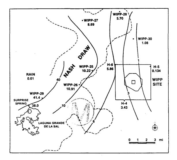
Figure 4.3.20: Total dissolved uranium content of analyzed fluids. Figure 2 of Lambert and Carter (1987).
