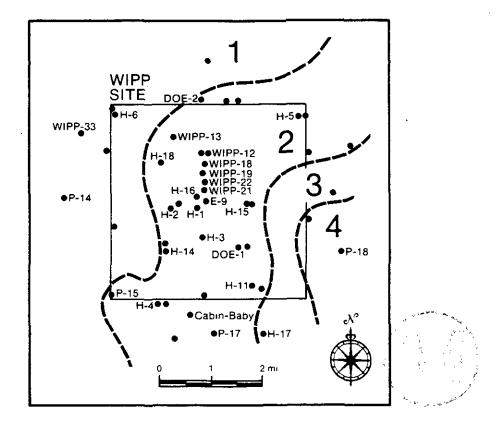
Figure 1.5: Generalized halite distribution within the Rustler Formation at and near the WIPP site. Slightly modified from Figure 9 of Chaturvedi and Channell (1985). Zone 1: no halite present within the Rustler Formation; Zone 2: halite present only below the Culebra Member; Zone 3: halite present between Culebra and Magenta Members; Zone 4: halite present above the Magenta Member.
