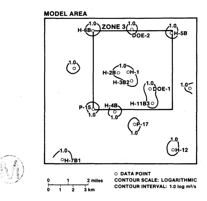
Figure 4.1.10: Estimation error in initial kriged Culebra transmissivities, based on data available as of April 1986. Slightly modified from Figure 3.8 of Haug et al. (1987).
