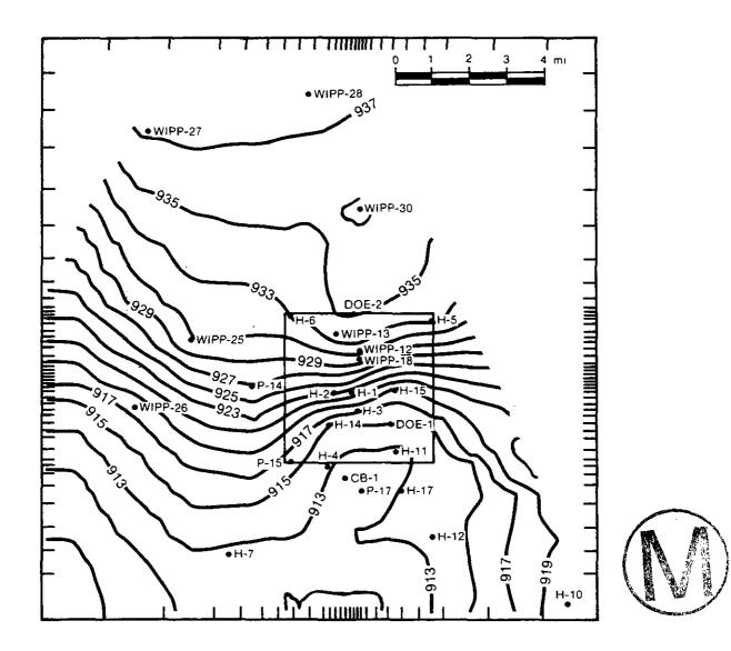
Figure 4.1.25: Calculated pre-shaft, freshwater-equivalent head distribution in the Culebra dolomite, based on calibrated transmissivity distribution shown in Figure 4.1.24. Figure 4.5A of LaVenue et al. (1988).
