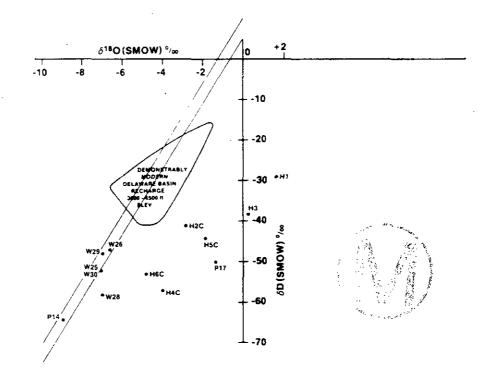
Figure 4.3.13: Stable-isotope character of waters from the Rustler/Salado contact, compared with modern precipitation in the northern Delaware Basin. The "modern recharge" field is defined as in Figure 4.3.10. Figure 15 of Lambert and Harvey (1987).
