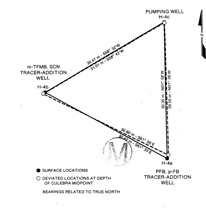
Figure 4.2.7: Physical layout of the H-4 hydropad. The figure includes orientations and spacings between holes, both at the surface and at the depth of the Culebra dolomite. Figure 6.1 of Kelley and Pickens (1986).
