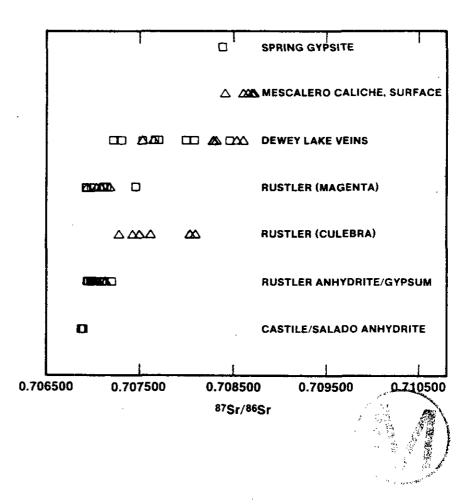
Figure 4.4.7: 87Sr/86Sr in Ochoan and related rocks at and near the WIPP site. Squares are anhydrites or gypsums; triangles are carbonates. All samples from the Dewey Lake are from veins. Samples from other units include both matrix and veins. Figure 17 of Lambert (1988).
