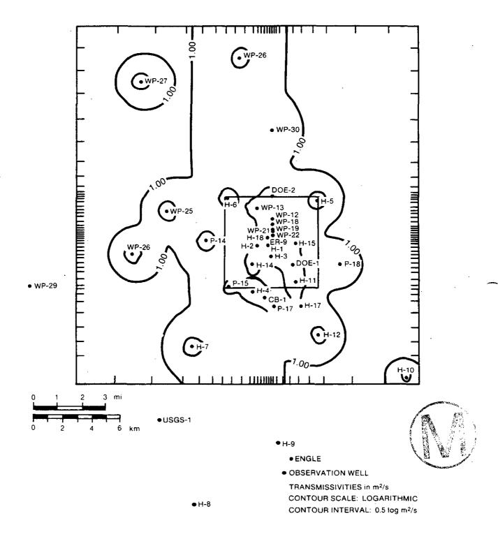
Figure 4.1.21: Estimation error in initial kriged Culebra transmissivities (one standard deviation), including estimated uncertainty in individual measurements. Values kriged using code K603. Figure 3.11B of LaVenue et al. (1988).
