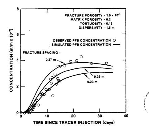
Figure 4.2.4: Best-fit simulation of measured transport behavior along the H-3b2 - H-3b3 flow path, assuming matrix tortuosity of 0.15. Fracture porosity is assumed to be the same as calculated for the flow path H-3b1 to H-3b3. Figure 4.11a of Kelley and Pickens (1986).
