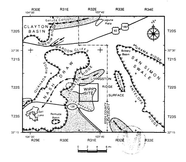
Figure 4.4.2: Probable distribution of stream channels and flow directions at and near the WIPP site during Gatuna time. Figure 11 of Bachman (1985). The present distribution of the Gatuna Formation is indicated by the stippled pattern.
