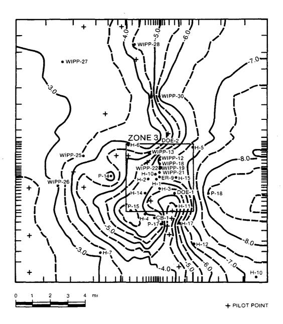
Figure 4.1.24: Calculated Culebra transmissivities at and near the WIPP site, based on steady-state calibration against freshwaterequivalent head distribution shown in Figure 4.1.23, fixing in place the fluid-density distribution shown in Figure 4.1.22. Figure 4.3 of LaVenue et al. (1988).
