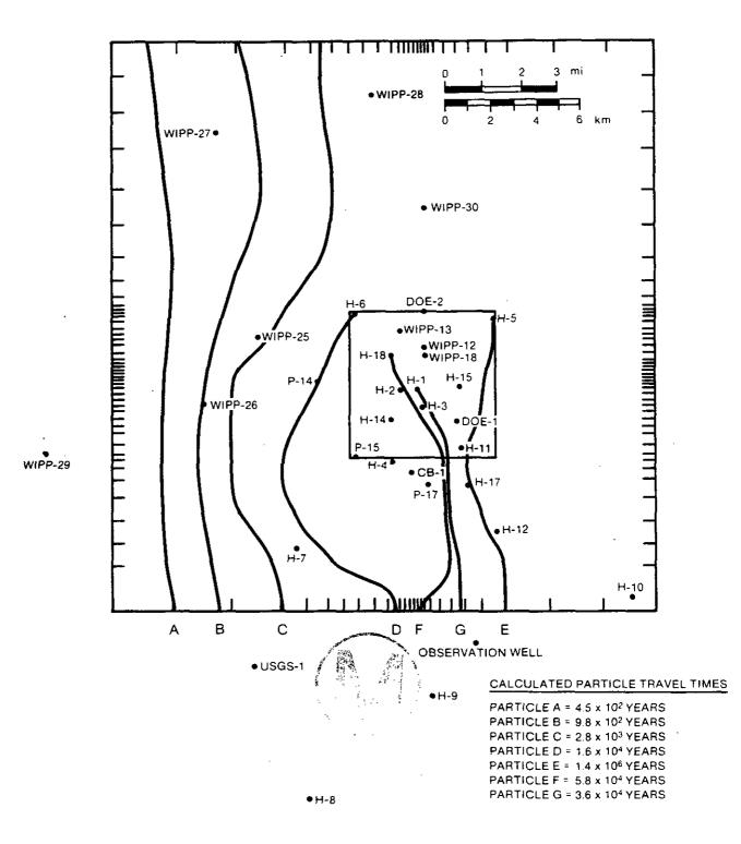
Figure 4.1.28: Calculated particle flowpaths and flow times within the Culebra dolomite, assuming steady-state and the transmissivity and head distributions shown in Figures 4.1.24 and 4.1.25. Figure 4.17 of LaVenue at al. (1988).
