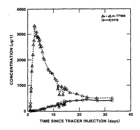
Figure 4.2.1: Observed tracer behavior during the convergent-flow test at the H-3 hydropad. Figure 4.5 of Kelley and Pickens (1986).
