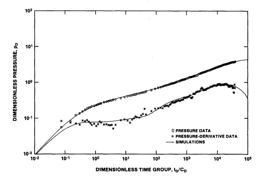
Figure 4.1.18: Measured and simulated hydrologic response of WIPP-13 during the pumping phase of the WIPP-13 multipad interference test. Slightly simplified from Figure 6-1 of Beauheim (1987c).
