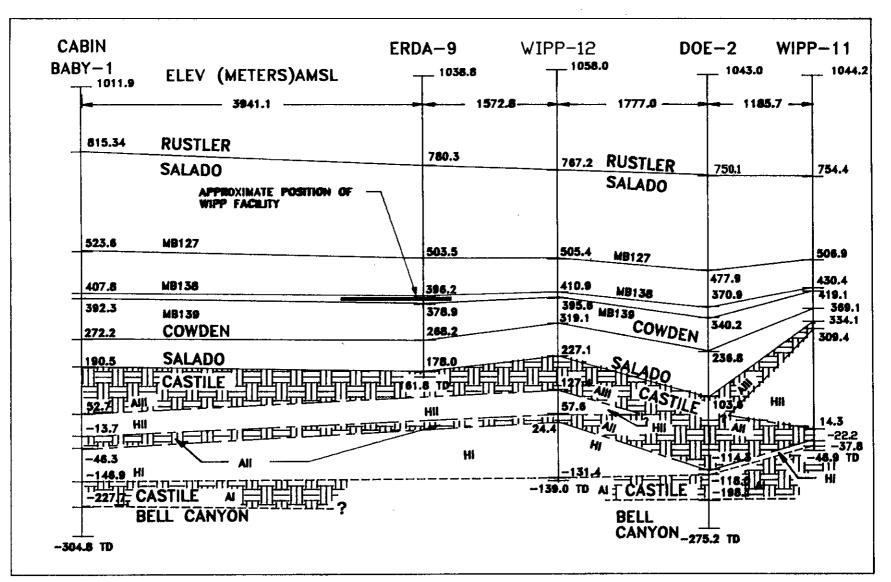
Figure 3.1: Generalized stratigraphic cross section of the Salado and Castile Formations between holes Cabin Baby-1 and WIPP-11. Hole locations used are shown in Figure 3.2. Elevations and hole spacings are in meters.
