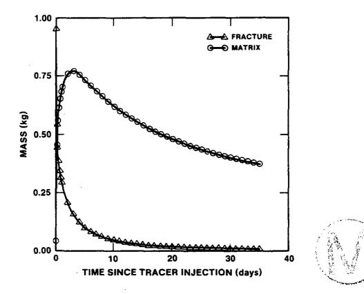
Figure 4.2.6: Calculated total masses of tracer m-TFMB in matrix and fractures as a function of time after injection. The fact that the total mass is less than 1 kg after approximately 2.5 days into the test reflects removal of tracer at the sampling hole, H-3b3. Figure 4.13 of Kelley and Pickens (1986).
