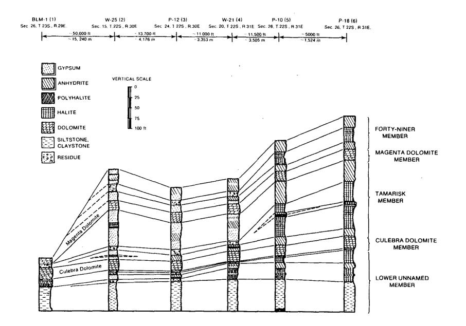
Figure 4.4.5: Columnar cross section across the WIPP site, showing lithologic correlations and variability of units in the Rustler Formation. Figure 2 of Snyder (1985).
