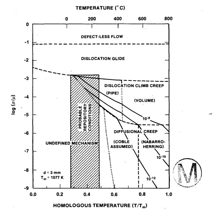
Figure 3.3: Deformation map for halite, assuming all deformation is anhydrous. Figure 2 of Borns (1987b). Homologous temperature  $(T/T_m)$  is the ratio between temperature and the dry melting temperature of halite. The stress axis is the log ratio of differential stress to halite shear modulus.
