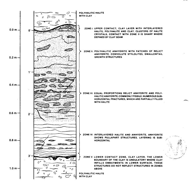
Figure 3.12: Generalized stratigraphic and structural cross section of MB139. The figure demonstrates the internal variability of the unit and the character of both upper and lower contacts. Figure 3 of Borns (1985).
