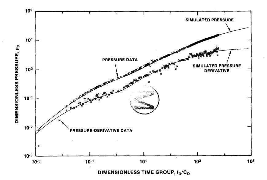
Figure 4.1.1: Measured and simulated response of H-3b1 to pumping of hole H-3b2. The presence of dual-porosity effects due to fracturing is indicated by the inflection in both measured and simulated pressure-derivative curves, in this case at a value of the dimensionless time group of approximately one. Simplified from Figure 6-11 of Beauheim (1987a).
