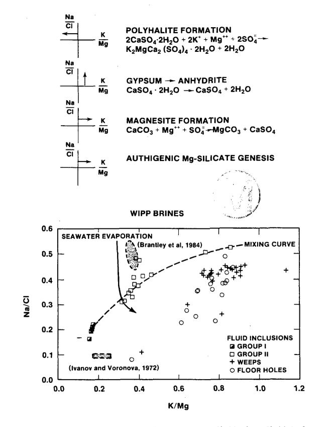
Figure 3.10: Compositional variability of Salado fluids from fluid inclusions and macroscopic brine occurrences in the WIPP facility. Figure 9 of Stein and Krumhansl (1986). Effects of individual reactions on fluid composition are also indicated.
