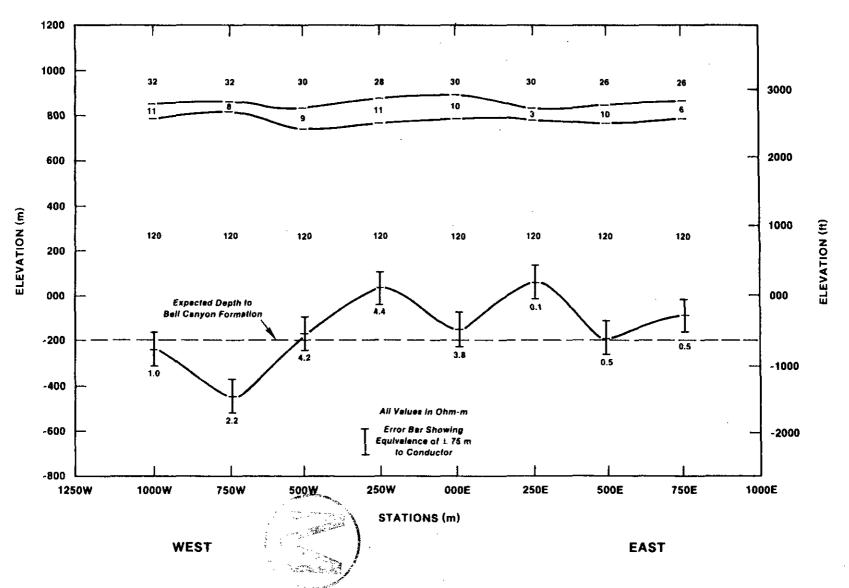
Figure 3.6: Cross section of apparent depth to first major deep conductor, showing brine locally present in both the Bell Canyon and Castile Formations. Line of section is along the north side of the WIPP waste-emplacement panels. Figure 4-11 of Earth Technology (1987).
