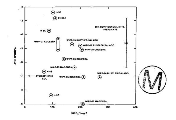
Figure 4.3.16: Relationship between 13C fractionation and bicarbonate for analyzed fluids. Figure 4 of Lambert (1987a).
