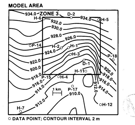
Figure 4.1.11: Best estimate of pre-shaft Culebra freshwater equivalent heads, based on data available as of April 1986. Slightly modified from Figure 3.9 of Haug et al. (1987).
