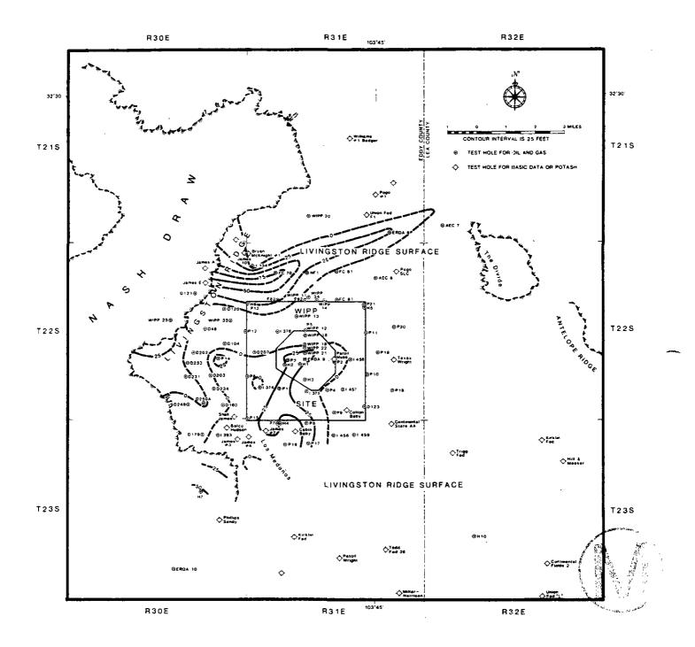
Figure 4.4.1: Distribution and thickness of the Gatuna Formation at and near the WIPP site. Figure 4 of Bachman (1985).
