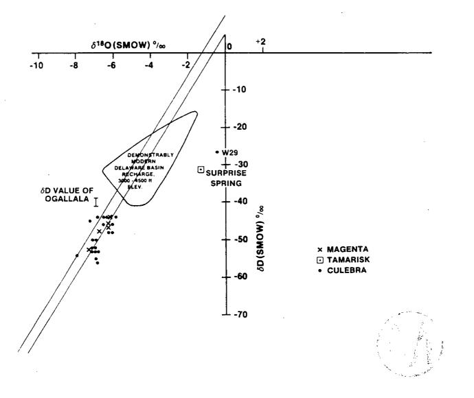
Figure 4.3.10: Stable-isotope compositions of waters from the Culebra and Magenta dolomites at and near the WIPP site. The "modern recharge" field is defined by the Carlsbad Caverns field and other consistent data contained in Figures 4.3.8 and 4.3.9. Note the anomalous character of samples from WIPP-29 and Surprise Spring. Slightly modified from Figure 14 of Lambert and Harvey (1987).
