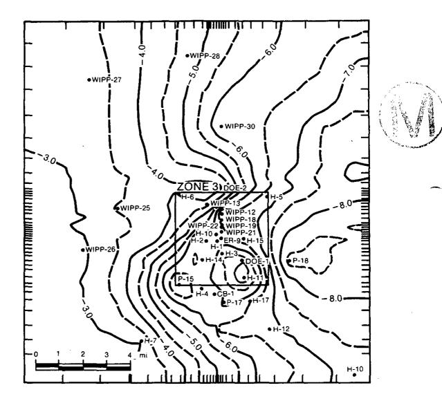
Figure 4.1.19: Initial kriged Culebra transmissivities, based on data available as of November, 1987. Values kriged with code AKRIP. Figure 3.12A of LaVenue et al. (1988).
