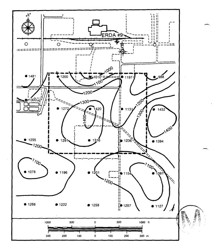
Figure 3.5: Contour map of apparent depth to first major deep conductor in survey including area of WIPP waste-emplacement panels, in meters. The heavily dashed rectangle outlines the surface projection of the WIPP waste-emplacement panels. Simplified from Figure 3-3 of Earth Technology (1987).
