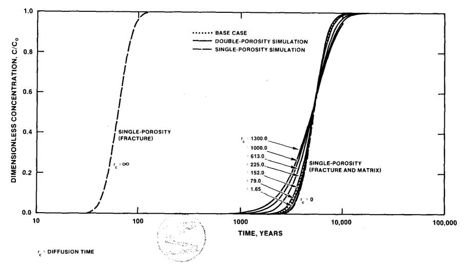
Figure 4.2.11: Estimated effect of variations in diffusion time on breakthrough, otherwise assuming base-case Culebra properties. The diffusion time is the time required for contaminant concentration at the center of matrix blocks to equal approximately 68% of the concentration in fractures. Modified from Figure 4.3 of Reeves et al. (1987).
