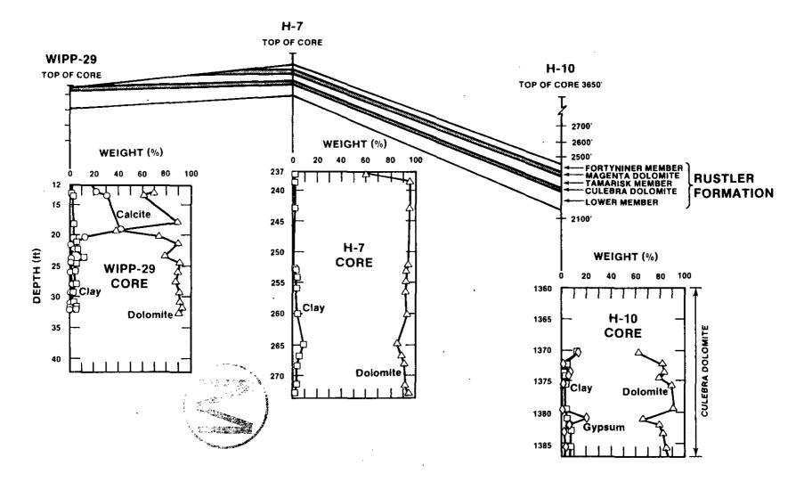
Figure 4.3.7: Fence diagram of variations in bulk mineralogy of core samples of the Culebra dolomite along the east-west section including holes WIPP-29, H-7, and H-10. From Siegel et al. (1988a).
