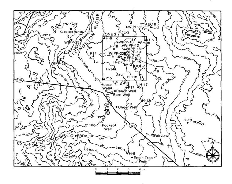
Figure 1.2: Boreholes at and near the WIPP site referred to in text. Holes were drilled as part of the site-characterization of the WIPP, as ranchers' wells, or as potash or hydrocarbon exploration holes. Only exploration holes which have been hydrologically tested are included.
