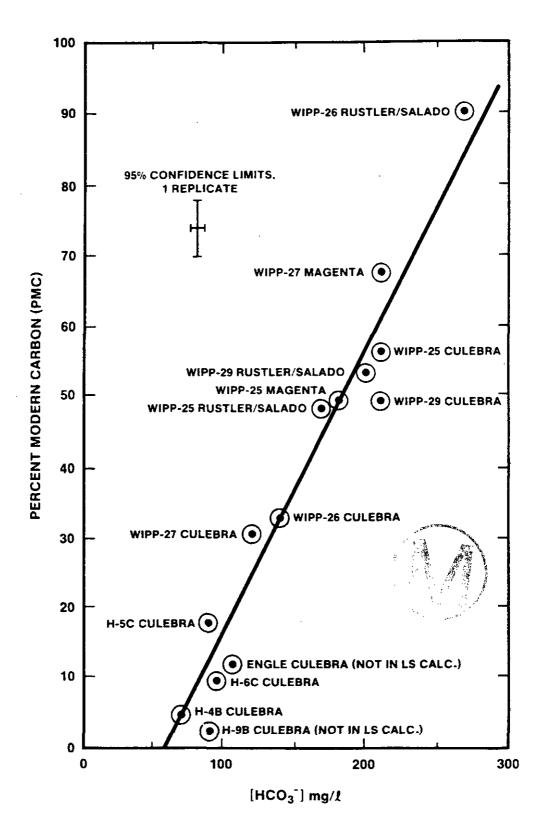
Figure 4.3.15: Relationship between calculated percent modern carbon (PMC) and bicarbonate in analyzed fluids. Figure 3 of Lambert (1987a).
