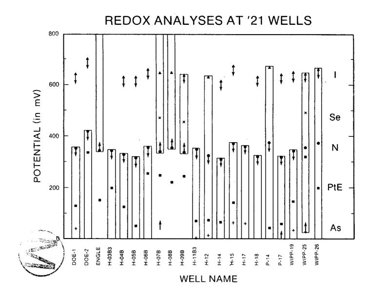
Figure 4.3.6: Variability in approximate redox potential of waters from several Culebra wells. Symbols:  $+ = AsIII/AsV; \Box = platinum electrode; o = NH3/NO3^{-}; x = SeIV/SeVI; A = I^{-}/IO3^{-}$ . Arrows indicate upper or lower limits resulting from one member of pair being present at levels below the detection limit. From Siegel et al. (1988b).
