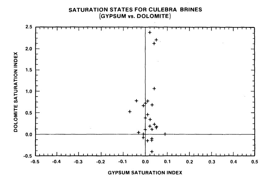
Figure 4.3.5: Variations in calculated dolomite saturation indices of Culebra waters as a function of calculated gypsum indices (Figure 4.3.4). From Siegel et al. (1988b).
