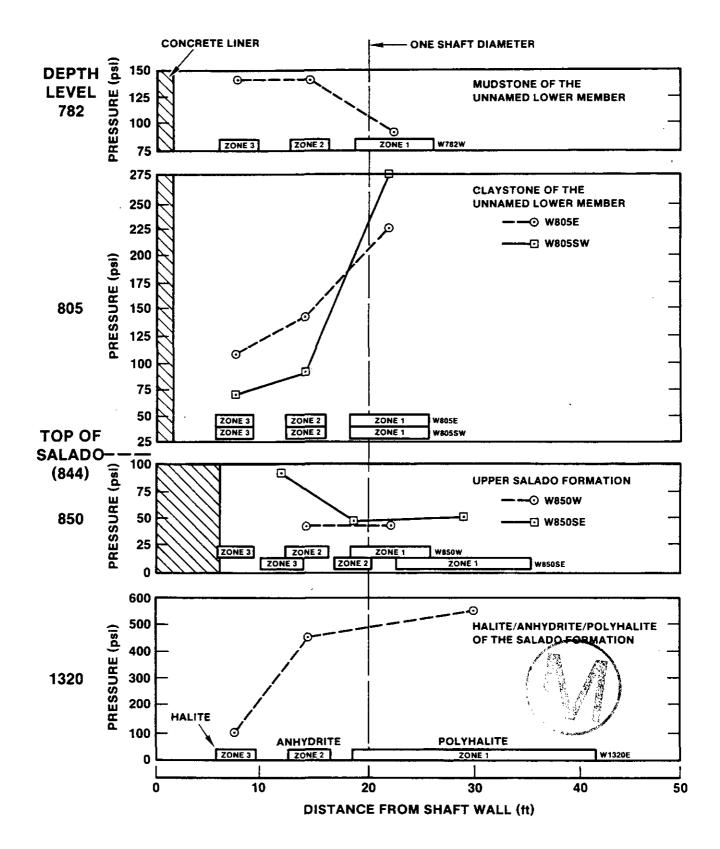
Figure 3.8: Summary of fluid formation pressures determined in 1987 testing in the WIPP waste-handling shaft. Figure 6.1 of Saulnier and Avis (1988).
