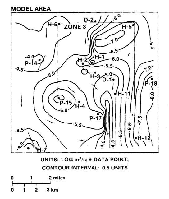
Figure 4.1.16: Final calculated Culebra transmissivities and flow directions, based on data available as of April 1986. Slightly modified from Figure 4.11 of Haug et al. (1987).
