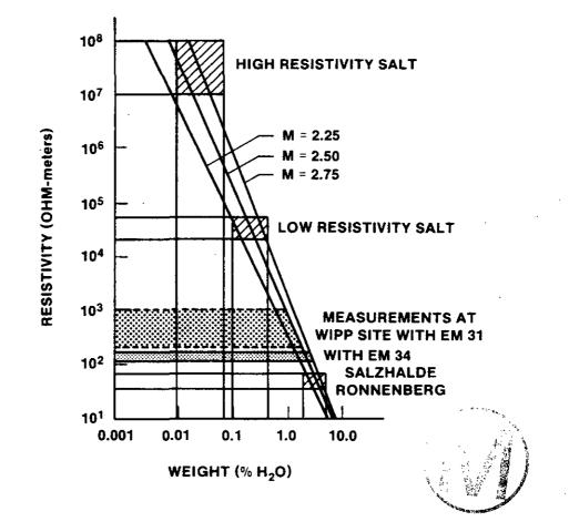
Figure 3.9: Apparent variation in water content of Salado halite at the WIPP facility horizon with depth into the wall. The EM31 survey investigates conductivity up to approximately 2 m depth and the EM34 survey to a depth up to 20 m. Figure 9 of Pfeifer (1987).
