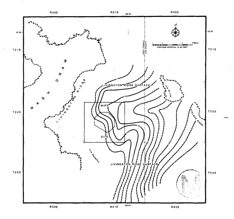
Figure 4.4.3: Distribution and thickness of Triassic rocks at and near the WIPP site. Figure 5 of Bachman (1985).
