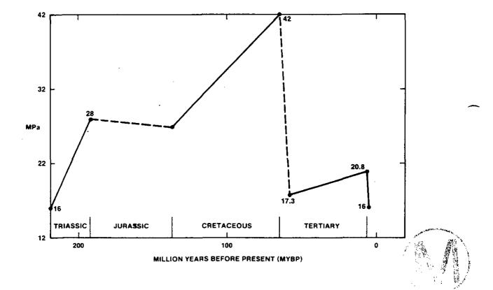
Figure 3.13: Variations in approximate overburden pressure at the WIPP facility horizon as a function of time. Overburden estimates (in MPa, 1 MPa = 145 psi) derived from Figure 10 of Borns (1985) by addition of constant 12 MPa overburden resulting from assumed constant thickness of interval between WIPP facility horizon and Rustler-Dewey Lake contact.
