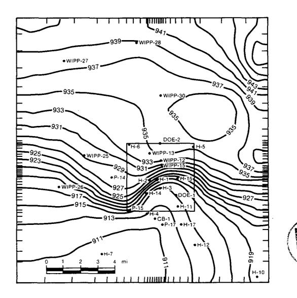
Figure 4.1.23: Estimate of pre-shaft, freshwater-equivalent heads in the Culebra dolomite, based on data available as of November 1987. Figure 3.14 of LaVenue et al. (1988).
