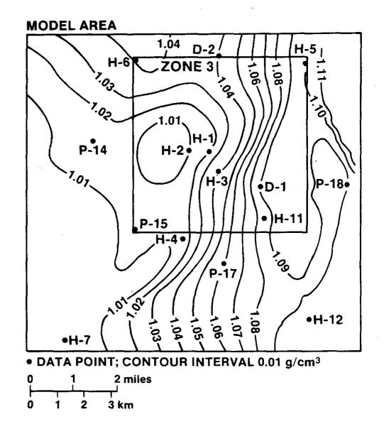
Figure 4.1.13: Best estimate of density distribution of Culebra fluids, based on information available as of April 1986. Figure 3.10 of Haug et al. (1987).
