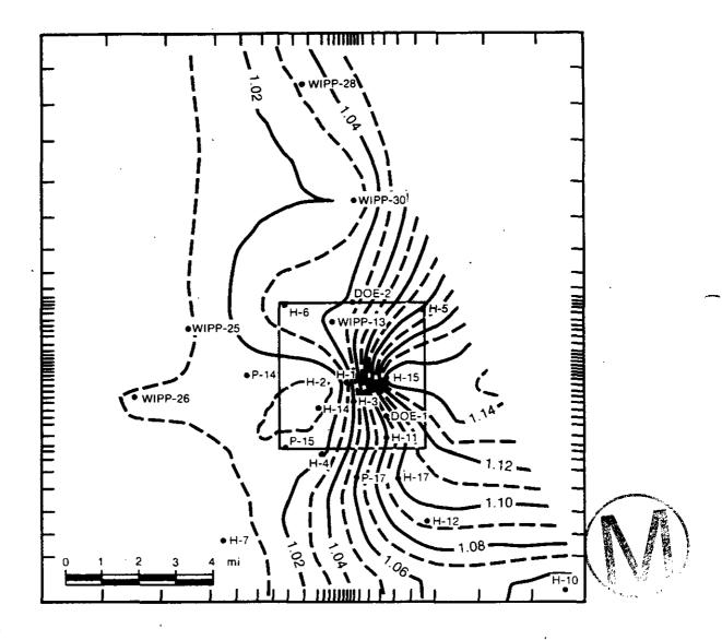
Figure 4.1.22: Measured density distribution of Culebra fluids, based on information available as of November 1987. Figure 3.15 of LaVenue et al. (1988).
