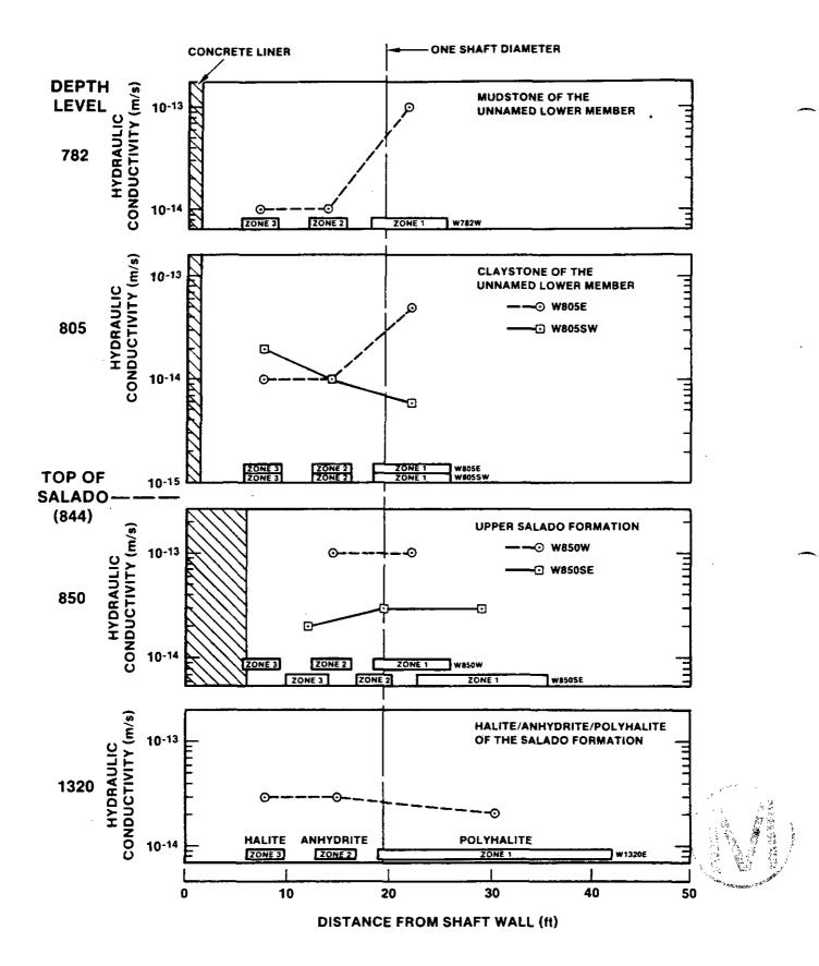
Figure 3.7: Summary of formation conductivities determined in 1987 testing in the WIPP waste-handling shaft. Figure 6.3 of Saulnier and Avis (1988).
