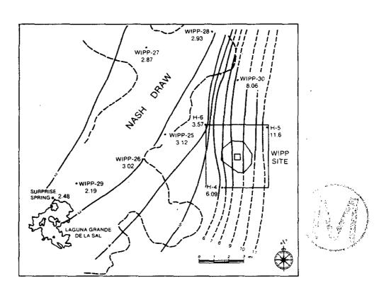
Figure 4.3.19: Contours of 234U/238U activity ratios in analyzed fluids, relaxing constraint of linear variation between data points. Modified from Figure 3 of Lambert and Carter (1987).
