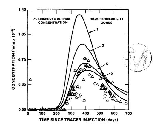
Figure 4.2.8: Best-fit simulation of m-TFMB behavior during testing at the H-4 hydropad, assuming effective injection and stability of 1 kg of tracer and control of behavior by the specified numbers of multiple high-permeability zones. Figure 6.11 of Kelley and Pickens (1986).
