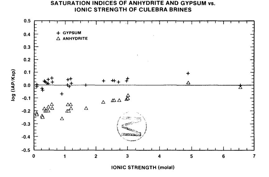
Figure 4.3.4: Variation in calculated gypsum and anhydrite saturation indices of Culebra waters as a function of ionic strength. From Siegel et al. (1988b).
