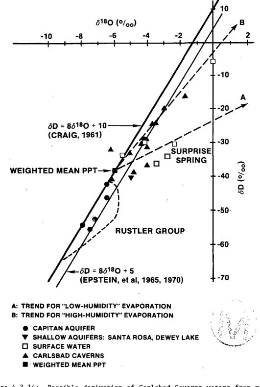
Figure 4.3.14: Possible derivation of Carlsbad Caverns waters from modern precipitation. Modified from Figures 13 and 14 of Chapman (1986), by addition of the statistical correlation line for meteoric precipitation of Epstein et al. (1965, 1970) and deletion of waters from the Roswell Basin. operation of this effect on Rustler, Dewey Lake, and confined Capitan waters, as well as Ogallala water from the High Plains is not explained.
