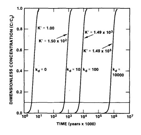
Figure 4.2.12: Variations in calculated breakthrough times to the boundary of WIPP zone 3 as a function of assumed matrix retardation, otherwise assuming base-case material properties. Matrix retardation (K') is proportional to  $1 + k'_d$ . Therefore, for a matrix distribution coefficient ( $k'_d$ ) of 0, K'=1.0. Slightly modified from Figure 4.1 of Reeves et al. (1987).
