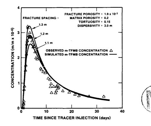
Figure 4.2.2: Best-fit simulation of measured transport behavior along the H-3bl - H-3b3 flow path, assuming matrix tortuosity of 0.15. It is assumed that 1 kg of m-TFMB was successfully injected, and remained stable throughout the test. Figure 4.10a of Kelley and Pickens (1986).
