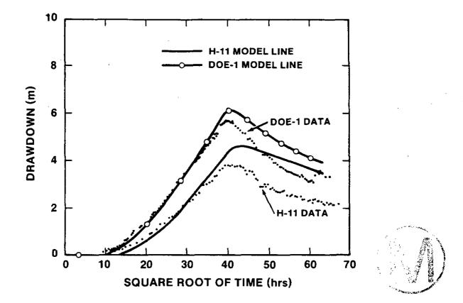
Figure 4.1.8: Comparison of measured and simulated responses at H-11 and DOE-1 during the H-3 multipad interference test, assuming perfectly linear flow. Figure 25 of Tomasko and Jensen (1987).
