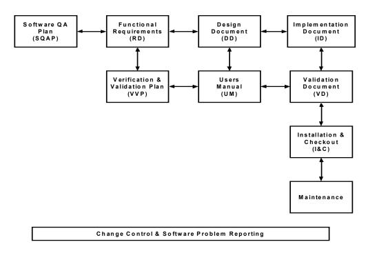
Figure 1. Major Components of DOE's Software Development Process
