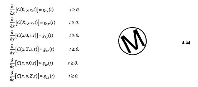
These conditions are sometimes specified internally in the domain and called point source/sink.
