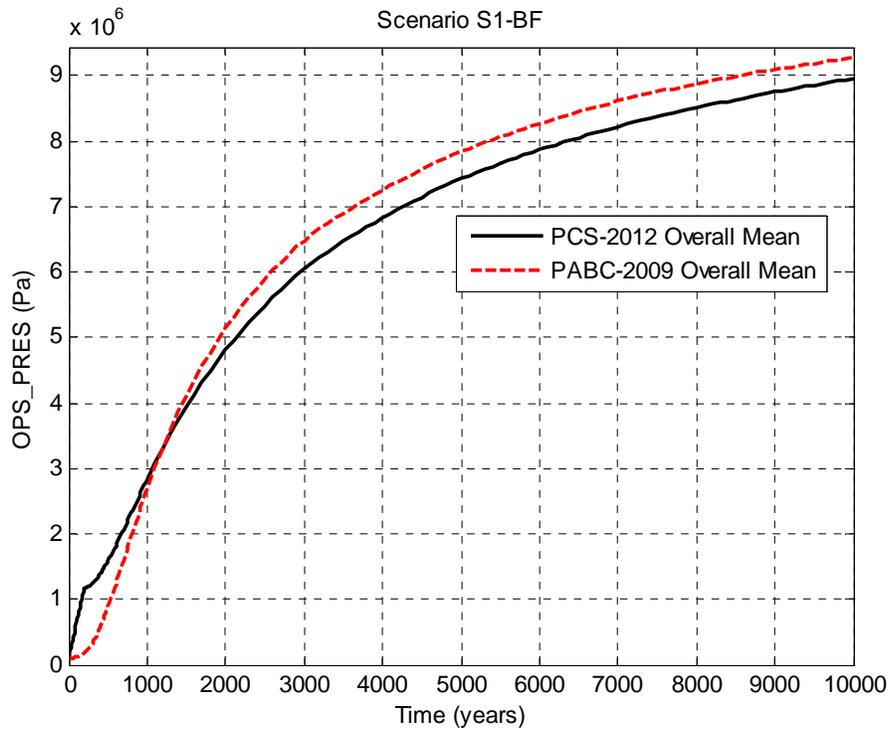
Figure 5-8: Overall Means of Pressure in the Operations Region, Scenario S1-BF.
