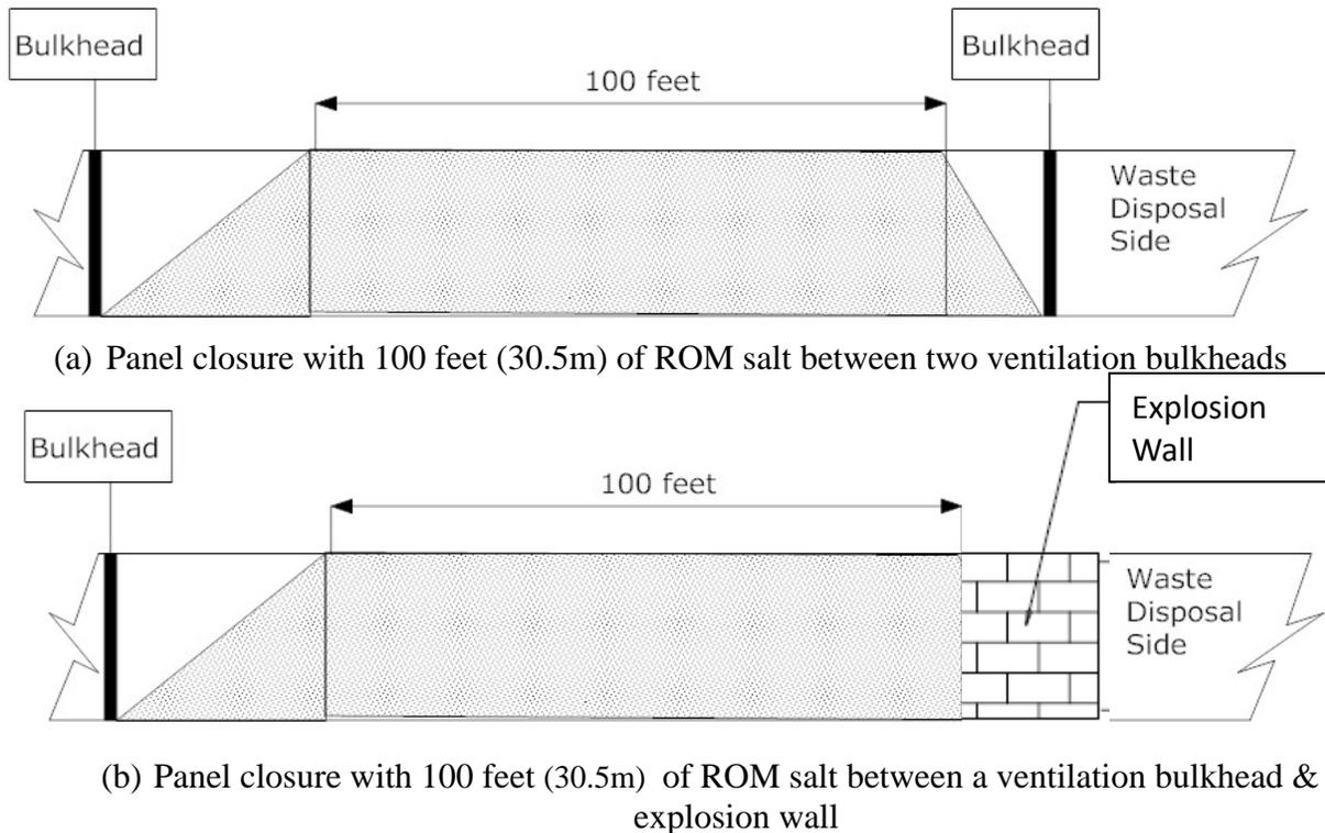
Figure 2-2: Schematic of the ROMPCS
