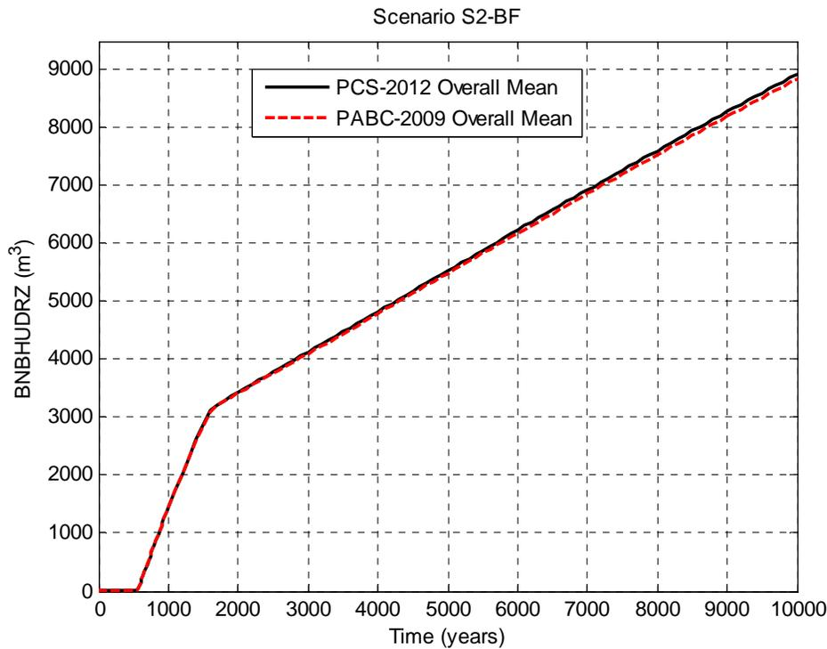
Figure 5-14: Overall Means of Brine Flow up the Borehole, Scenario S2-BF.
