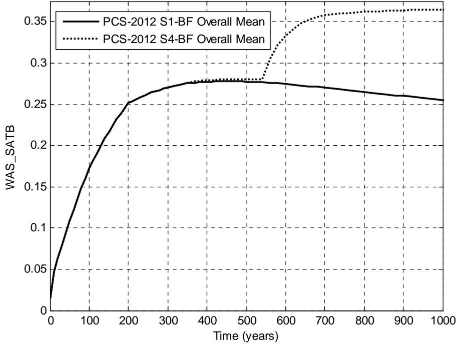
Figure 5-19: Overall Means of Waste Panel Brine Saturation, Scenarios S1-BF and S4-BF for Years 0 to 1,000.
