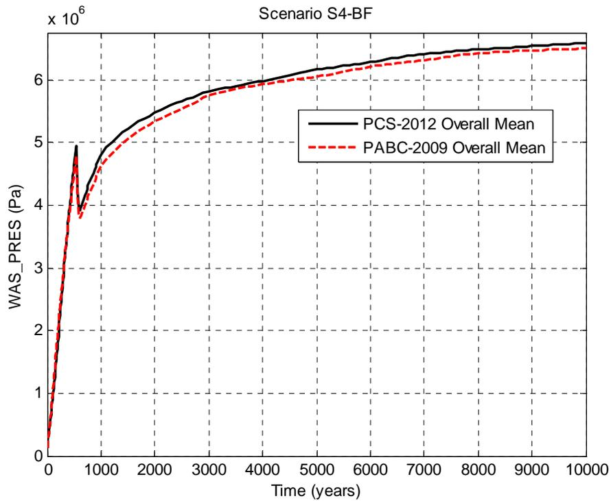
Figure 5-16: Overall Means of Waste Panel Pressure, Scenario S4-BF.
