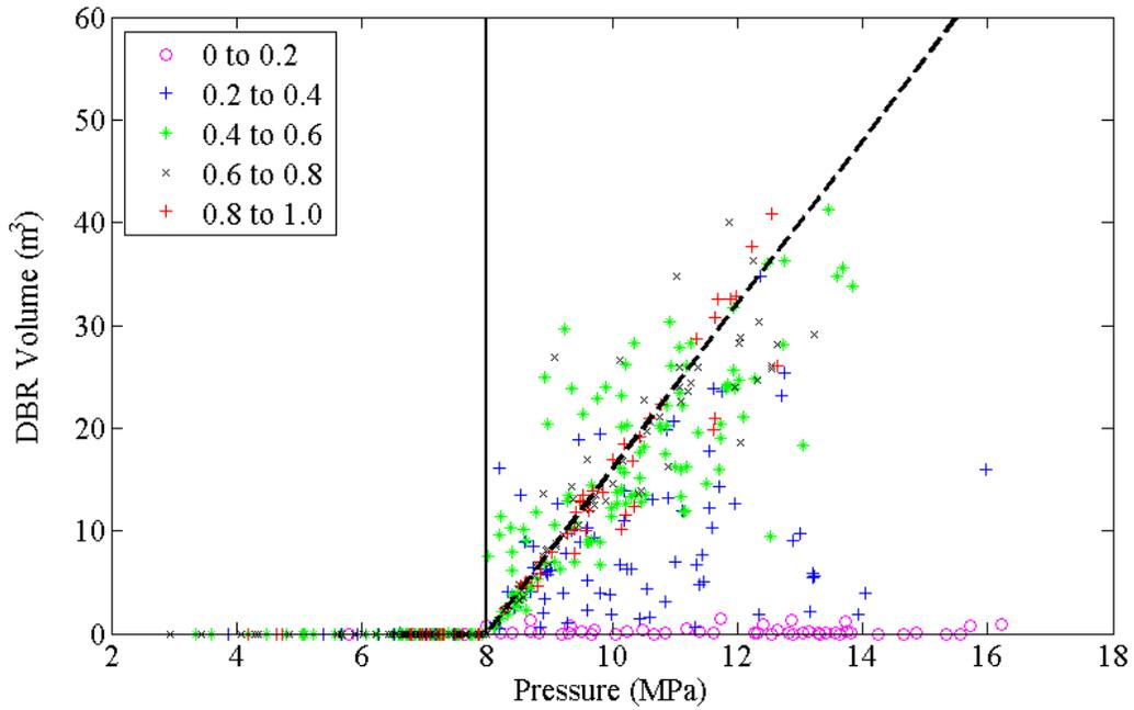
Figure 5-27: DBR Volume vs. Pressure, Scenario S2-DBR, Replicate 1, Lower Intrusion, PCS-2012 PA
