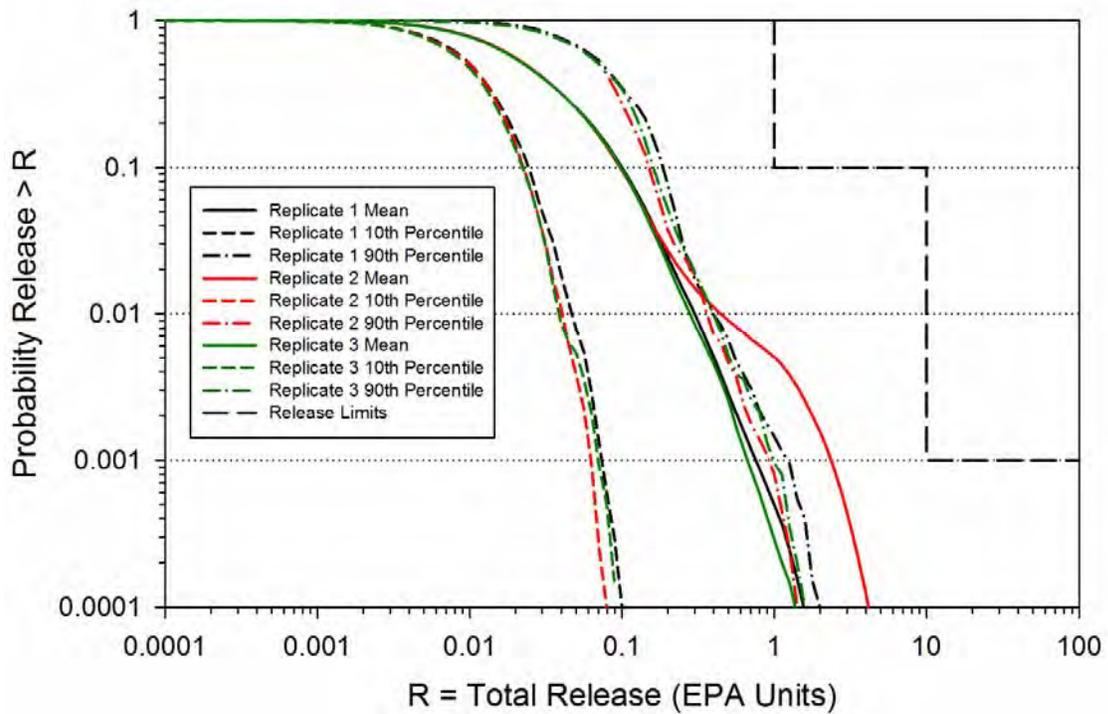
Figure 5-32: PCS-2012 PA Mean and Quantile CCDFs for Total Normalized Releases, Replicates 1-3
