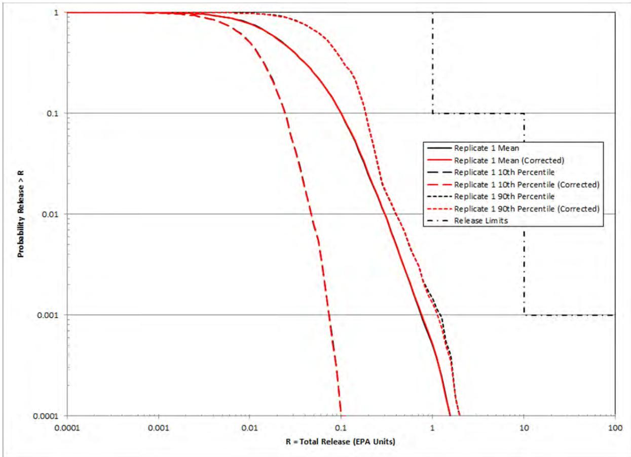
Figure B-1: Comparison of PCS-2012 PA Mean and Quantile CCDFs for Total Normalized Releases, Replicate 1
