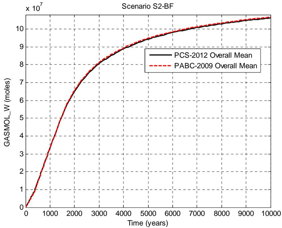
Figure 5-13: Overall Means of Waste Panel Gas Generation (in moles), Scenario S2-BF.
