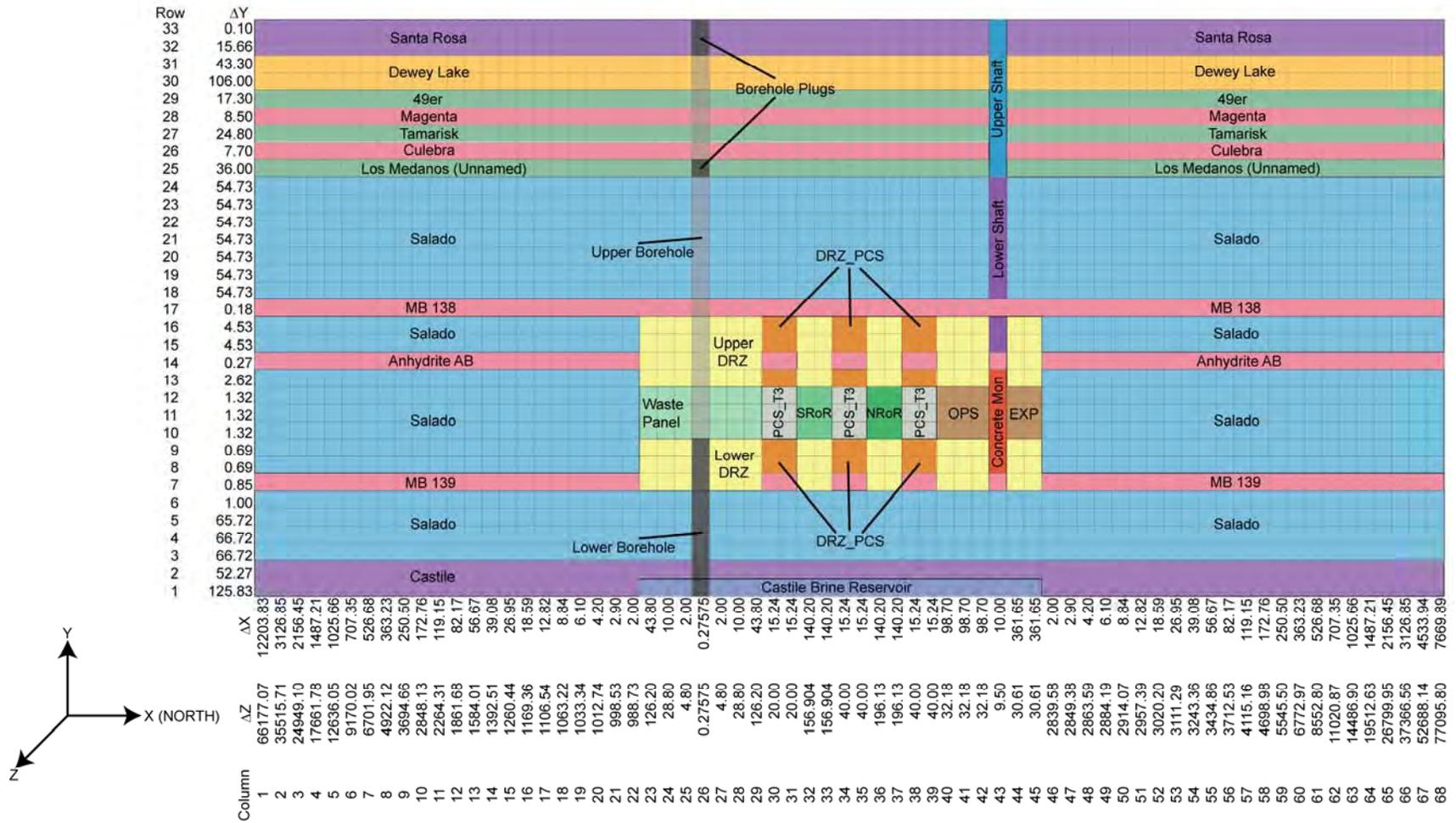
Figure 5-2: PCS-2012 BRAGFLO Grid and Material Map for an E1 Intrusion ( $\Delta x$ ,  $\Delta y$ , and  $\Delta z$  dimensions in meters).
