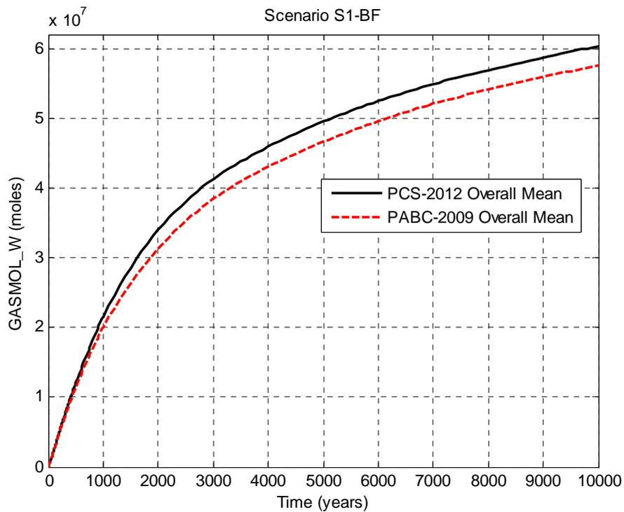
Figure 5-6: Overall Means of Waste Panel Gas Generation (in moles), Scenario S1-BF.
