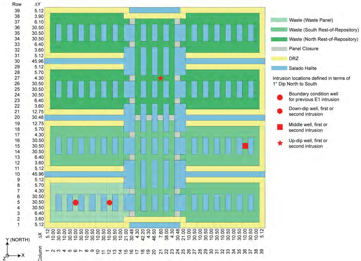
Figure 5-25: PCS-2012 PA DBR Computational Grid and Material Map (logical grid).
