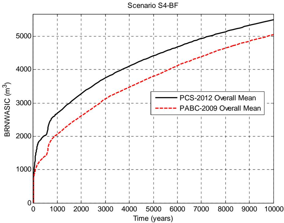
Figure 5-18: Overall Means of Cumulative Brine Inflow to the Waste Panel, Scenario S4-BF.
