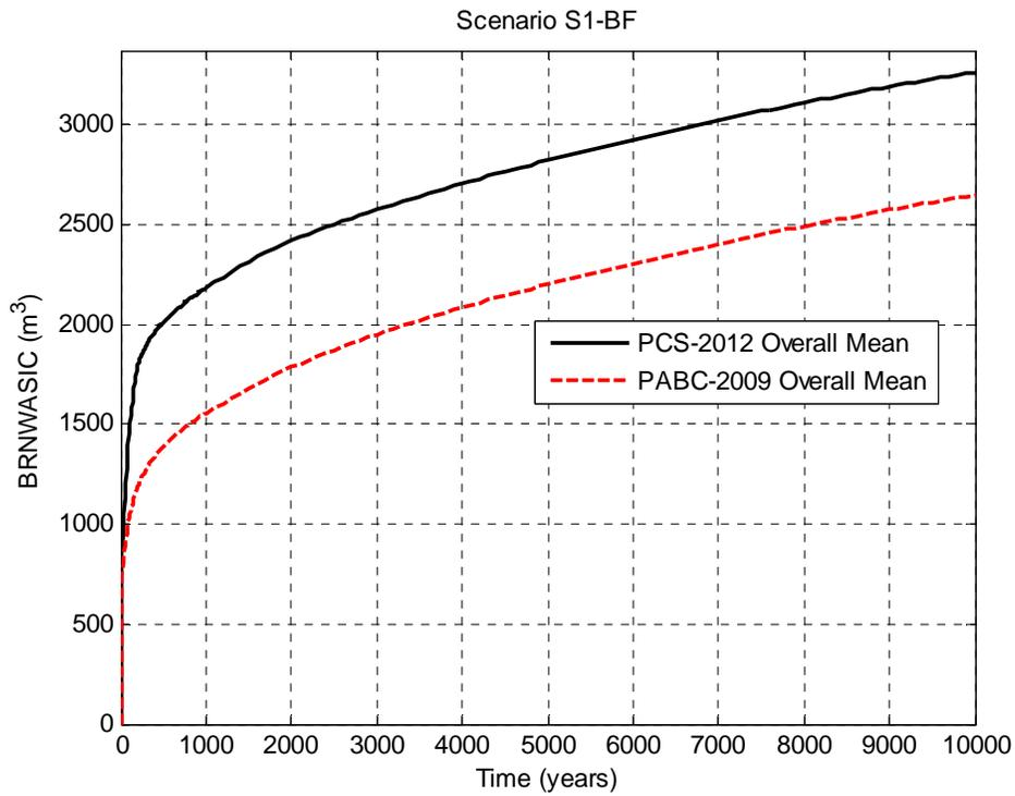
Figure 5-3: Overall Means of Cumulative Brine Inflow to the Waste Panel, Scenario S1-BF.
