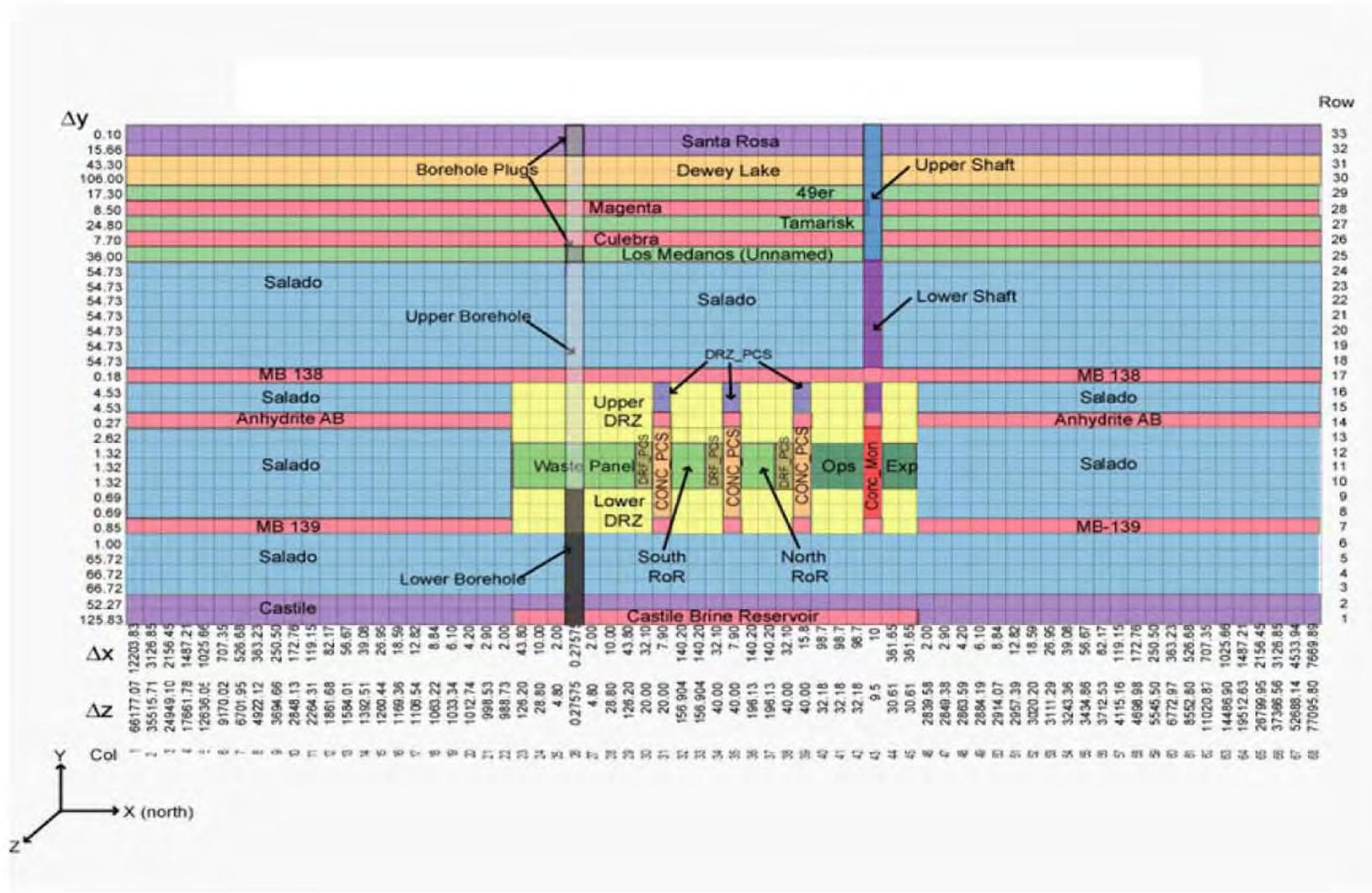
Figure 5-1: PABC-2009 BRAGFLO Grid and Material Map for an E1 Intrusion ( $\Delta x$ ,  $\Delta y$ , and  $\Delta z$  dimensions in meters).
