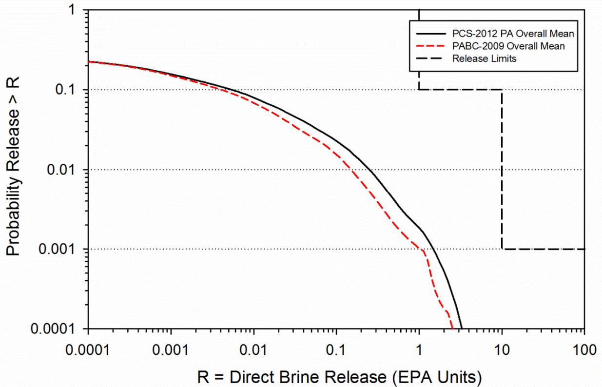
Figure 5-28: PCS-2012 PA and PABC-2009 Overall Mean CCDFs for Normalized Direct Brine Releases
