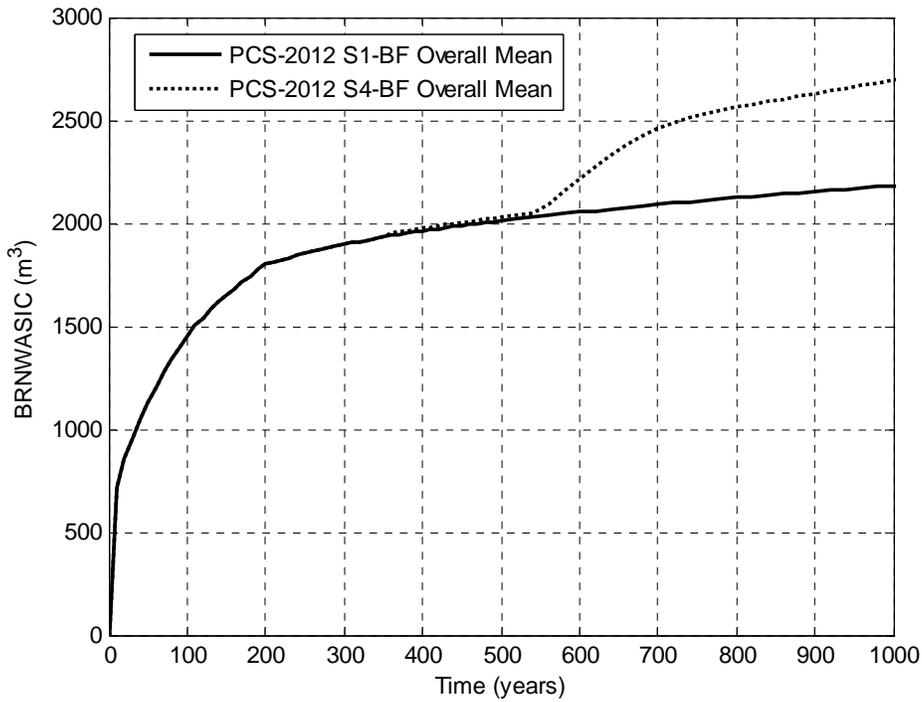
Figure 5-17: Overall Means of Cumulative Brine Inflow to the Waste Panel, Scenarios S1-BF and S4-BF for Years 0 to 1,000.
