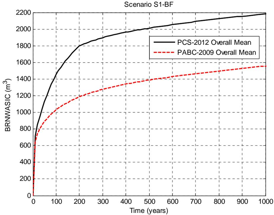
Figure 5-4: Overall Means of Cumulative Brine Inflow to the Waste Panel, Scenario S1-BF and Years 0 to 1,000.
