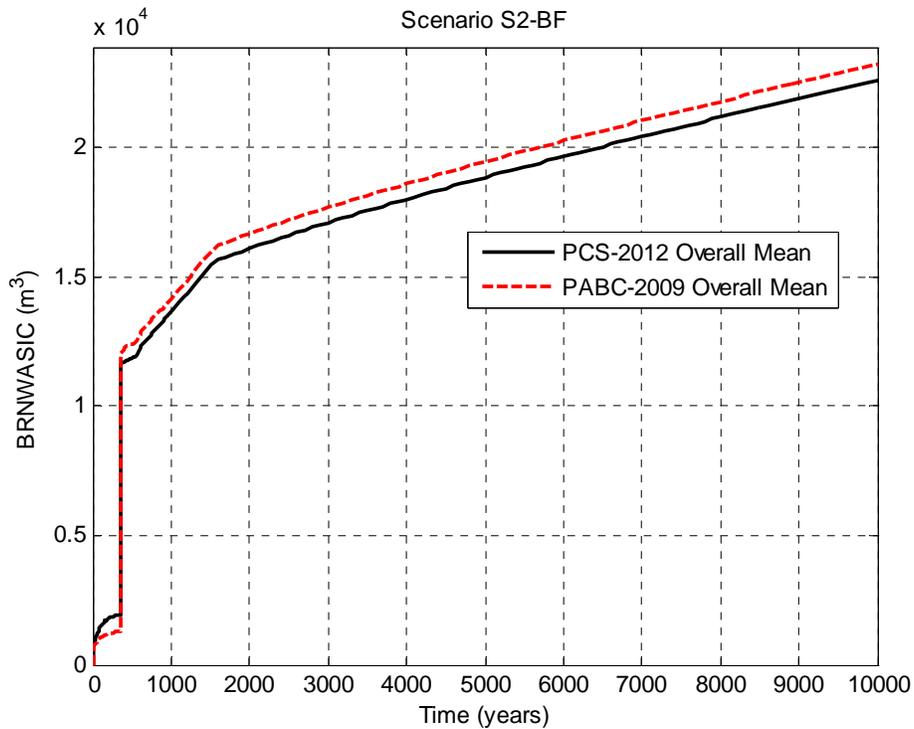
Figure 5-11: Overall Means of Cumulative Brine Inflow to the Waste Panel, Scenario S2-BF.
