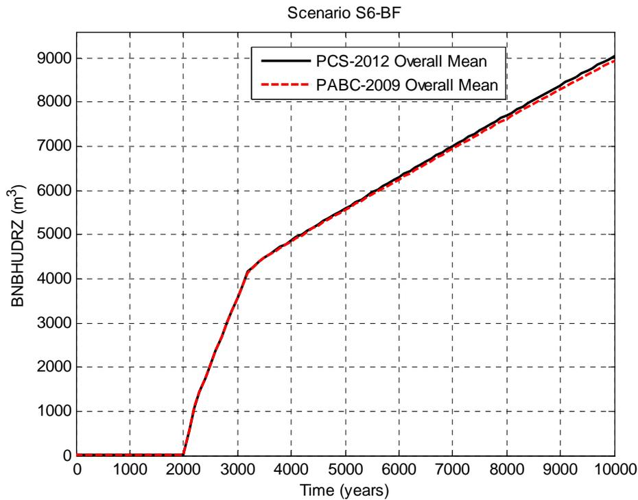
Figure 5-23: Overall Means of Brine Flow up the Borehole, Scenario S6-BF.
