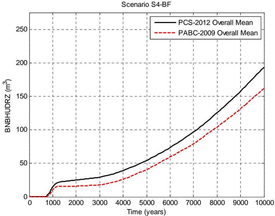
Figure 5-22: Overall Means of Brine Flow up the Borehole, Scenario S4-BF.
