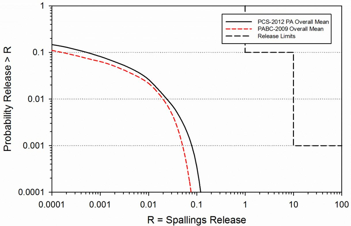
Figure 5-24: PCS-2012 PA and PABC-2009 Overall Mean CCDFs for Normalized Spallings Releases
