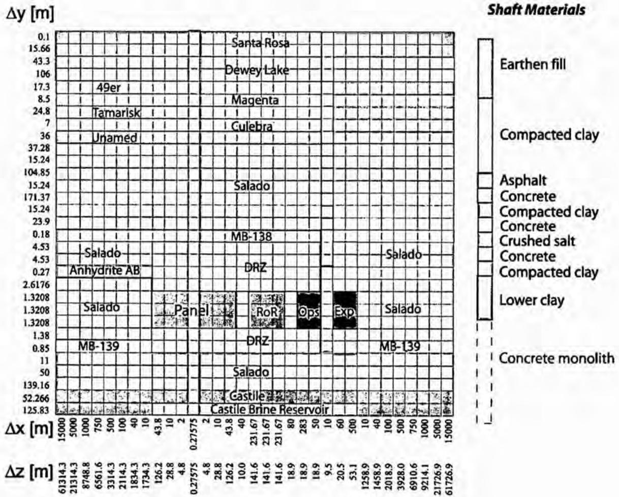
Figure 1: Baseline BRAGFLO logical grid showing the location of the shaft. The shaft is enlarged to the right and the materials used in the baseline model are labeled.
